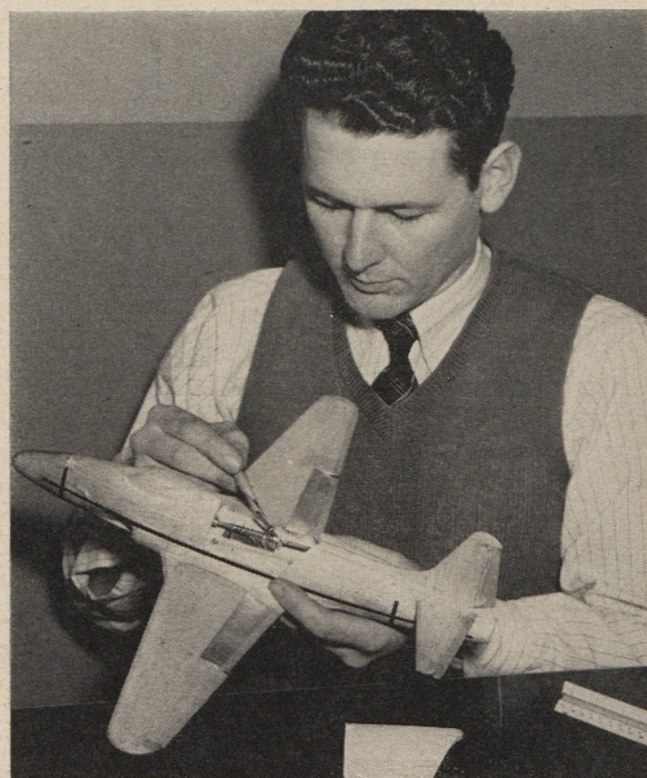
Frank R. Deis inspects controlling mechanism inside scale model F-80 which is actuated by magnetic field from copper bands which run around wall inside the test chamber.
