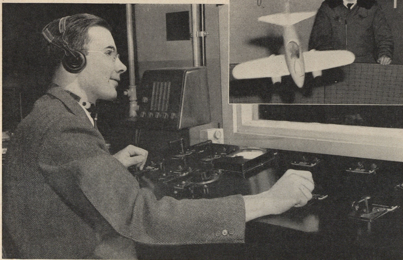
Paul Doty operates the control panel outside the inner test chamber. From here he regulates the constant-speed motor, fan velocity, power for pitch control of fan, and lights. Inset, an observer watches as Doty puts model of new jet into dive.
