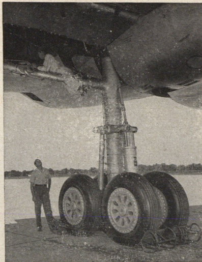
Another major alteration in production-type B-36 is in the landing gear. The 110-inch single tire (left) is supplanted by a 4-wheel truck carrying standard 56-inch wheels. This not only saves 2600 lbs in weight but is operationally safer in case of blowouts.
