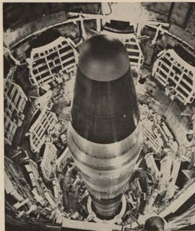
Ready for launch is this ten-story-tall Titan II intercontinental-range missile on 150-foot-deep underground launch pad. Titan II is silo-launched in less than a minute, has thrust, range, and payload greater than any other US ICBM. Employed by SAC and AFSC, Titan II was also launch vehicle for Gemini.
