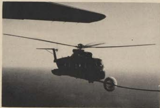
This Sikorsky HH-3E Jolly Green Giant rescue helicopter moves in to refuel from Lockheed HC-130P over the South China Sea. In-flight refueling enables HH-3Es to remain on alert for longer periods, and to respond sooner whenever an airman is downed.
