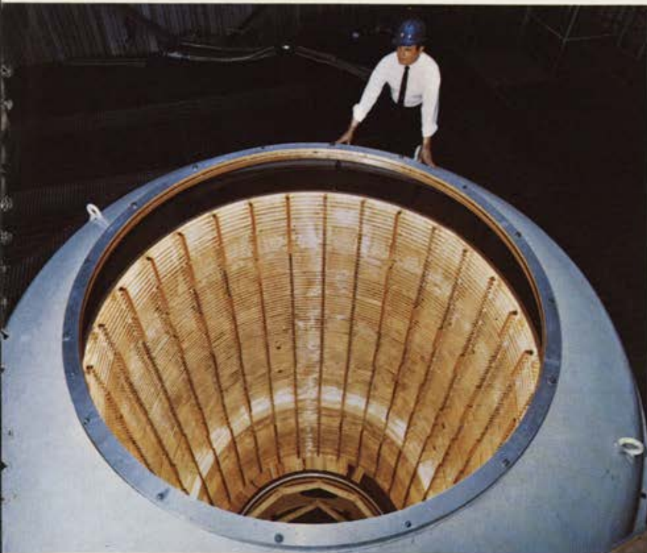
This radiant heating reflector assembly stands vertically inside a 20-foot high vacuum bell—part of the Beech Transient Heat Facility used for thermal studies of rocket and missile propellant tank systems and components.
