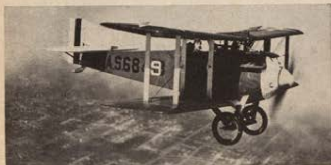
In its day, 1919, the Thomas-Morse MB-3A could hit a top speed of 152 mph. Powered by a 340-horsepower Hispano-Suiza engine, the stubby MB-3A measured 26 feet in wingspan, only 20 feet from propeller to rudder. The Army liked it well enough to buy 54 copies from the now-defunct Ithaca, N. Y., firm.
