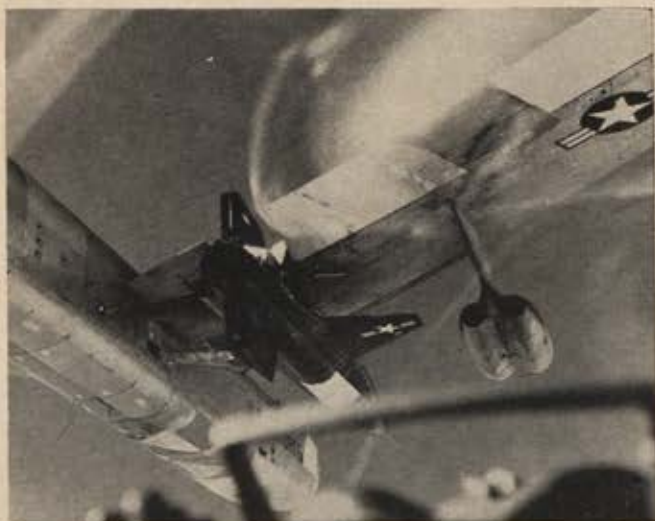
Somewhat lost in the cloud of publicity that attended the missile/space boom of the 1950s and early 1960s were the achievements of the Air Force's X-15 rocket-airplane research program. Carried along under the wing of a specially modified B-52, the X-15 soared, rocket-powered, to enormous altitudes, producing vast amounts of data on human and machine parameters of controlled, manned flight—data fed into many on-going programs.
