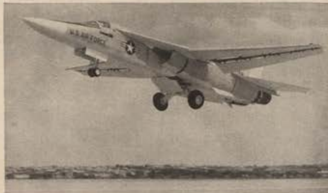
Both TAC and SAC will use versatile F-111, first aircraft to employ both variable-sweep wings and turbofan afterburning engines. It is designed to fly from under 100 knots to Mach 2.5 at altitude, with supersonic low-level dash, and holds unofficial range record for tactical fighter using only internal fuel.
