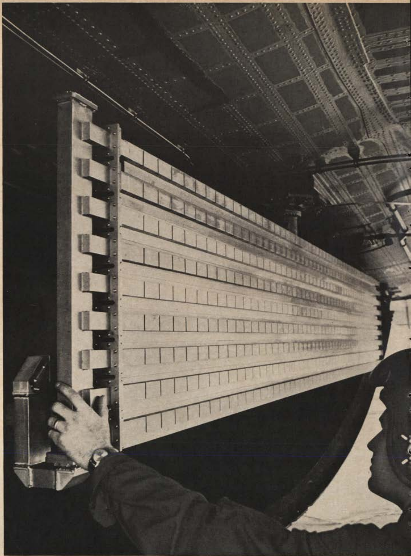
Installed in the radome of an Air Force RC-121, new Westinghouse experimental overland radar antenna is made ready for actual flight tests.
