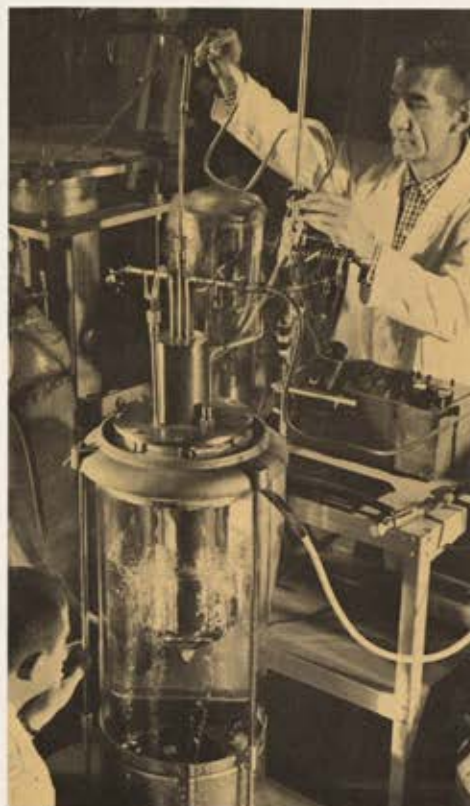
By sub-cooling liquid hydrogen to an icy slush, Beech engineers here are testing the feasibility of further reducing hydrogen volume to boost fuel loads without increasing tank size and weight.
