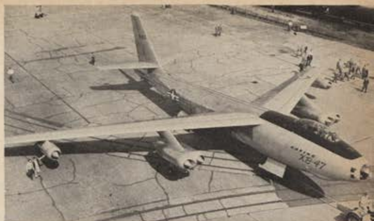
The Boeing B-47, shown in its experimental XB-47 configuration, was one of the B-36's successors in the SAC air fleet. With its ultrathin wings supporting 6 jet engines in double nacelles in-board and singly near the sweptback wingtips, its design was striking for the time. It, too, like the B-36, was never used in war.
