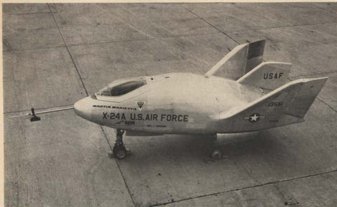
A promising prospect for future Air Force earth-to-orbit shuttling and back is the lifting body, the wingless craft that derives its lift from its own shape. This is Martin Marietta's X-24A manned supersonic lifting body research vehicle, being used in a USAF-NASA exploration of the capabilities of such unorthodox craft. It was turned over to the Air Force in July after extensive engineering tests.
