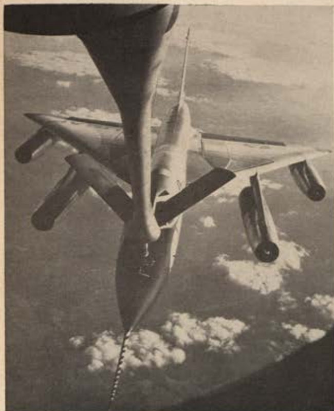
Fastest bomber yet developed for Strategic Air Command is the B-58 Hustler, here refueled by a KC-135 tanker. One-third of the size of a B-52, the B-58 can exceed Mach 2 at 35,000 feet. It carries nuclear weapons but is not readily adaptable to a conventional-weapon payload so has not been used in Vietnam. Despite capabilities, the B-58 is scheduled for phase out by 1970.
