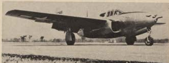
First US-built jet was the Bell P-59, powered by two 2,000-pound-thrust General Electric J31 engines. It was first flown in October 1942, piloted by Col. (later Lt. Gen.) Laurence C. Craigie. Sixty were built, but none was employed in combat.
