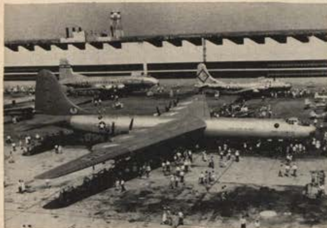
Above all, the B-36 was big, its very bigness attracting crowds wherever it was shown. Its bomb bay held as much as three freight cars, its deicing system could have heated a 600-room hotel. Crewmen moved between fore and aft sections via a tunnel.
