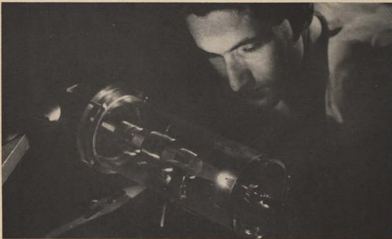
Ionized gases may cause surface pitting on the skins of spacecraft flying within earth's or some other planet's atmosphere. Ion accelerator pictured is used by NACA to study ion impact effects at speeds of 15,000 mph or even faster.
