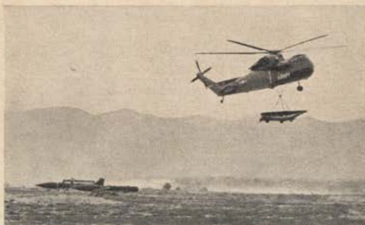
CHOPPER JOHN —Twin-engined Army H-37s (Sikorsky S-56s) airlifted Honest John missiles, launchers, and crews at Project AMMO, a missile demonstration at White Sands, New Mexico, and Fort Bliss, Texas, to show how helicopters provide mobility for Army missiles under combat conditions. Other Sikorskys flying at Project AMMO were H-34s (S-58s) and H-19s (S-55s).
