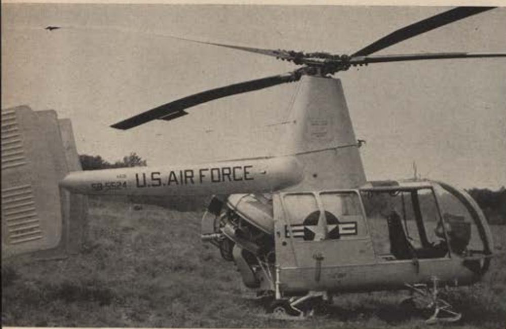
The Kaman H-43's servo-flap control helps create positive three-axis stability.
