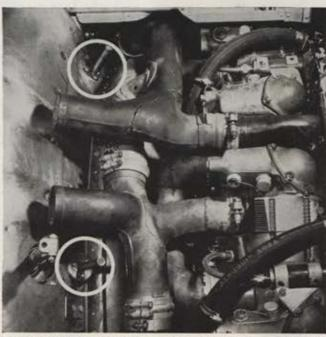
2. EASY INSTALLATION. Shown in Lockheed's transcontinental Super Constellation, these Fenwal unit Fire and Over-Heat Detectors are precision-set at the factory. Fenwal unit detectors eliminate the need for external relays, costly field adjustment and periodic maintenance. Fenwal units are in to stay — and stay right.
