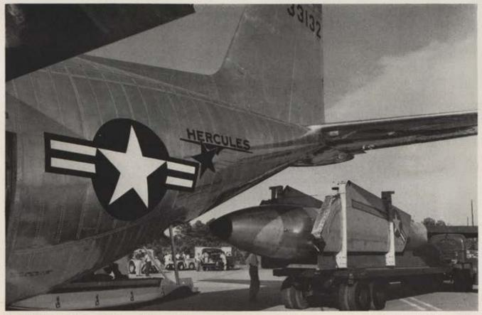
Martin TM-61 Matador missile could be rushed to any forward area at 400 mph speeds by Lockheed's C-130A Hercules.
