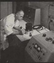
Seal testing by mass spectrograph
