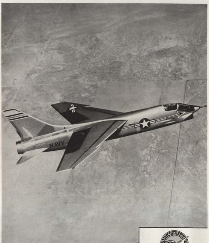
NEWEST SUPERSONIC FIGHTER, the Navy's Chance Vought XF8U-1, is a slender, sweptwing aircraft designed for air superiority missions in areas of sea operations. Throughout, the XF8U-1 is characterized by its uncluttered design and simple structure. It was built to take full advantage of the tremendous thrust of its Pratt & Whitney Aircraft J-57 turbojet engine.
