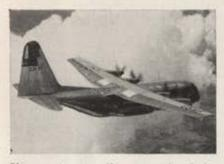
Slim engine nacelles, a mark of the turboprop, are evident in this shot.
