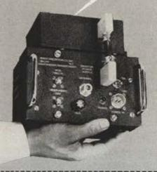
Radio Receptor's Miniature Transponder Beacon, Model RRco-XI, opens the way to once "impossible" applications. For instance, it is capable of full transponder beacon protection for short range liaison aircraft, helicopters, lifeboats and ground patrols.
