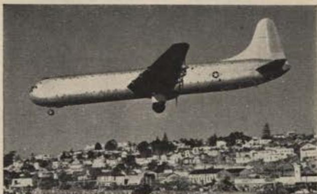
World's largest landplane, the Consolidated XC-99 has a wing-span of 230 feet and a length of 182 feet. It can carry 400 fully equipped combat troops. Top speed is well over 300 mph.
