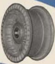
Bendix 56 x 16-inch wheel used on the latest type of jet bomber.
