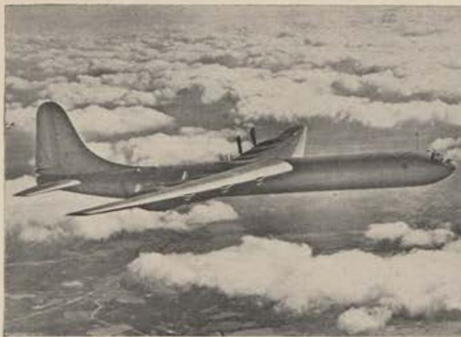
Sister ship of the XC-99, the B-36, proved itself beyond expectation last July when it flew a simulated combat mission of 6000 miles at an average air speed of more than 300 mph. The plane took off at a gross weight of over 300,000 pounds, the heaviest air load ever lifted. Craft was production model.
