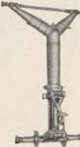
Bendix main landing gear shock strut, used on the newest commercial transport planes.
