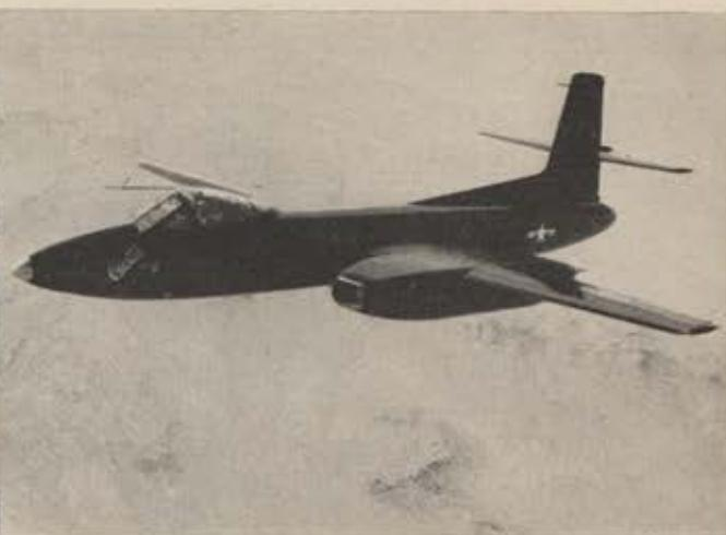
Heaviest fighter ever built, the Curtiss Wright XF-87 grabbed one of the ten most outstanding flights of the year by virtue of its highly successful initial test run at Muroc Air Force Base, California, last March. Craft was designed to do over 600 mph., with range of 1500 miles and ceiling over 35,000 ft.
