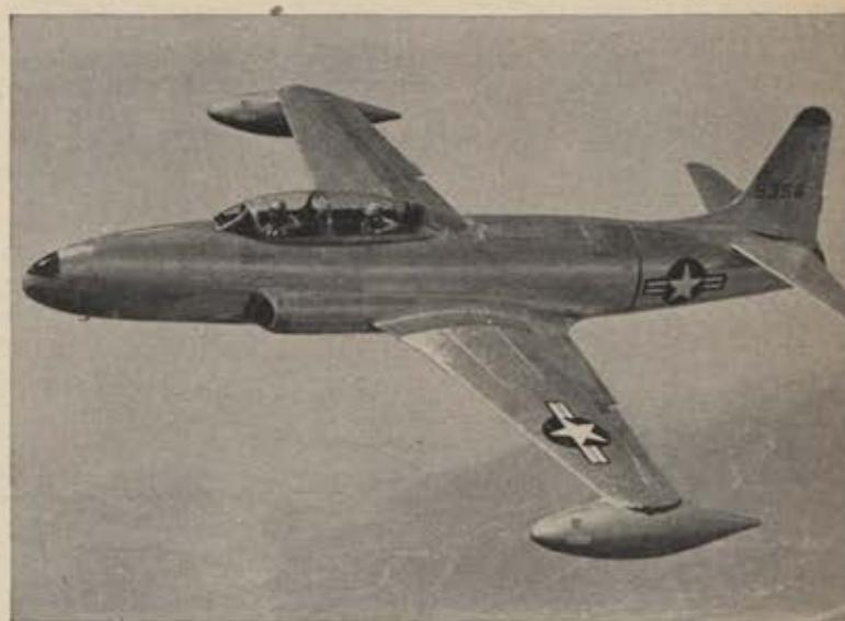
A two-place adaptation of the F-80 was introduced by Lockheed and USAF in the TF-80 above. Plane will be used to acquaint student fliers with jet operations and with split-second navigational problems incident to high-speed flight. Below, the husky Curtiss Wright F-87 all-weather fighter which is about as heavy as B-17. Production model will have only two engines.
