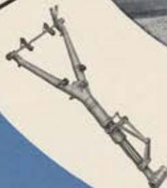
Bendix commercial transport nose strut, companion to the main landing shock strut shown above.
