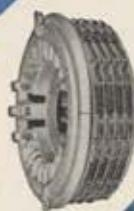
The Bendix segmented rotor brake—this four-rotor brake is designed for the high landing speeds of jet powered bombers.
