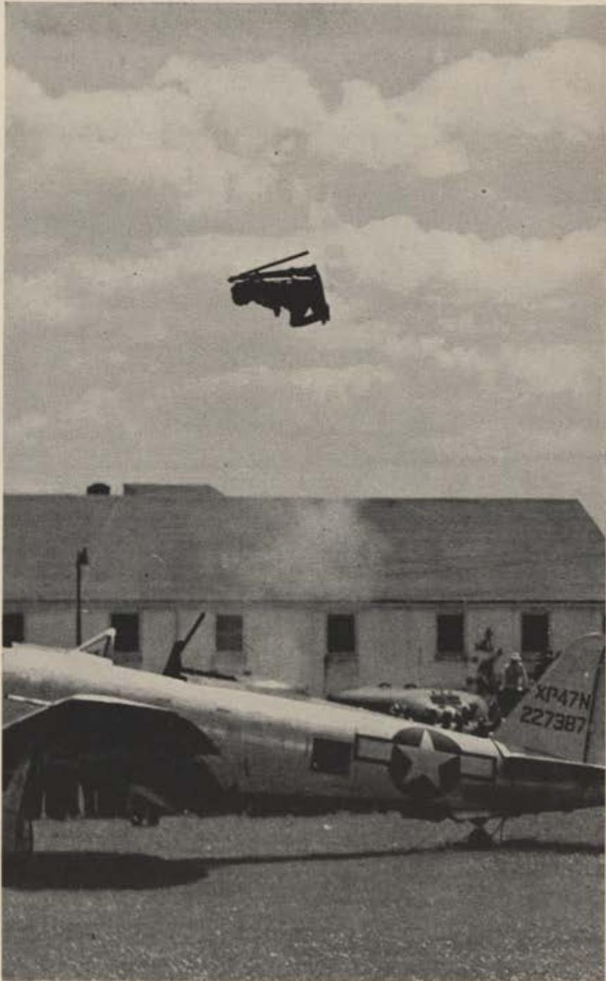
An early test, using dummy, in the development of automatic pilot ejection. Through ingenious device pilot can leave a disabled ship despite the extreme air pressure created by high speed flight. Automatic controls are a safeguard against blackout.
