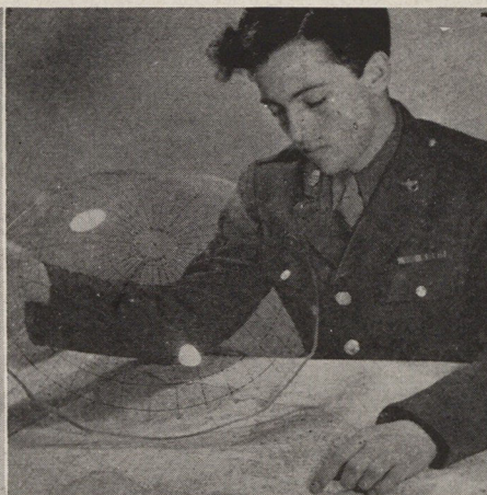
Before taking off, the navigator can plot course on wide-scale planning sphere chart (left) to determine which sphere-chart sections he will need for the flight, as well as coarse calculations such as direction and distance. Details are transferred to larger chart. Center, comparison between sphere and polar projection. Right, transferring plot information from small size planning to flight sectional spheres for actual use.
