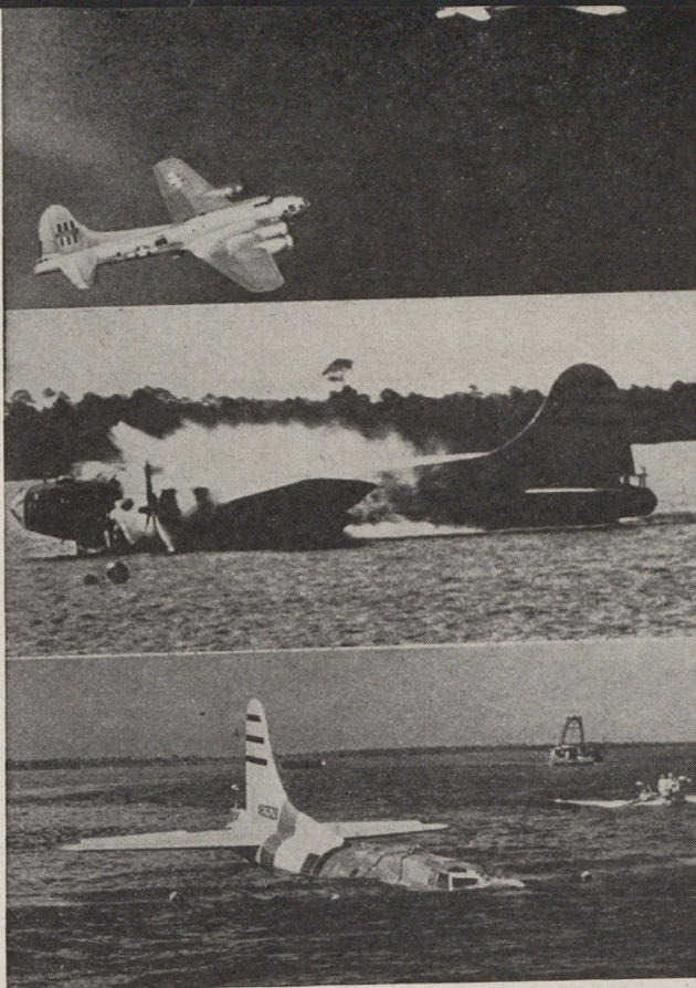
Part of a research program to develop safer ditching procedures, Air Matériel Command lands radio controlled B-17 in the water off Eglin Field, Fla. These drones were used in the Bikini tests.
