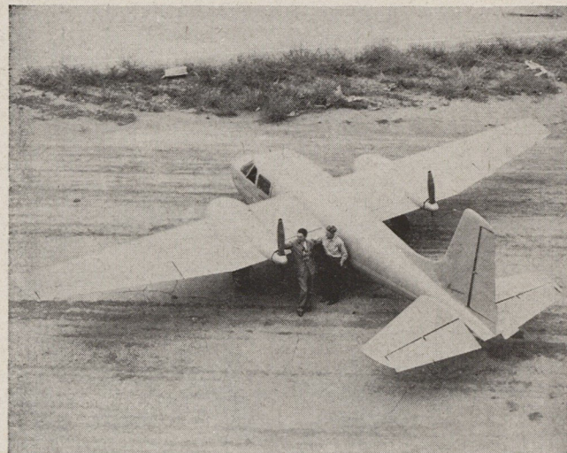
Top view of Baumann Brigadier Two-Fifty, five-place all metal pusher-type executive transport, powered by two flat-six 125 hp Continental engines. Cruising speed is 150 mph at 65% power.
