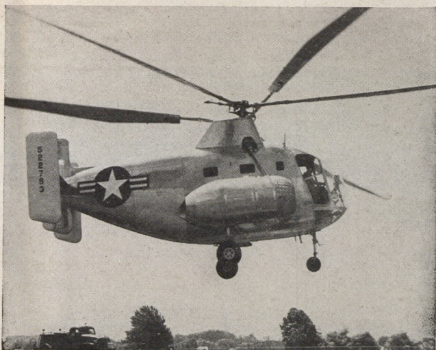
Largest helicopter ever accepted by the AAF, the twin-engined intermeshing twin-rotored Kellett XR-10 showed a ninety mph cruising speed and 350 mile range at initial running at North Wales, Pa.
