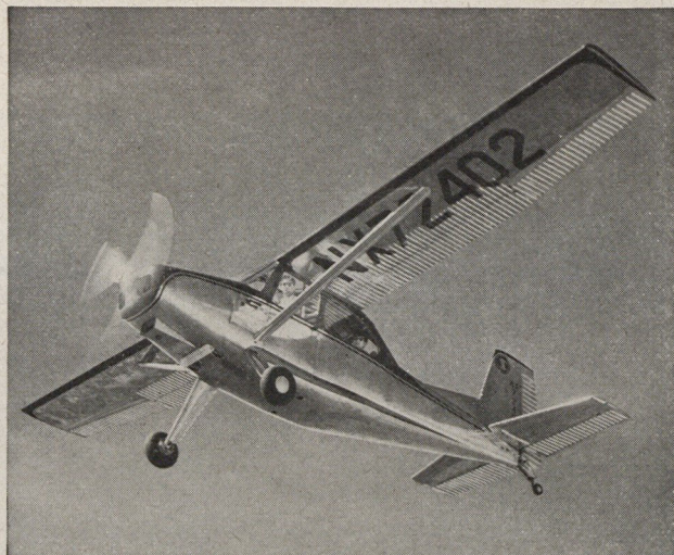
Luscombe's latest, the four-place all-metal Silhouette, was unveiled at the Flying Farmer's meeting at Oklahoma A&M in August. It cruises 500 miles at 130 mph on a 165 hp flat opposed six engine.
