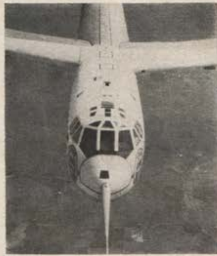
Specially instrumented B-52 with a fourteen-foot nose probe logged data on gusts faced in low-level flights.
