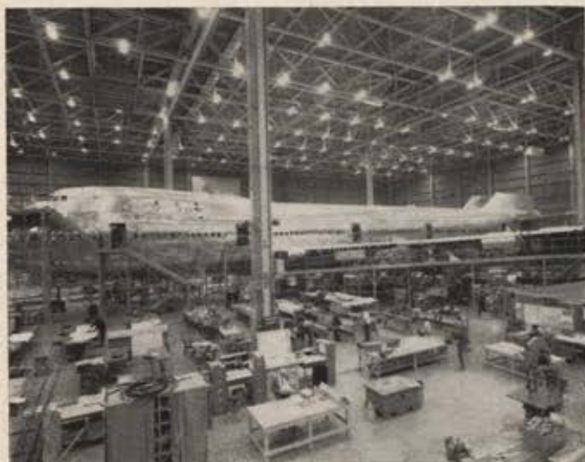
The mockup of the Boeing 747 is shown at Everett, Wash., plant where it is used by engineers to develop installations, components, and methods to produce the plane.
