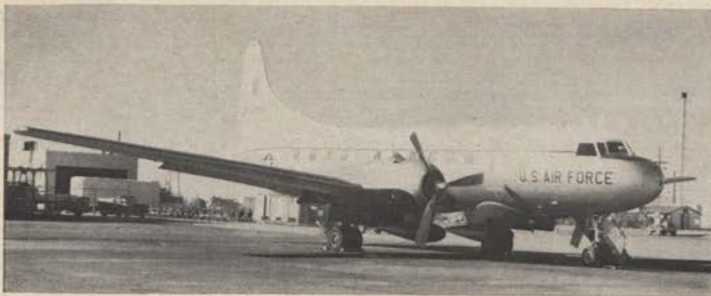
Convair C-131Bs, like this one at Holloman AFB, N. M., were employed by USAF pilots in searching out LO-LOCAT conditions. G-forces were recorded on visicorders, tape recorders, and digital computers installed in the cabin.
