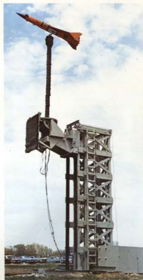
Models are installed on this 40-foot-high range tower for measurements of radar, antenna and passive radar augmentation patterns.
