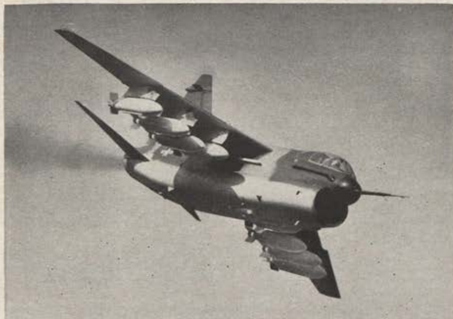
Allison-Spey TF41 engines for Air Force A-7D Corsair II tactical fighter are now coming off production line, with indications that first USAF A-7D squadron may be ready for Vietnam combat early next year. This A-7D is shown on test flight at LTV Aerospace Corporation plant in Dallas, Tex., powered by interim Pratt & Whitney TF30 engine and toting eight 700-pound ordnance tanks.
