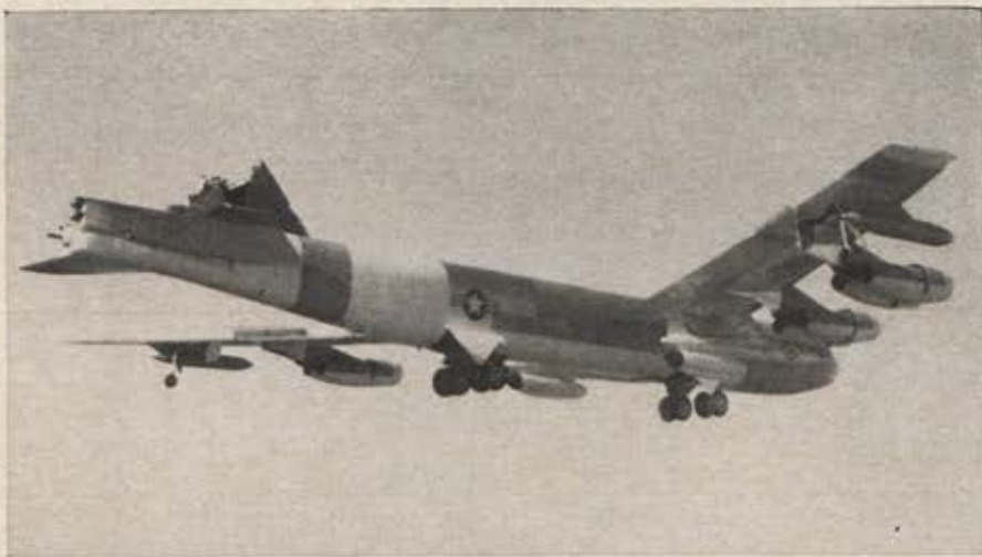
On a low-level test mission to obtain dynamic structural load data, this B-52H bomber lost a major part of its vertical stabilizer, but its four-man Boeing experimental test crew was able to land it safely at Blytheville AFB, Ark.
