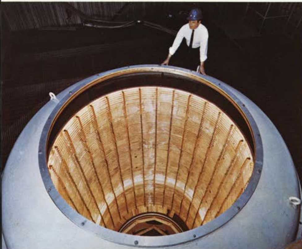
This radiant heating reflector assembly stands vertically inside a 20-foot high vacuum bell—part of the Beech Transient Heat Facility used for thermal studies of rocket and missile propellant tank systems and components.
