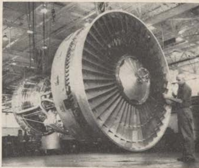
The Pratt & Whitney JT9D turbofan engine, which will power the Boeing 747, develops 43,500 pounds of thrust. Even more powerful engines are expected in the next decade.
