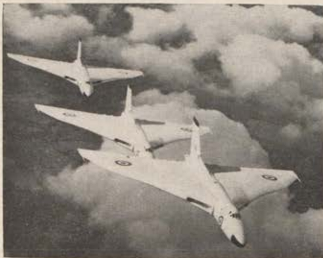
Principal weapon of RAF's new Strike Command is the Hawker Siddeley (formerly Avro) Vulcan, a four-jet medium bomber. It cruises at Mach 0.94 over a combat radius of about 1,750 miles. There are eighty in the RAF today.
