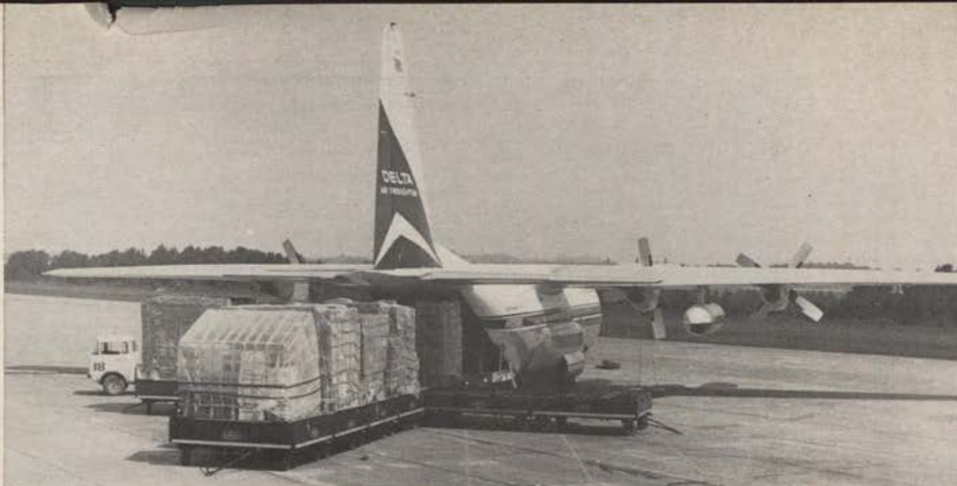
Newest version of the Lockheed Hercules (USAF's C-130 being used extensively in Vietnam) is the 100, a stretched version of the airfreighter. Delta Air Lines will have its three standard Hercules, one of which is shown above with its roller rail loading system in use, modified into the longer (100 inches) and thirty percent more productive turboprop freighters.
