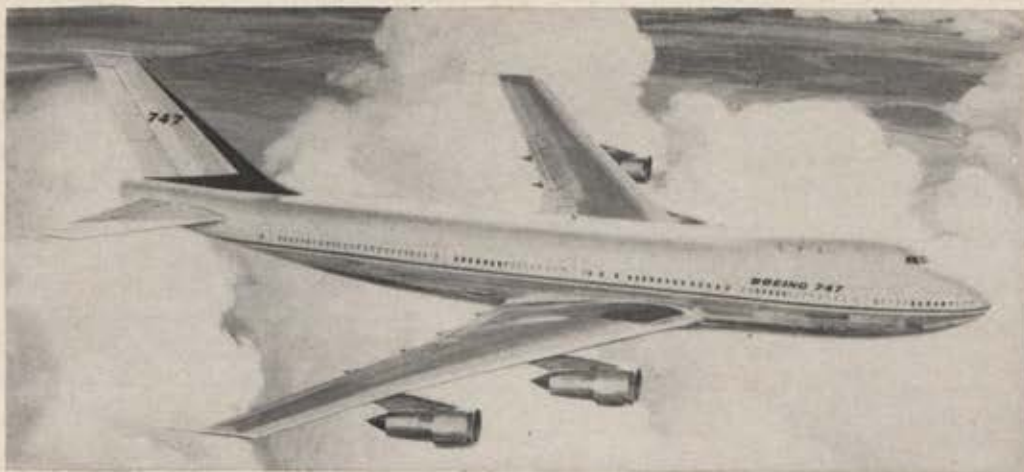
The cargo version of the Boeing 747, shown at left in its passenger configuration, will be able to transport a gross payload of 221,000 pounds across the country—four times the revenue ton-mile capacity of the 707-320.
