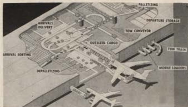
Part of the L-500 airfreighter total-system approach is the study of various terminal/cargo-handling possibilities such as artist's concept of automated complex above.
