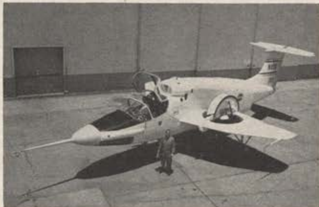
Employing unique fan-in-wing design, this Ryan XV-5B is undergoing flight tests in San Diego, Calif., before delivery to NASA's Ames Research Center at Moffett Field, Calif. Shown with plane, originally developed for Army as XV-5A, is Ryan chief test pilot William A. Armstrong.
