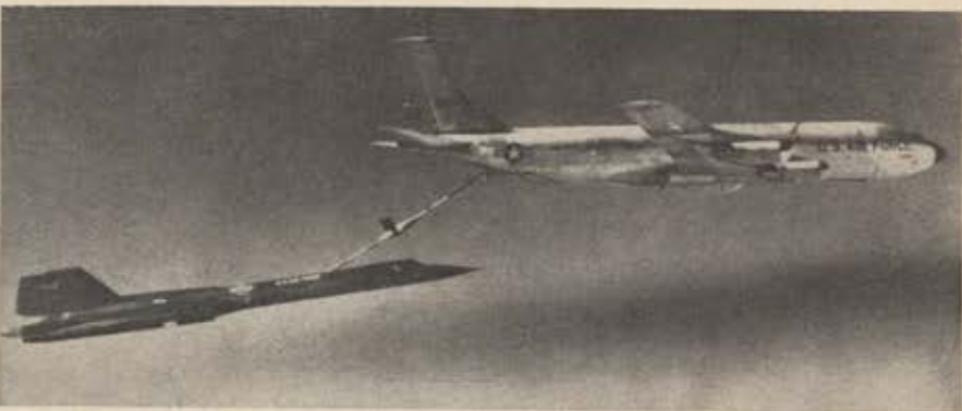
SAC SR-71s have initiated supersonic training flights over continental US. At normal 80,000-foot operating altitude, booms of triple-sonic plane will be muted, but they'll be more severe as it drops to be refueled by KC-135 tankers.
