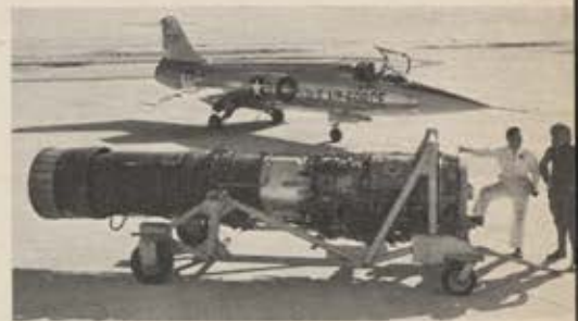
POWERFUL J79 TURBOJET ENGINE (above), product of the Aircraft Gas Turbine Division, Cincinnati, Ohio, recently powered the F-104 "Starfighter" to new world's speed and altitude records.
