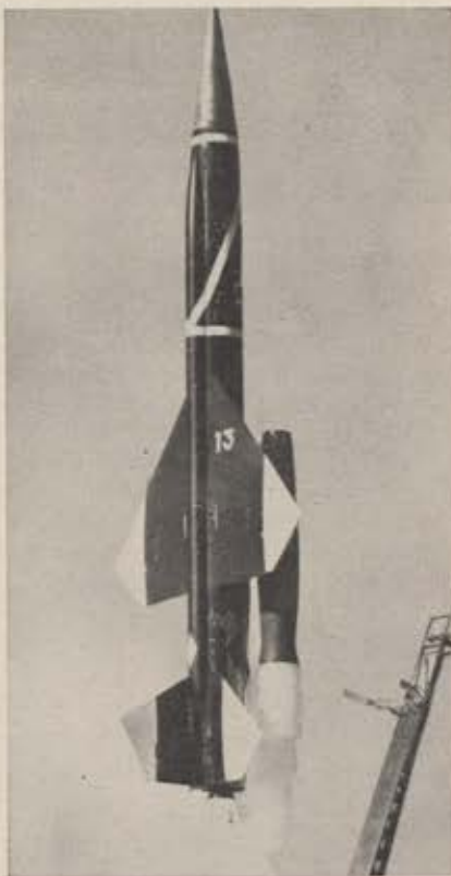
Bomarc supersonic missile, now in ADC arsenal, is launched vertically. The deadly "bird" is keyed to actions of SAGE.
