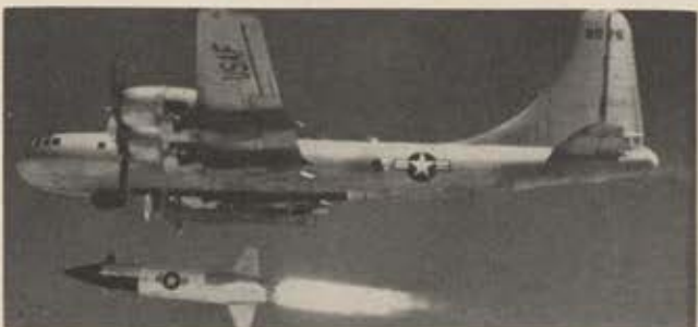
B-50 test bed drops GAM-63 Rascal.
