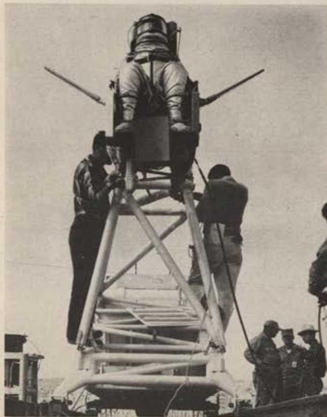
Subject clad in Air Force MC-2 high-altitude suit is readied for high-speed ride on rocket sled at Edwards AFB, Calif. Test will subject rider to terrific shock of windblasts.
