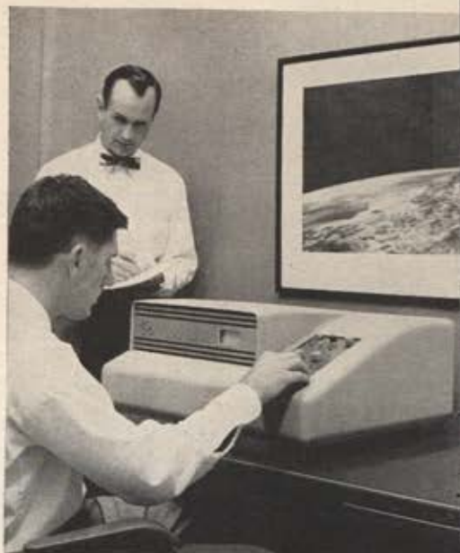
Prototype model of ASI Digital System Simulator. Unit is designed to give direct check of reduction of logical equations, to study a system's operations prior to construction, and to study alternate logical designs.
