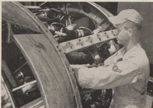
Air Reservist performs vital maintenance on C-119 engine.
