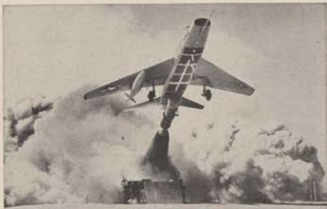
Zero launcher makes it possible for this F-100 to blast into the air at 275 mph without benefit of usual runway.
