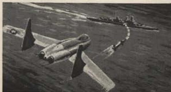
Jam-proof Missile Guidance attains new accuracy and reliability through control by modulated light.
