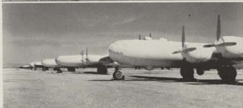
At Davis-Monthan AFB, Ariz., the stripped B-29s and B-50s are covered by white plastic cocoons to protect them from the weather. Here at the 3040th Aircraft Storage Squadron's depot, all salvageable parts are cleaned, crated, and shipped to supply depots for eventual installation in active aircraft.
