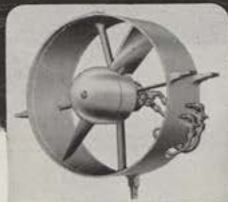
Production units of Aeroproducts Ram Air-Driven Generator (left) have been installed on the Navy's Douglas A4D Skyhawk; Aeroproducts Ram Air-Driven Hydraulic Pump (above) is scheduled for installation on jet fighters.
