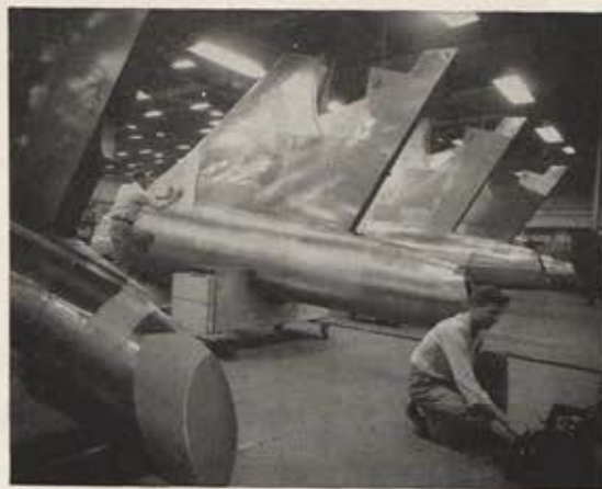
Final assembly and inspection of aft fuselage section of F-101 prior to delivery to McDonnell.
