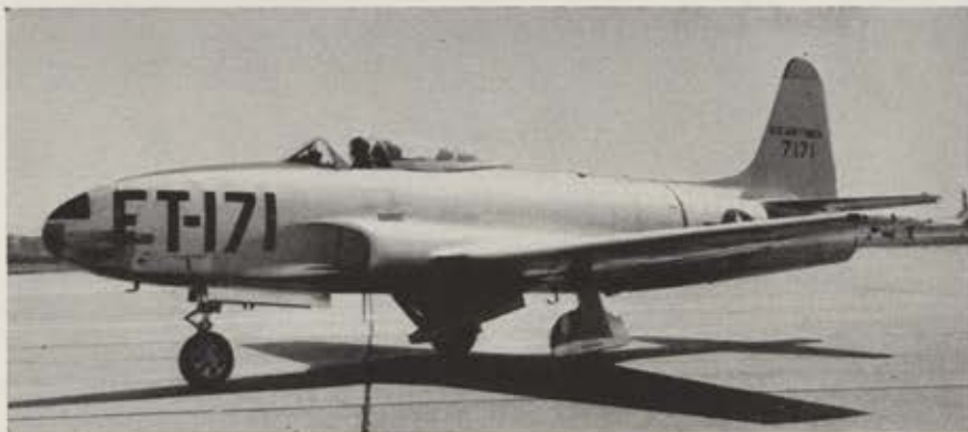
First all-magnesium airplane was flown recently. It is being tested by ARDC.
