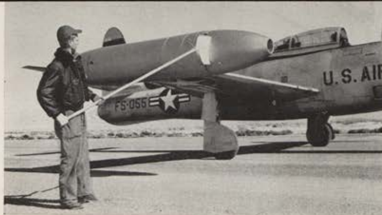
A/2C Thomas O. Summers keeps a safe distance from a "hot" F-84 sampler plane of the 4926th Sampling Squadron as he removes the wafer containing an atomic cloud sample from the cloud-busting aircraft's tip-tank slot.
