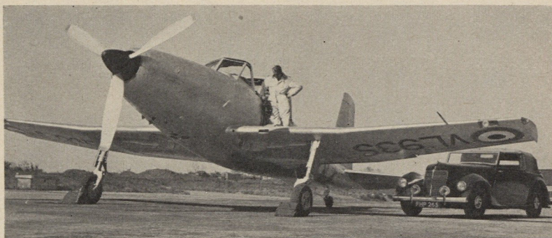
Price Owen, chief test pilot for England's Armstrong Siddeley aircraft factory, climbs into the cockpit of the new and strikingly efficient Balloil, powered by a Mamba gas turbine engine. The engine weighs but 1000 pounds and has 1000 hp. The engine in the car, by comparison, weighs 3000 pounds and has only 16 hp.
