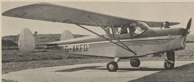
Another British development, this one in the personal plane field, is the new "spin-proof" Chrislea Super Ace, now in production at Exeter, England. Plane will carry four people with ample luggage room. Skis or floats can be used interchangeably with regular gear. Note car-like roominess and good vision.
