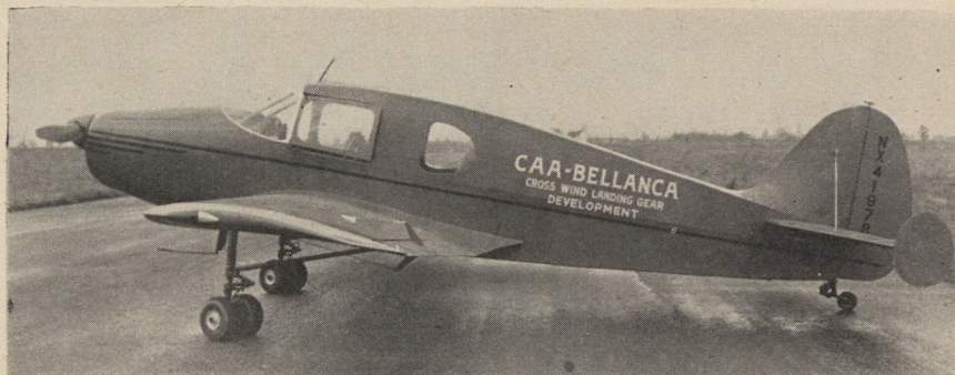
Latest achievement in the cross-wind landing gear program is introduced by Bellanca Aircraft Corp. of New Castle, Delaware. Bellanca is unique in that it features a dual wheel arrangement which eliminates much of the shimmy. See More X-Wind Gear .
