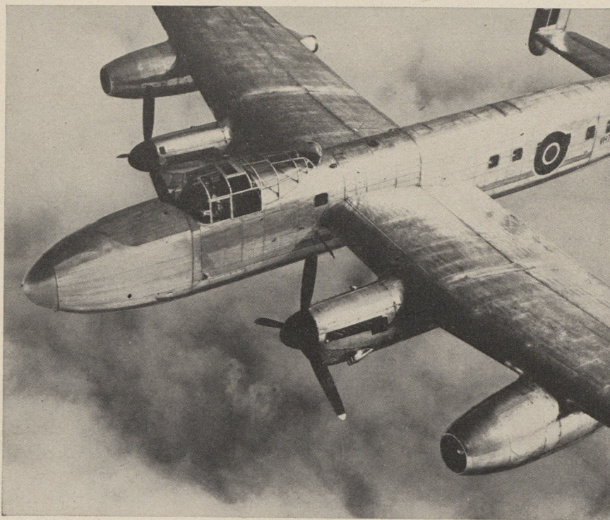
To date England has moved ahead faster than the US in research into the feasibility of applying jets to commercial airliners. One of the earliest experiments (above) was with a converted Lancaster bomber on which two Nene-Merlin jets were installed.
