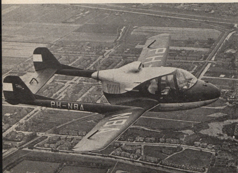
Winner of first prize as best small taxi and feeder plane at recent Paris International Air Show, the four-place 150 hp Dutch-built Fokker has a cruising speed of 140 mph. The new type is pusher for safety and forward visibility.
