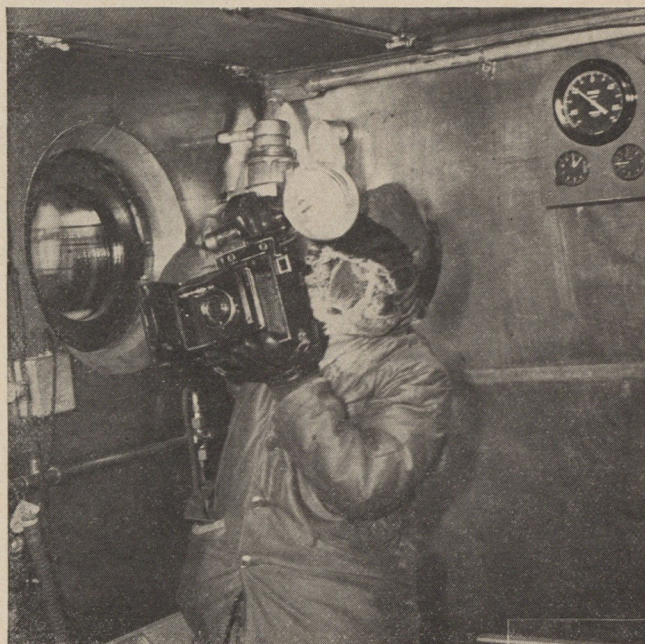
Within the temperature-controlled altitude chamber, pressure can be dropped to simulate 100,000 feet. Photographer shown above is shooting while thermometer, shown behind him, indicates -40^{\circ}\text{F} .
