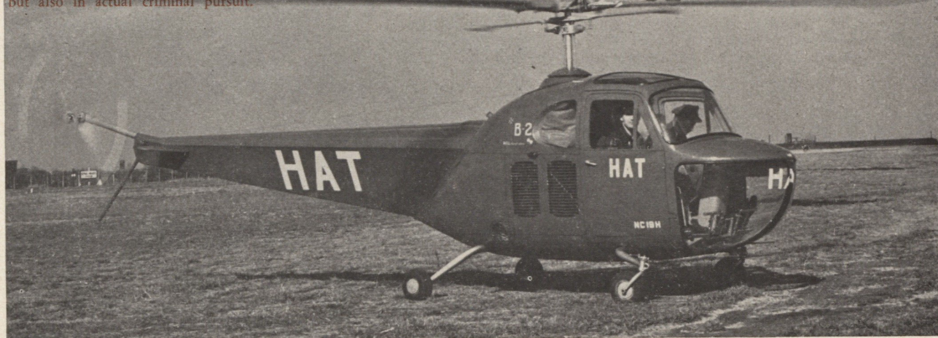
HAT's flying courses are given either in the two-place 178-hp Franklin-engine Bell 47s (front three craft) or in 450-hp Pratt & Whitney Wasp engine 4-place Sikorsky S-51s, like the top two ships.
