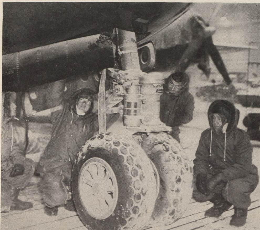
At minus seventy, APGC crews examine landing gear of a B-29 for operating conditions inside the giant climatic hangar at Eglin Field in Florida. GI clothing for arctic conditions is tested at the same time.
