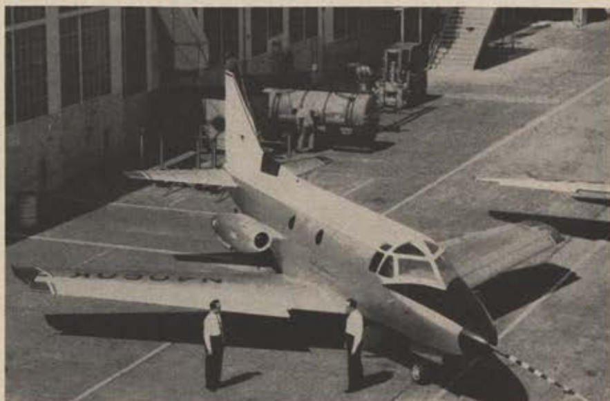
North American's new utility jet trainer, the Sabreliner, has a top speed of 575 mph. It has a wing span of forty-two feet and a gross weight of 15,320 lbs.
