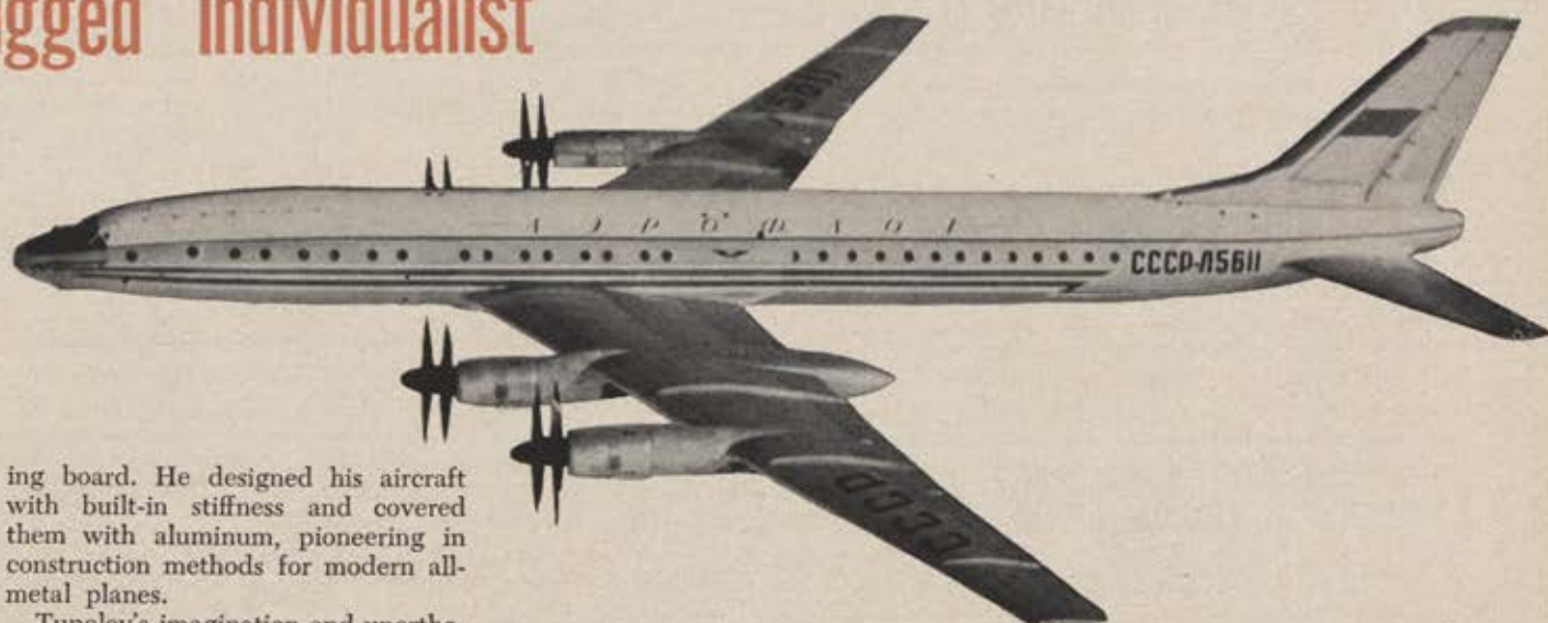
The enormous four-engine turboprop transport, TU-114, was built for Aeroflot, the Red airline, under supervision of Tupolev. Reds say it will soon be in service.
