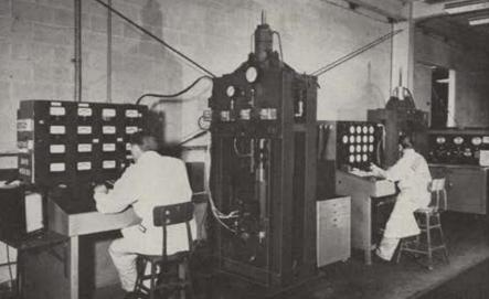
Expert laboratory technicians test stabilizer actuator for accuracy and operating characteristics using special Western Gear designed test stand which provides control instrumentation and automatic cycling.
