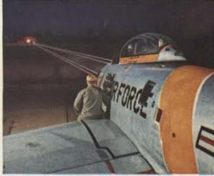
TO WIN AND HOLD AIR SUPERIORITY — On target! Night bore sighting exercises make sure planes are ready for gunnery. TAC aircraft can also deliver air-to-air rockets, powerful A-weapons.
