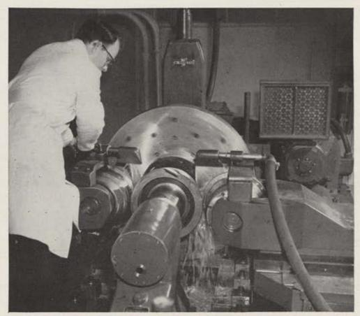
Opposed heavy-duty steel rollers cold-flow tough materials onto a spinning mandrel
