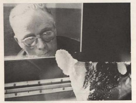
A research mechanic peers through a window at an ice build-up on a model airfoil section during a test in a new icing tunnel at Boeing's Seattle plant. Facility permits study of airplane icing conditions under controlled situation.
