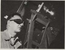
Test specimen glows as it is moved into the focal point of the furnace.
