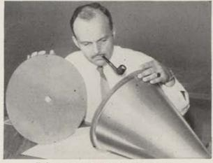
Hydrospin turned out the cone with integral flange from the simple disc at left
