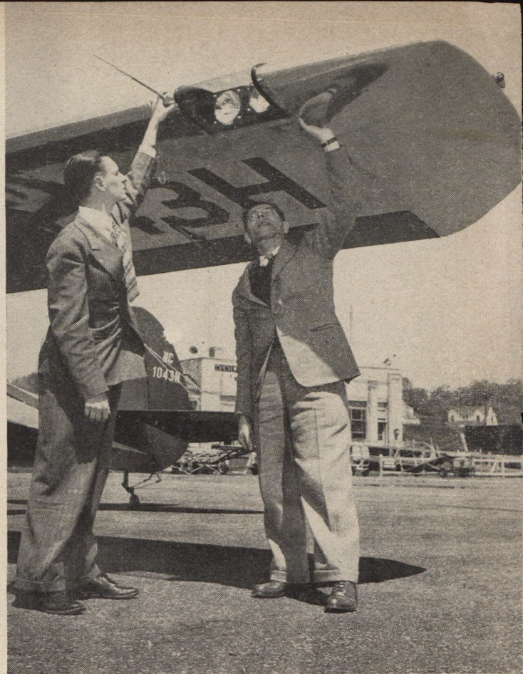
Arthur Dean, left, and Samuel Gordon, general observers, inspect landing lights on the new Aeronca. One points straight ahead, the other is canted downward for taxiing. Wing skin is all metal.
