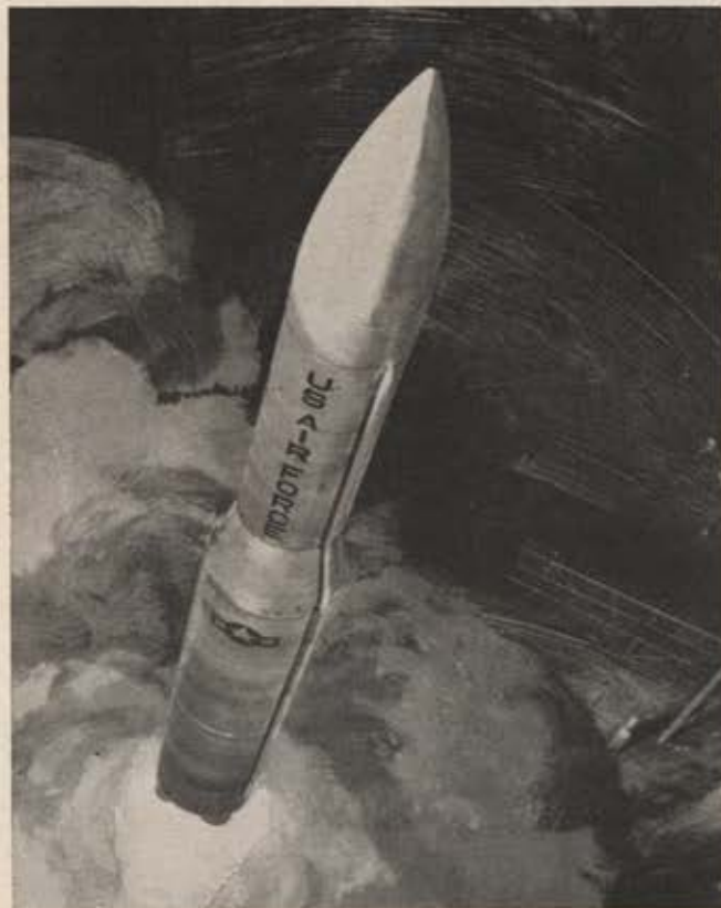
This artist's conception of the USAF Minuteman III, newest version of the solid-fuel ICBM, illustrates bullet-shaped shroud which covers new reentry system. Larger third-stage engine increases the missile's flexibility and payload.
