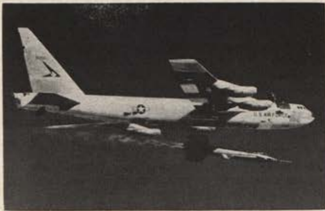
One finding of X-15 program was that pilots experienced excessive heart rates just before launch from the B-52, indicating tense anticipation rather than physical stress. Above, one of the early airdrops from B-52 mother ship.
