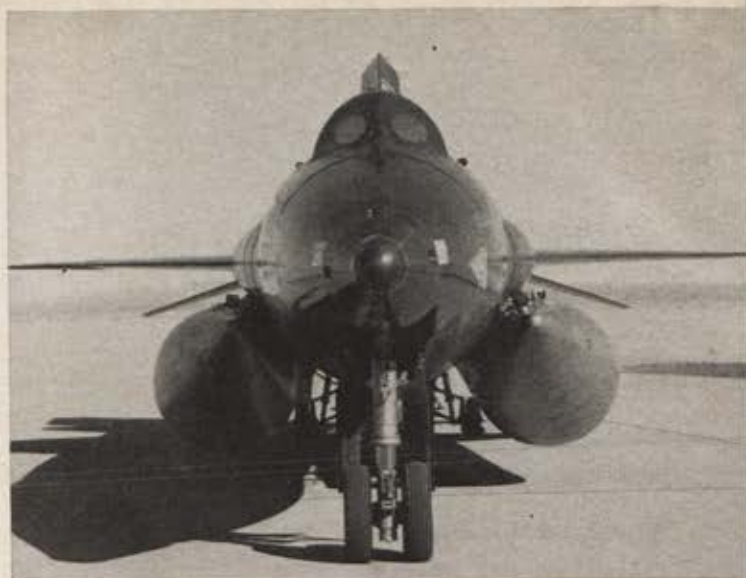
Front view of X-15 with auxiliary propellant tanks, which are jettisoned during flight and recovered by parachute housed in tank forward section. Ball nose of aircraft is attitude sensor. Note elliptical windscreens on cockpit.
