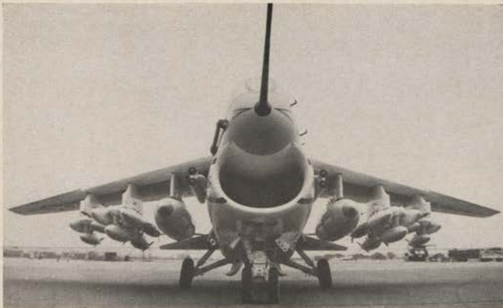
The Ling-Temco-Vought A-7 Corsair II aircraft, shown here in its A-7A Navy version, will soon be in use with the Air Force, providing it with significant new tactical capabilities, including a greater load-carrying capability and greater range than any other single-jet aircraft, all-weather/day-night attack capability, and probably the best maintenance-to-flight-time ratio of any jet in service.
