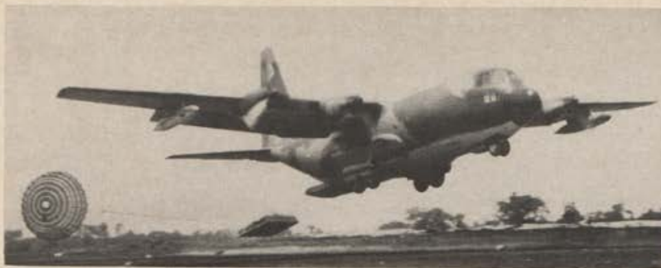
A method of delivering cargo that has greatly increased accuracy of delivery of supplies in the combat area is LAPEDS (low-altitude, parachute-extraction delivery system), which allows C-130s to put pallets of cargo exactly where they are needed for ground troops.
