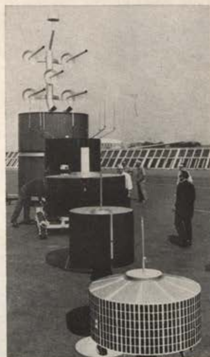
USAF's 10,000-channel experimental tactical communications satellite in rear dwarfs its predecessors. From front are Syncom, world's first synchronous communications satellite, Early Bird, Intelsat II, and ATS-1.
