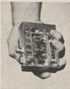
The up-link-receiver (C-band) shows rugged state-of-the-art construction.
