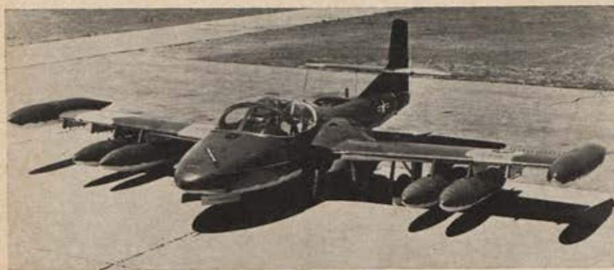
First of thirty-nine Cessna A-37A attack aircraft ordered by USAF is now undergoing field tests at TAC's Air Commando Wing at England AFB, La. At gross weight of 12,000 pounds, it will carry more than 4,800 pounds of ordnance. Air Force is also buying fifty-seven A-37Bs as replacement for A-1 Skyraiders and T-28s.
