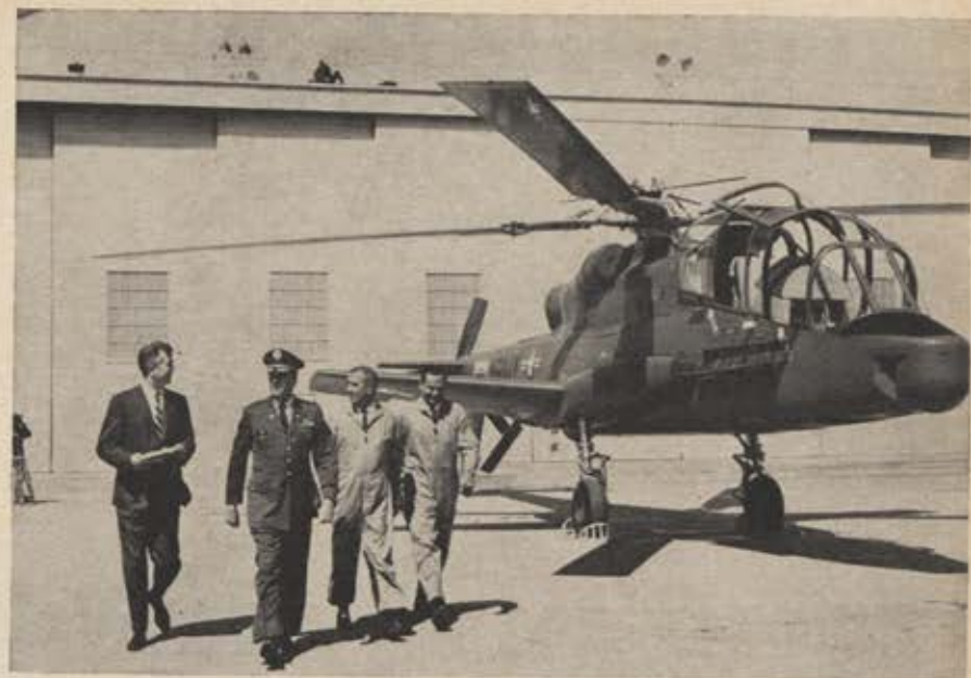
First prototype of US Army's AH-56A Cheyenne, formerly called the Advanced Aerial Fire-Support System (AAFSS), was unveiled early in May at Lockheed-California Company's Van Nuys plant. The rigid-rotor compound aircraft, designed to cruise at 240 mph, will be armed with rockets, wire-guided antitank missiles, a grenade launcher, and belly machine gun. From left in photo are Jack Real, Lockheed's AH-56A manager; Lt. Col. Woodbury Johnson, Army project officer; and Herman Salmon and Don Segner, Lockheed test pilots.
