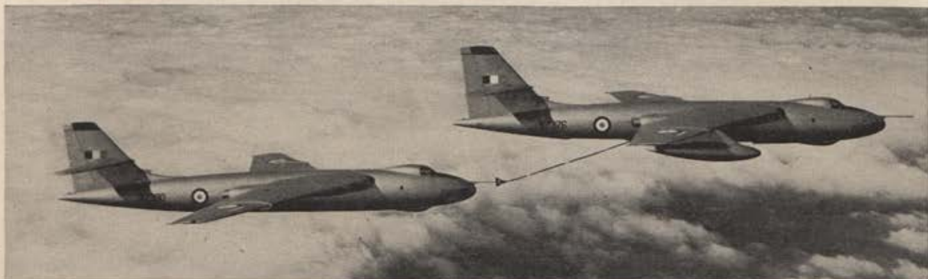
V-force capability is being increased by use of probe and drogue aerial refueling, here demonstrated by two Valiants.
