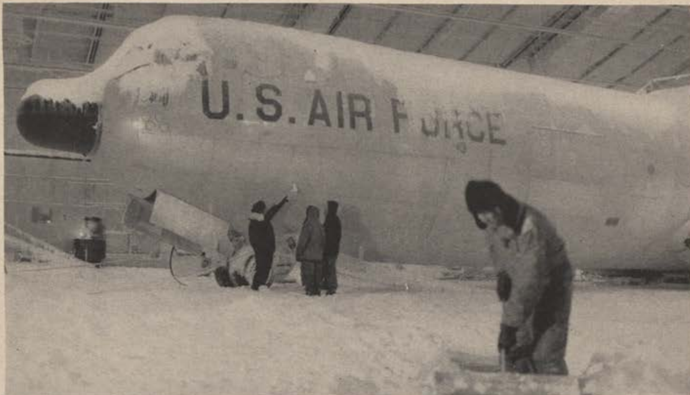
Giant C-133 turbo-prop transport is tested at -65^{\circ}\text{F} in mammoth ice box at Air Proving Ground Center, Eglin Air Force Base.
