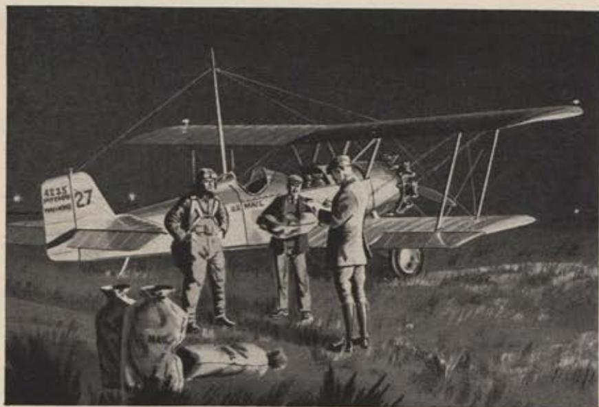
ARC installed first radio range receiving equipment, with six foot rigid rod antenna, which was used on "Mailwing" biplanes by Pitcairn Aviation, 1928.
