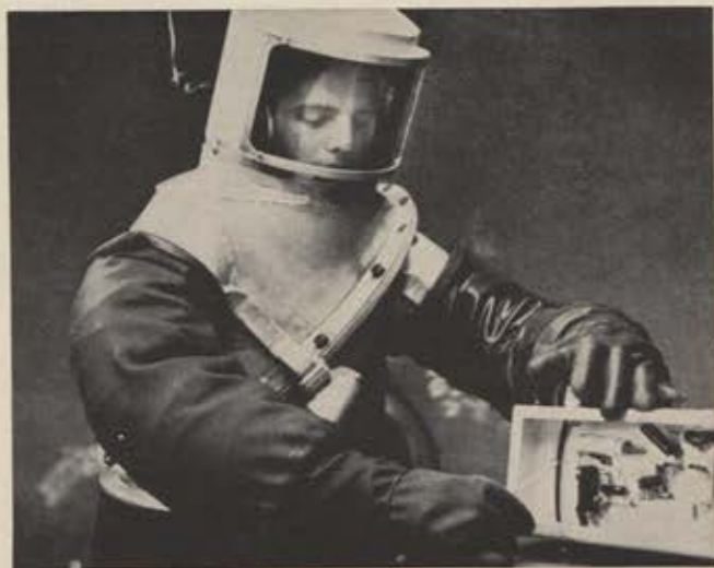
Man in a vacuum. Experimenter in AFOSR-Litton High Vacuum chamber demonstrates ability to work while in the suit.
