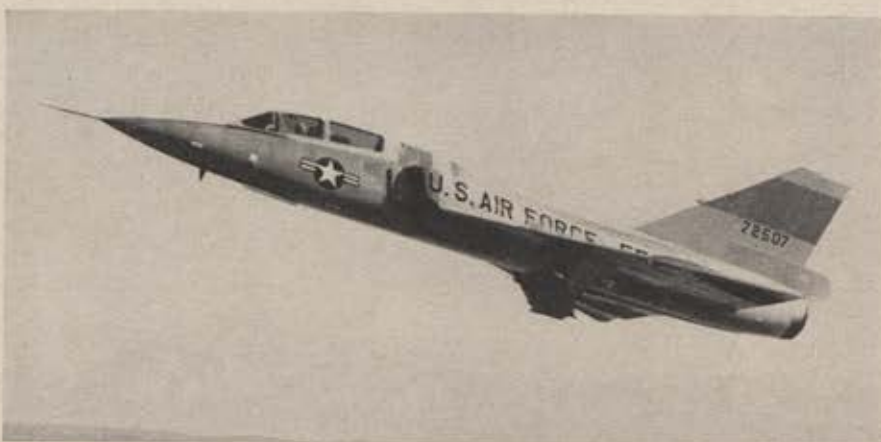
First flight photograph of Convair's F-106B two-place, all-weather jet interceptor, shows fighter retracting its landing gear after takeoff from Edwards AFB on its maiden test flight. The F-106B is externally identical to its sister F-106A except for the second seat and the longer canopy. The flight was supersonic.
