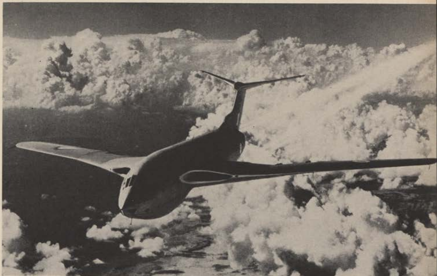
The Handley Page Victor is a crescent-winged, four-jet craft with cruising speed of more than 700 mph at 60,000 feet.
