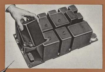
The Master Air Data Computer provides a single coordinated source for input information required by the various aircraft control and instrumentation systems. It is a central "clearing house" for aerodynamic intelligence. There is no fundamental limit to the number of functions, outputs or services that this computer can perform.
