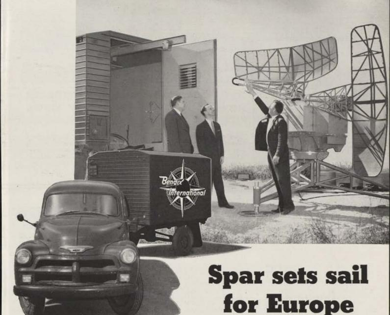
Bendix-International recently took delivery of its first SPAR, the low-cost portable GCA radar. The equipment went directly from Laboratory for Electronics' test field at Norwood, Mass., above, to foreign markets for demonstration before fourteen interested European governments.
