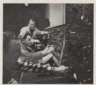
3. SIMULATOR EQUIPMENT evaluates the J47's integrated electronic control operation, finds a compressor discharge pressure sensor unit to be out of tolerance...
