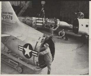
1. HAMILTON AFB MAINTENANCE SYSTEM IN OPERATION. In this typical case history, a G-E J47 is removed for routine check. Trouble is suspected. Engine sent to test . . .
