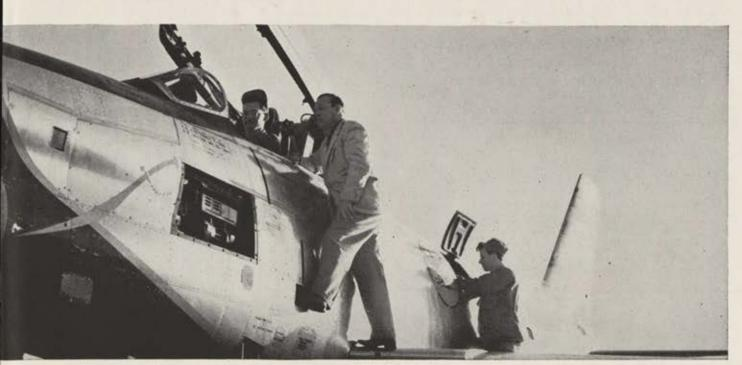
5. FINAL TESTING. A special seven-man run-up crew checks J47 out in F-86D. By using a single crew for all J47 run-ups, the 325th Fighter Interceptor Squadron at Hamilton has reduced the number of personnel required for run-ups by two-thirds.
