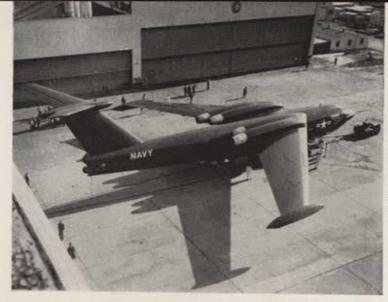
Martin's XP6M-1 Seamaster. Bombers based on water could be dispersed easier.
