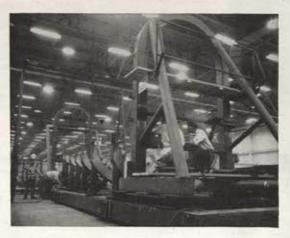
Tooling up for the B-52 job, these TEMCO workers are building the huge jigs in which major fuselage sections will be fabricated.
