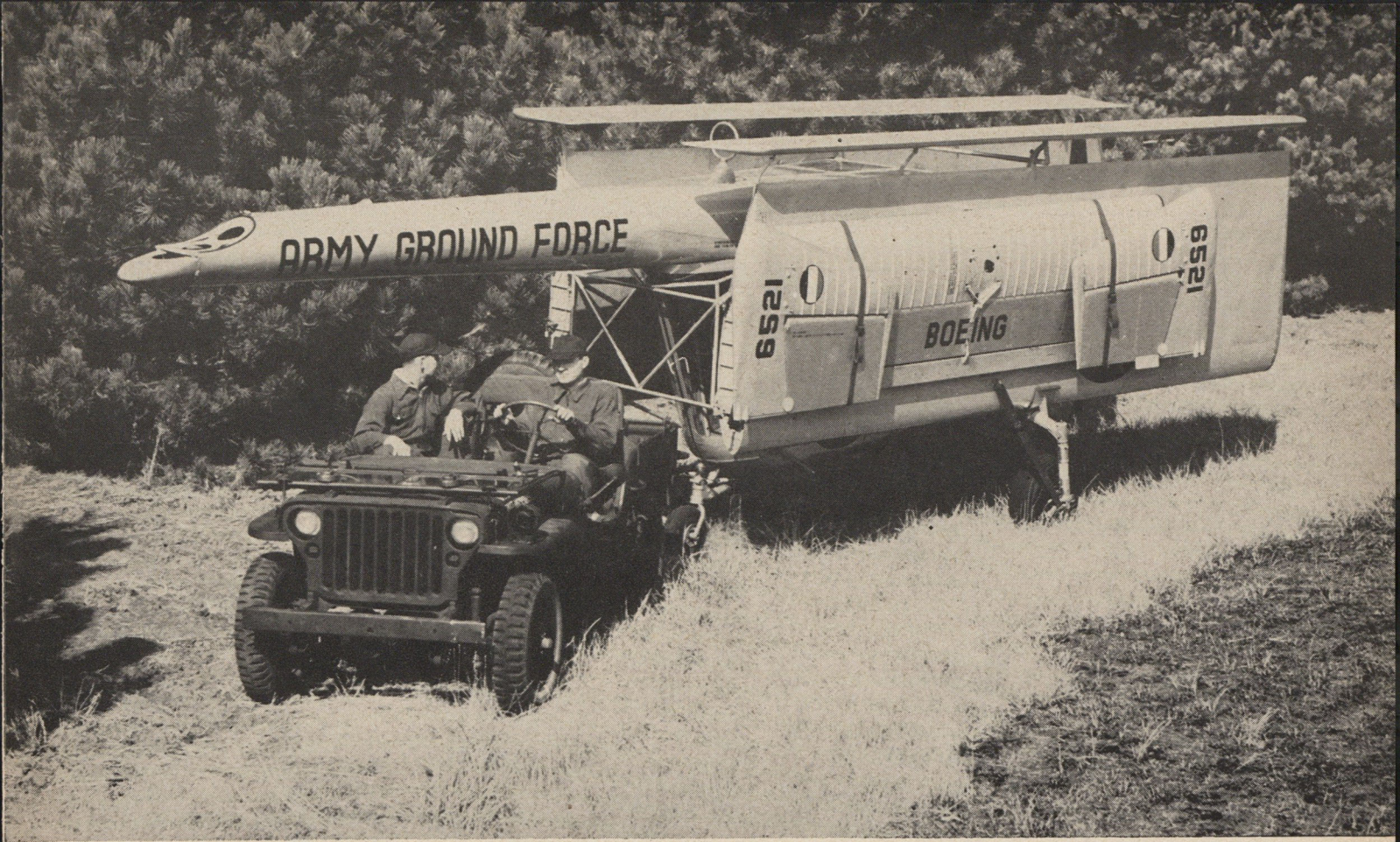
Knocked down and packaged, the L-15 can be towed at 40 mph on its own wheels by a jeep. Prop removed, it can be snatched off ground and towed, glider fashion.
