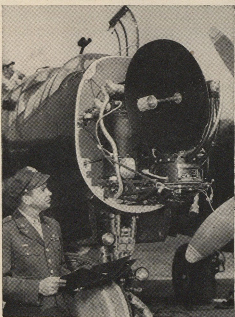
Plastic nose of P-61 is removed to show great amount of radar used in collecting storm data.
