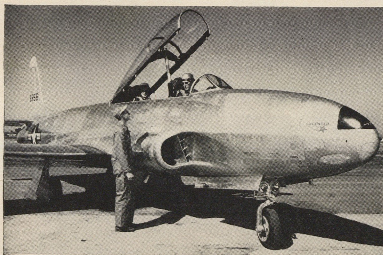
In California, Lockheed Aircraft introduced the new two-place jet trainer, the TF-80C, a modified Shooting Star with the fuselage lengthened by 38 inches. Here test pilot Tony LeVier tries out the front cockpit while F. E. Gaiser, Lockheed engineer, smiles from rear. Canopy is 7 feet long.
