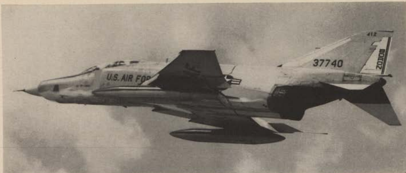
New materials have been critical in aviation since wire bracing, wood, and canvas gave way to sheet aluminum. Improved aluminum alloys, titanium, and beryllium lowered structural weight still further in the 1950s and 1960s. Biggest strides ever are expected with metal/plastic composite materials in the 1970s. First major production involves boron rudder for the F-4 Phantom aircraft. This material shows excellent potential for reducing structural weight by almost one-third.
