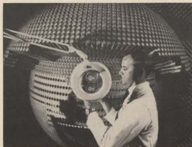
This antenna is one of several in the one-tenth-scale prototype of advanced design array radar (ADAR) being built for the Air Force by Hughes Aircraft Co., Fullerton, Calif. The phased-array radar, the most powerful yet built, is designed to be a sensor for satellite identification and as a ballistic missile defense designation/discrimination sensor.
