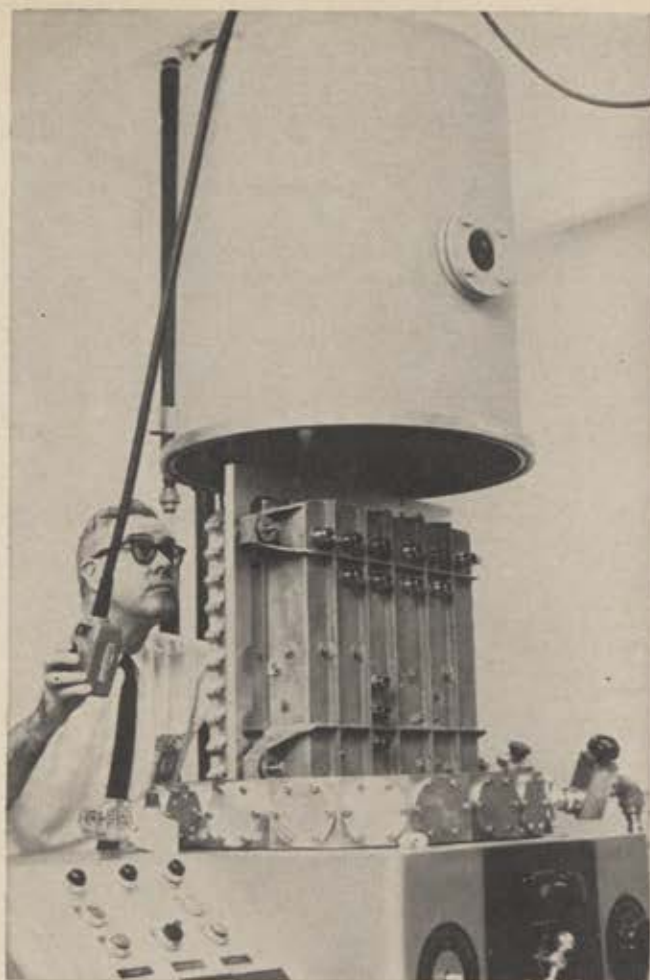
Experimental work indicates that airborne computers will continue to shrink; work capacity will increase. Sperry Rand-Univac model, above, flew for first time on Titan III this year, has 1.8-cubic-foot volume, and performs 125,000 operations to deliver fifty steering commands per second.
