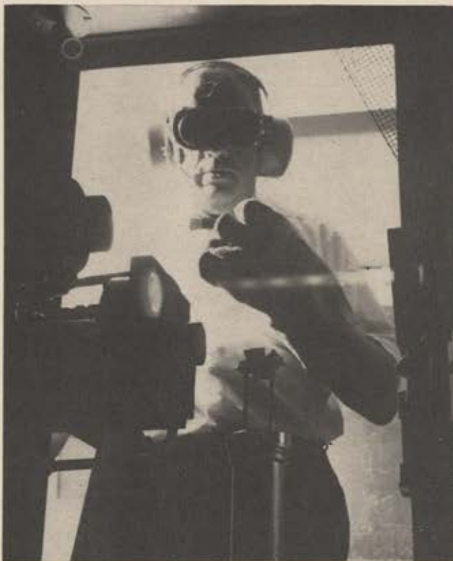
New materials are needed for most systems. Boeing engineer above is working on ceramics for face of radar which can withstand close-by nuclear blast. Samples are heated to 3,500° F. and then their ability to pass radar signals is measured. Ceramic is tougher than granite in impact tests.
