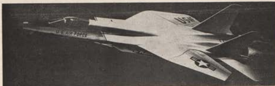
To match the Russian tactical fighters expected to replace the MIG-17 and MIG-21, USAF proposes, in its FY 1969 budget, an advanced tactical fighter, the FX, shown in artist's concept at left, with variable-sweep wings and improved maneuver capability.
