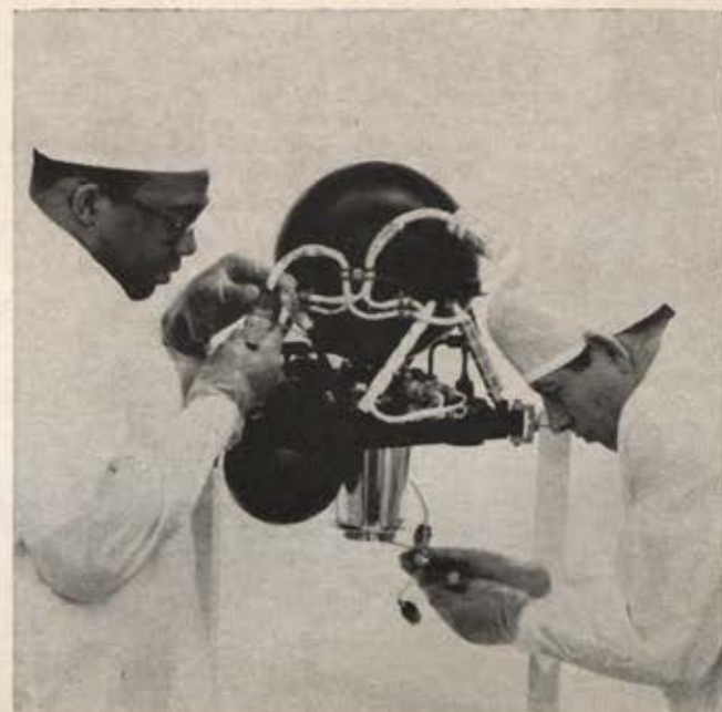
Mars will be the target of a pair of Mariner spacecraft expected to be launched by NASA in 1969. Above, technicians make final checks on a test engine at TRW, Inc. The hydrazine engine will perform midcourse corrections.
