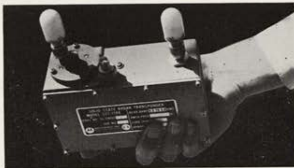
THIS IS A MOTOROLA SST-119X: It is one of a complete family of off-the-shelf, low-cost S-, C-, X- and K-band transponders, any of which may be crossbanded to accommodate special requirements.
