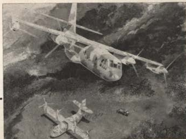
Another proposal being studied for the LIT is the tilt-wing V/STOL technique shown in the artist's concept above. This approach was tested extensively with the LTV XC-142 and is available in the Canadair CL-84 transport.
