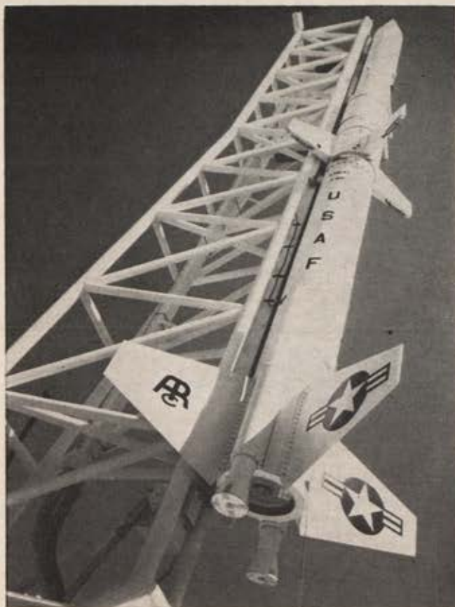
One-hundredth Athena missile, part of advanced ballistic reentry study, was launched from Atlantic Research Green River, Utah, site on March 29. Missile's 470-mile flight duplicates 6,000-mile ICBM path, but can be fired overland.
