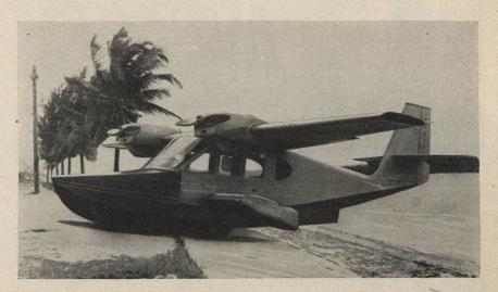
See New Amphib. The Aqua-1 six-place amphibian, powered by two 125 hp Lycoming engines. In a recent shakedown flight, the new craft indicated a cruising speed of 130 mph at 75% of power. Newest NACA non-porpoising hull-shape is featured.
