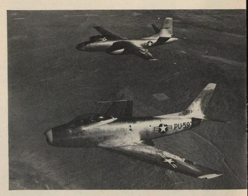
Here are two of the "most modern" planes Senator Taft urges the US to build in sufficient numbers each year so that practical tests can be assured. Top, the North American B-45 four-jet bomber. Below, North American's jet P-86 fighter.
