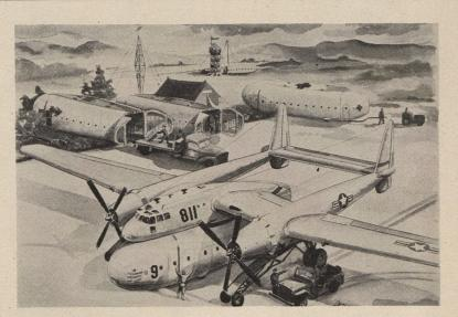
Pack-plane. Artist's conception of the new Fairchild XC-120, which will allow pod-like lower nacelle to be detached from the cockpit and center section. These pods have the capacity of 2900 cubic feet and can be constructed to serve a variety of uses; cargo, ambulance or complete operational units. Performance will be similar to the C-119.
