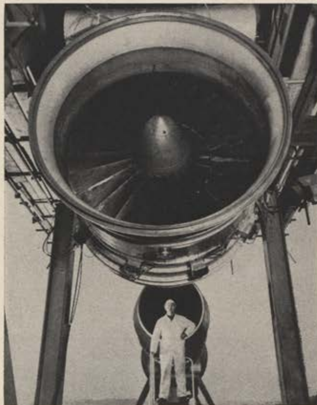
The British aero-engine industry has been most successful in its export efforts. The Rolls-Royce RB.211 shown in this picture is slated to power Lockheed's 1011 airbus. This turbopan is of a novel three-shaft design offering much improved maintenance conditions, excellent economy, and relatively uncomplicated construction. Engines of this type hold the promising prospect of helping to maintain British manufacturers' leadership in the field of jet engines.
