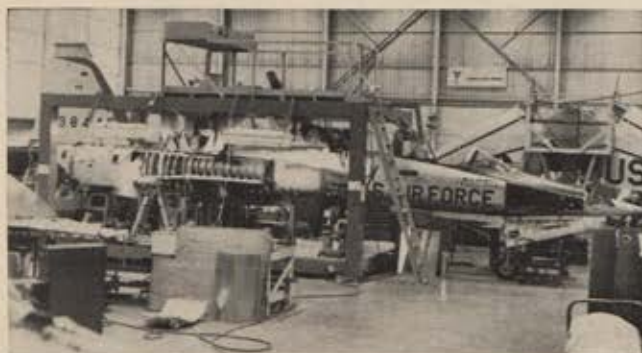
Northrop engineers working on an advanced version of the F-5 fighter for the Air Force. The new configuration, designated the F-5-21, will feature two 5,000-pound-thrust GE J85-GE-21 jets that are to provide about twenty-five percent more thrust than the engines in the F-5A and -B.
