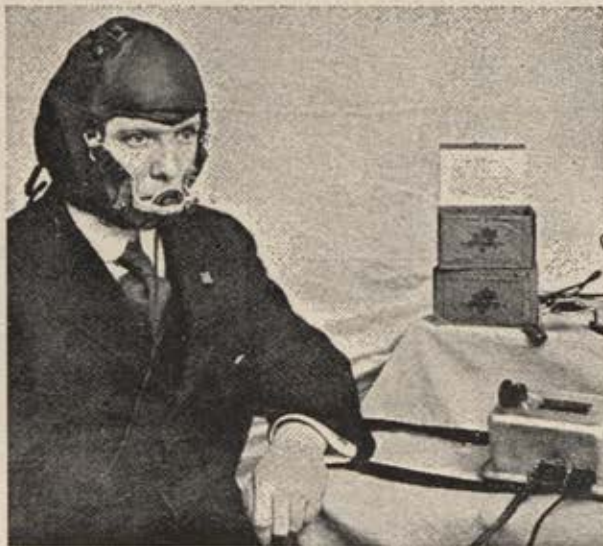
Edwin S. Pridham, Magnavox founder, demonstrating anti-noise transmitter that enabled WW I aviators to communicate with other aircraft and ground stations.
