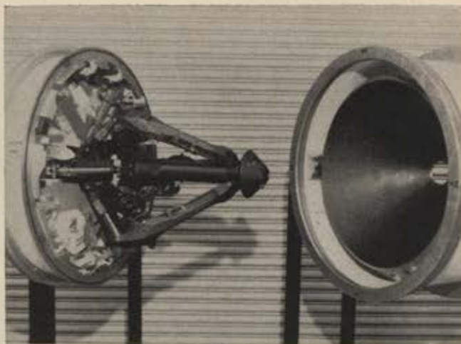
North American Rockwell photo shows Apollo-9's docking subsystem, comprised of a probe, left, and a drogue and tension tie and docking ring. Probe is attached to the Apollo command module docking tunnel through which the astronauts transfer into the LM after the drogue portion is removed.
