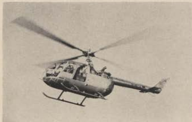
The BO-105 utility helicopter is the first larger German rotorcraft design. The two-ton helicopter features two engines and a rigid rotor. Its performance figures are exceptionally good. Boeing/Vertol has worked out an agreement to manufacture and sell the BO-105 in the US.
