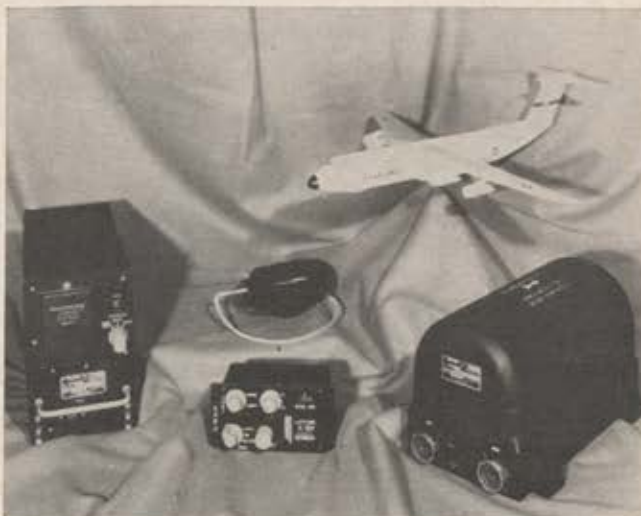
C-5 pilots and navigators are furnished a battery of novel navigation aids. Lear Siegler furnishes the two Precision Aircraft Reference Systems, components of which are above.
