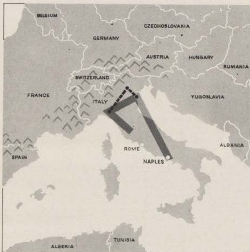
TYPICAL AREA COVERAGE OF MOVING MAP DISPLAY COMPARED WITH ROLLER MAP STRIP. 1000 x 1000 nautical miles at both scales; 1:500,000 and 1:2,000,000.
