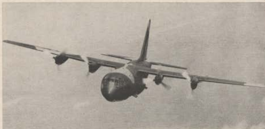
Follow-on to Vietnam veteran dragonship, AC-47, is the AC-130 gunship, which will further increase US ability to hit targets on first pass despite poor visibility. Integrated attack system effectively combines reconnaissance with strike capability.
