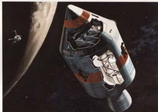
This cutaway view of the Apollo Service Module shows approximate positioning of four Beech cryogenic gas storage systems (two for liquid oxygen and two for liquid hydrogen). These will carry oxygen and hydrogen supplies for life support and electrical energy generation for a 14 day mission.
