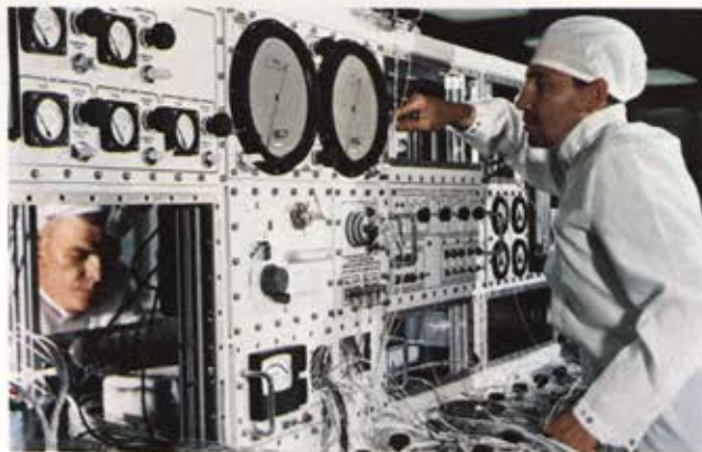
Beech also developed and built the Beech Maintenance Equipment needed to test and functionally certify Beech-built airborne systems after installation in the Apollo spacecraft.
