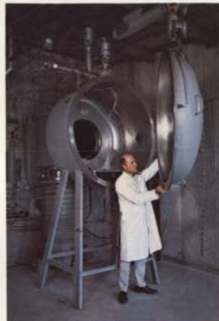
A vacuum leak detection system was especially designed by Beech to provide accurate measurement of helium or hydrogen gas leakage or permeation. Permeation levels as low as 1 \times 10^{-6} std cc per sec have been measured.
