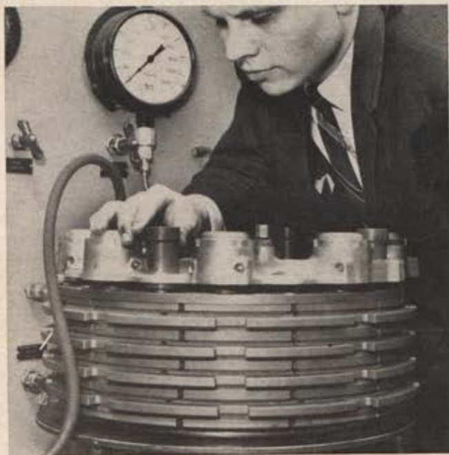
B. F. Goodrich and Lockheed achieved breakthrough in C-5's brakes by using beryllium, which cuts weight by thirty-five percent, yet is more durable than conventional material.
