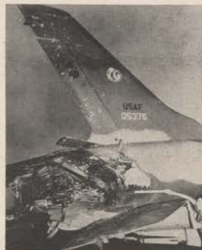
This F-105 Thunderchief picked up some enemy hardware while on a mission over North Vietnam and brought it back to base. Airman points to a missile's tail protruding from aft section. F-105s fly seventy-five percent of USAF missions over North. With new tail, this aircraft is back in action.
