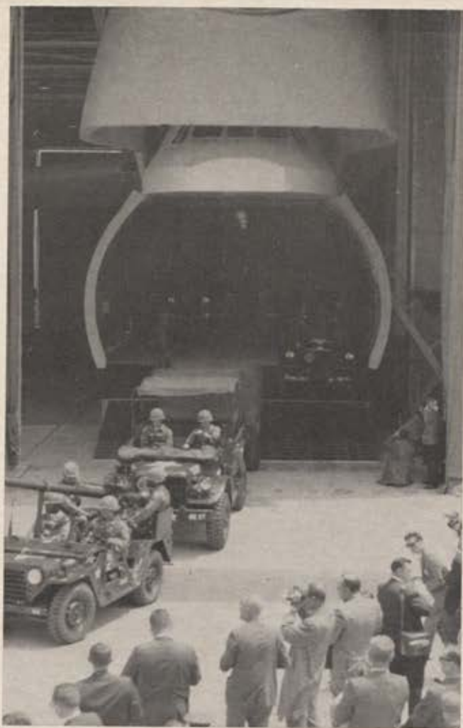
Through-loading capability of the C-5 speeds up the aircraft's ground time and reduces its vulnerability in forward areas, since offloading takes no more than fifteen minutes.
