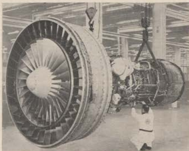
TF39's most distinguishing characteristic is the huge stage-and-a-half front fan, which measures more than eight feet in diameter and provides high bypass ratio.
