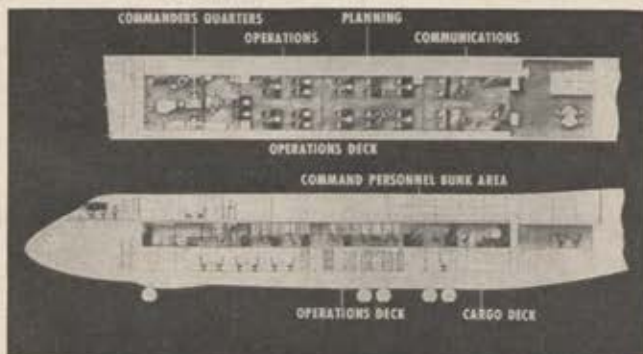
C-5's potential for use as an Airborne Command Post is most promising corollary mission currently under study. In-board profile layout shown here features three decks.
