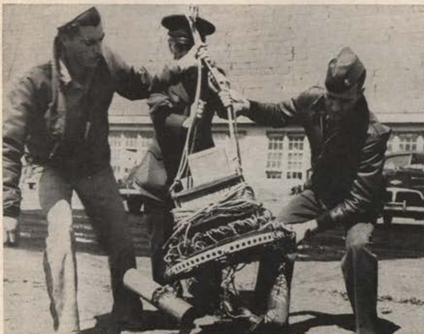
Three US servicemen hold a captured Japanese balloon bomb to show the complicated release mechanism. On the right side of the cast aluminum wheel hangs one of the sandbags which were to be dropped at preset altitudes. When all the sandbags were dropped, the balloon would discharge its load of bombs and then destroy itself with a small demolition charge.
