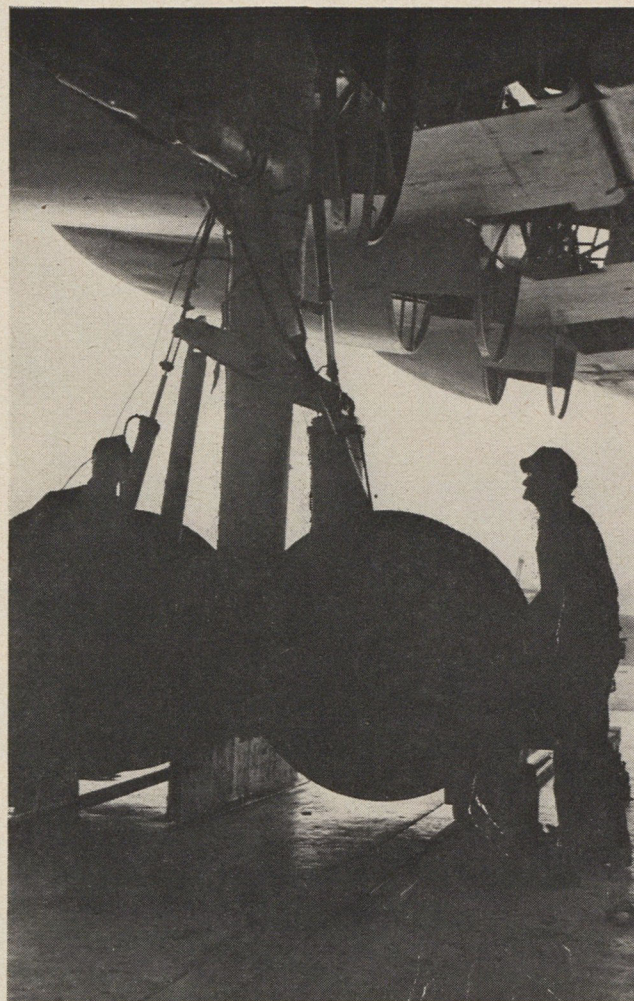
To move the 90,000 lb airframe, a hydraulic-rack is improvised from 10 oleo struts which move it in 15 ft strides.
