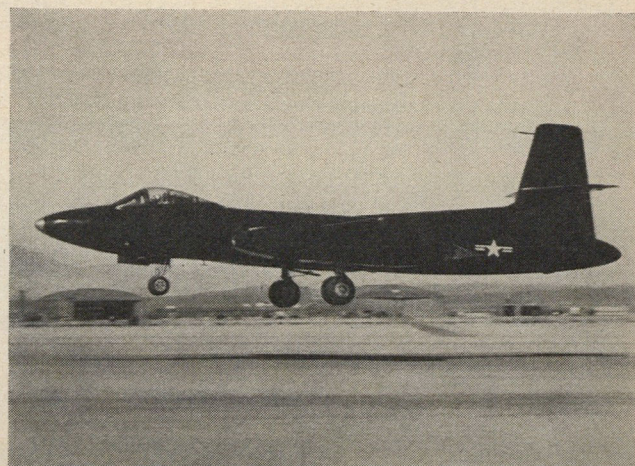
(See Most Powerful Fighter.) First take-off of Curtiss-Wright XP-87 at Muroc. Powered by four Westinghouse jets, its power is equal to electric locomotive. Plane is in 600 mph class.
