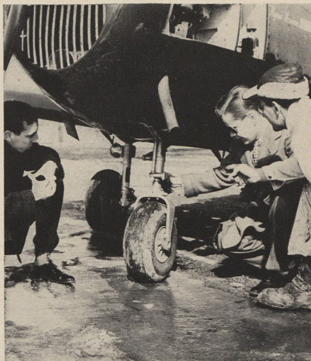
Technical check: Richard Schieler and George Parr inspect the Navion's steerable nose wheel. Arthur Kedjerski, Mallard's maintenance chief, explains the unit's operation.
