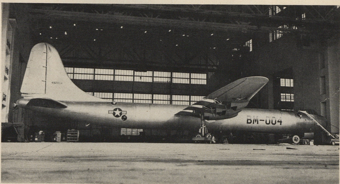
The 163-foot fuselage can just about be dollied into the static-test building at Wright Field. The 230-foot wing does better. The available depth, intended for two bombers, was 250 feet.
