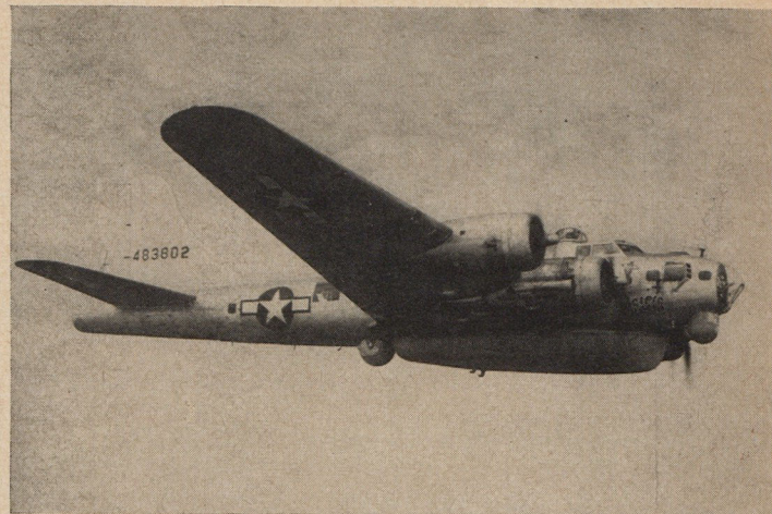
Last of regular Fortresses was the B-17H, a G modified for air-sea rescue work. It carried long-range radio, radar and chute-dropped lifeboat.
