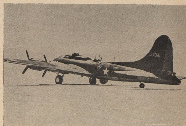
The fighter-type B-40 Fortress carried an extra turret on top, double waist guns and an almost limitless supply of fifty caliber gun ammunition.
