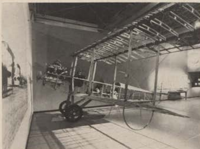
The Standard J-1 used by the Aviation Section during World War I for primary flight instruction. The airplane on display has only sample fabric covering to show wood and wire-braced construction in vogue during 1917-18 period.
