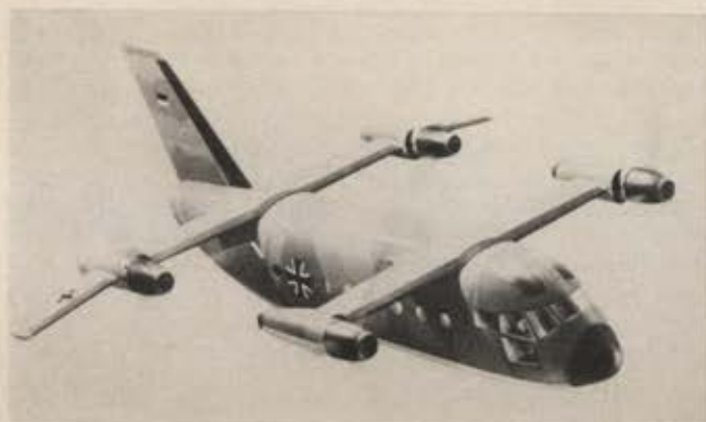
Ground tests of the VC 400 being developed by Germany's Vereinigte Flugtechnische Werke are scheduled for sometime later this year, with first flight of the four-engine, tandem, tilt-wing aircraft to be undertaken in mid-1970.
