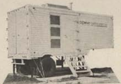
ONE OF THREE DORSEY UNITS that make up the transportable COMSAT Earth Station designed by Northrop Page Communications.
