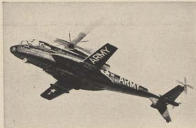
Heavy turret-mounted armament is planned for the Army/Lockheed AH-56A. In the configuration above, a 40-mm grenade launcher is in the nose and an Aeronutronics 30-mm "soft-recoil" cannon is in a 360-degree turret on the bottom of the aircraft. A multisensor sight is located between these two weapons. It will carry a laser range finder, low-light-level TV, and probably several other sensors. Other AH-56A configurations will carry 20-mm Gatling guns, and all of them have a very high ammunition capacity. It can lift the same payload as the Douglas A-1.
