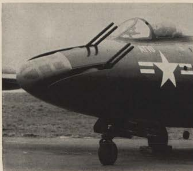
An early Navy attempt to give tactical fighters the capability to hit targets off their wing is pictured in this quadruple .50-caliber gun installation on a Grumman F9F.
