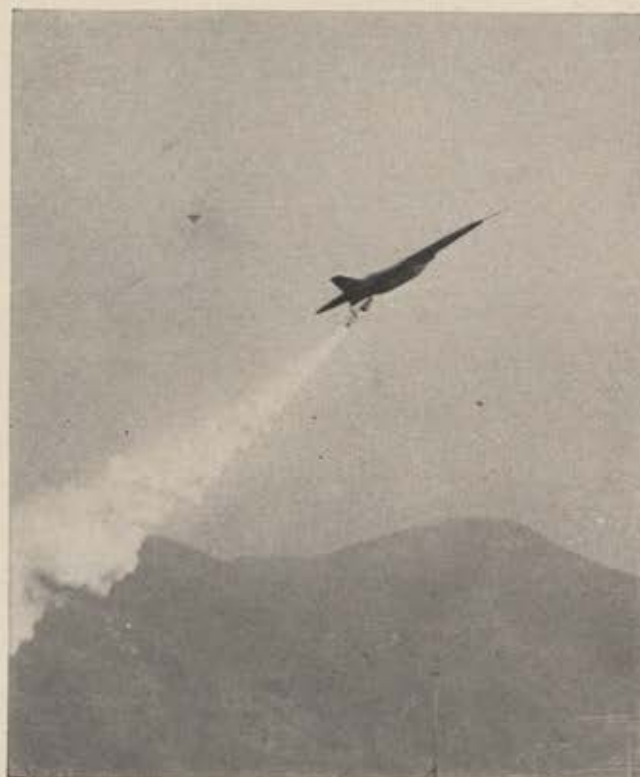
A Ryan supersonic Firebee II marks another milestone in its development as the advanced aerial jet target is launched from the Naval Missile Center, Point Mugu, Calif., with its external fuel tank in full mission configuration. Ryan is flight testing fourteen supersonic Firebee II prototypes.
