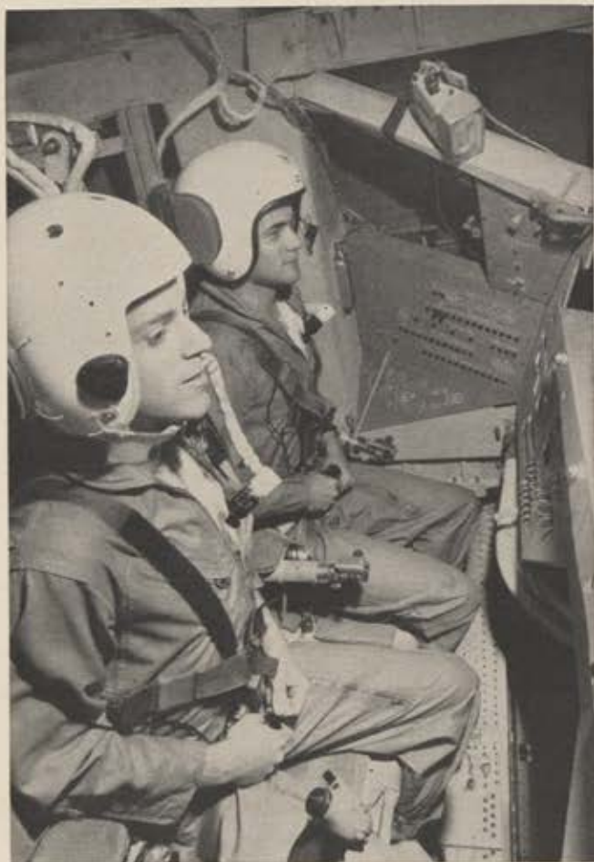
Two scientist-astronauts, Joseph Allen (left) and Brian T. O'Leary, ride an MSC centrifuge and experience forces of up to nine Gs during tests of the Apollo launch abort system, all part of MSC's lengthy preparations for Apollo flights, a main activity at Manned Spacecraft Center.
