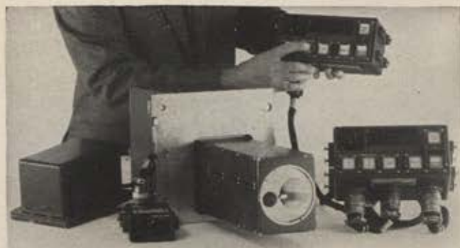
A key element in the new airborne sights is the laser range finder. This Hughes model has been ordered into production for tanks. Lasers can determine range to an accuracy of a few inches in a mile, and this precise range determination makes it possible to hit a target with the first rounds that are fired from an aircraft's weapon.
