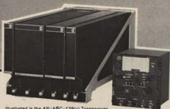
Illustrated is the AN/ARC-138(v) Transceiver utilized in airborne command and control applications.
