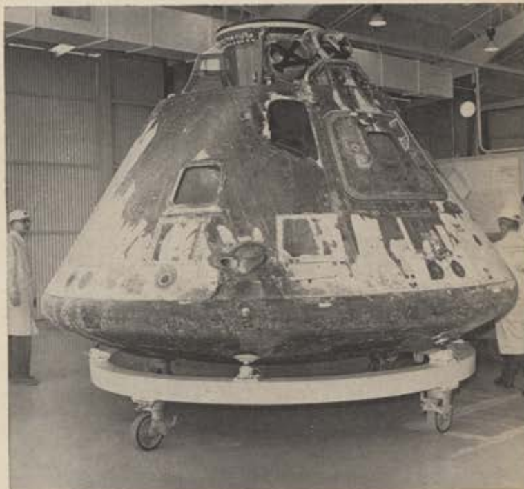
Reentry is a fiery maneuver, as can be seen from appearance of capsule. Maximum temperature on hot, leading edge of Apollo-8 spacecraft as it seared homeward through atmosphere was some 4,700° F. Hatch side was coolest.
