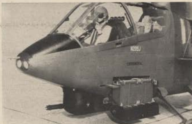
The TAT-102 chin-turret installation (above) with a 7.62-mm Gatling gun and a simple lead angle prediction sight played an important role in the renaissance of turret-mounted ground-attack systems, which is now affecting all of the military services. Emerson Electric developed the TAT-102, using company funds, and the weapon's effectiveness was proved in tests aboard the Army/Bell Huey Cobra several years ago. Much heavier guns, with laser sights, are being tested on the Cobra. Weapons as large as 105-mm and rocket-assisted ammunition are being considered.
