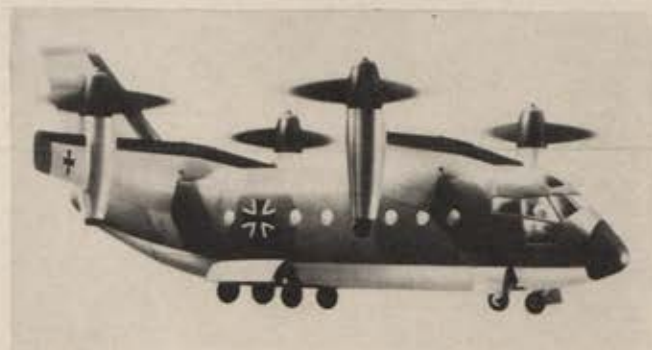
The VC 400, destined for both a military and commercial role, combines the properties of a helicopter during vertical flight with the characteristics of a high-speed turboprop transport aircraft performing a conventional flight.
