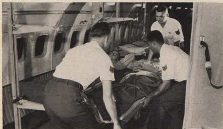
Medical Corpsmen load airman acting as litter patient aboard C-9A mockup at McDonnell Douglas plant to demonstrate working of removable stanchions that hold litters in up to four layers. Stanchions incorporate emergency masks, reading lights, ash trays, cold-air outlets, 28-volt outlets, patient call buttons, signal lights, and public-address speakers.
