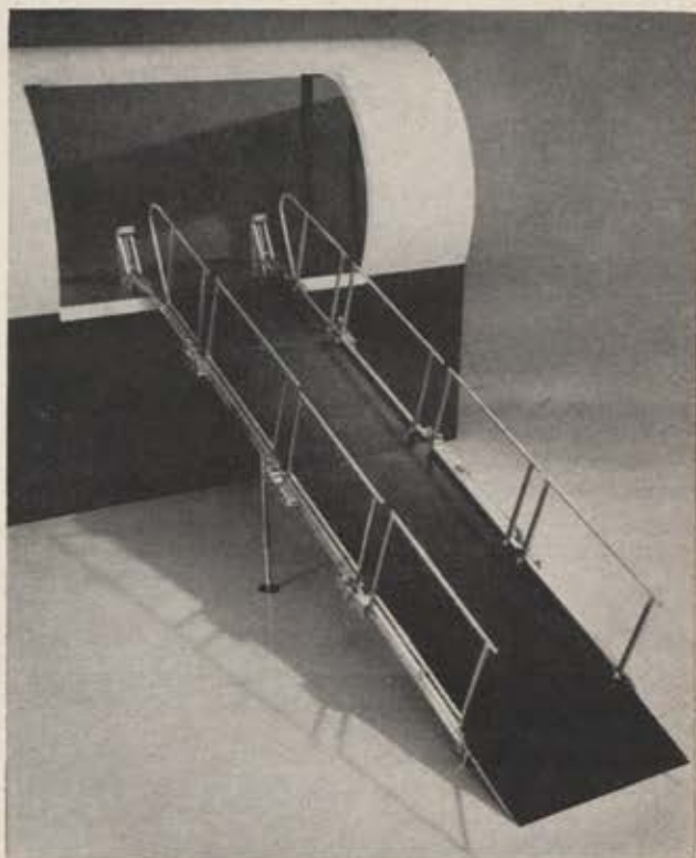
This mockup demonstrates hydraulically operated patient-loading ramp. When not in use hand rails fold down, support legs fold up, and ramp folds by sections into a compact package inside patient-loading door of the C-9A.
