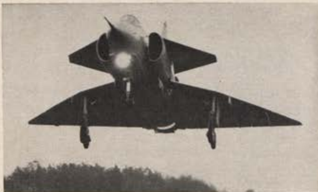
Watching a Viggen take off is a spectacular experience since, although it weighs fifteen tons, it will lift off the runway in only 1,300 feet. The STOL capability of the aircraft meets Swedish Royal Air Force dispersal requirements.
