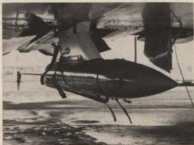
Sandpiper, USAF's new supersonic target missile, is powered by hybrid rocket, using both solid- and liquid-fuel technology. In recent firing from 49,000 feet from F-4C Phantom II, Sandpiper approached Mach 2, remained in level flight for five minutes, unusually long for any rocket.
