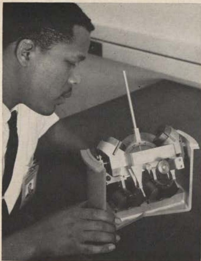
This is the heart of a satellite, a little damper that helps keep satellite in a fixed position relative to the earth. It's the core of a Philco-Ford-built Naval Research Lab satellite.
