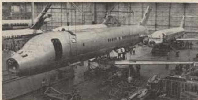
Wing and fuselage of first C-9A aeromedical transport are joined at McDonnell Douglas plant in Long Beach, Calif. The twin jet will carry up to forty litter or ambulatory patients, or both, more than 2,000 miles at some 500 mph.
