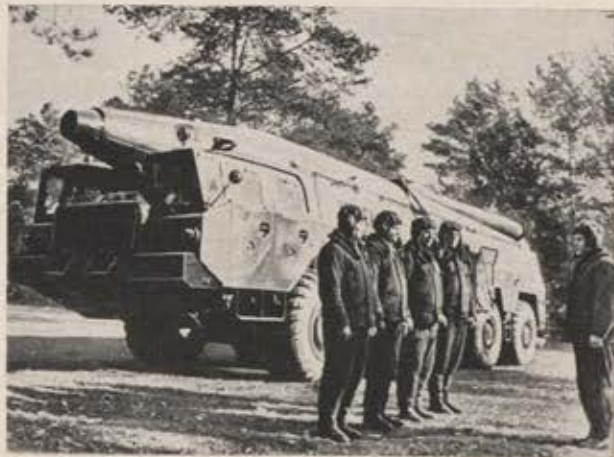
Crew of a Soviet Army mobile missile launcher stands at attention during a pause in their exercise. It is believed that this missile burns storable propellants, which are carried in an accompanying tanker-pumper truck.
