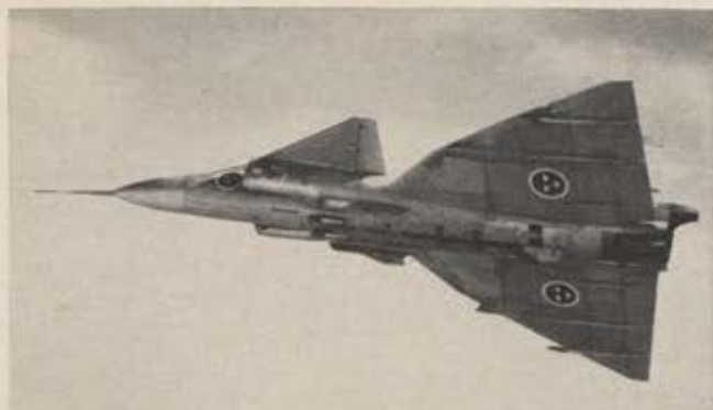
The Viggen , shown here clean, is designed to carry a wide variety of armaments. It has five permanent pylons for external stores, but additional hard points are available.
