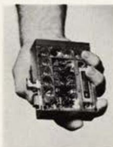
The up-link C-band receiver shows rugged state-of-the-art construction.
