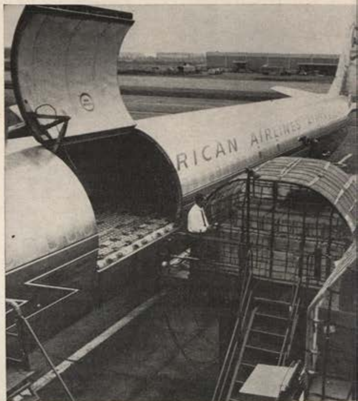
An American Airlines crew, using this special "Astroloader," can load or unload 90,000 pounds of cargo, arranged in "igloos," in twenty minutes with help of powered rollers inside 707 jet freighter. The payload is US Army materiel.
