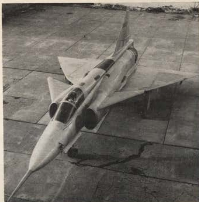
Viggen configuration makes use of wing-canard interference effect, which allows aircraft to take off and land at dispersed airfields consisting of reinforced sections of highway.
