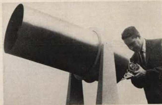
Itek lens above is considered obsolete in the optics business because it is more than five years old. It has a 20-foot focal length folded inside its 45-inch length and can photograph objects as small as one foot wide at a distance of 100 miles.
