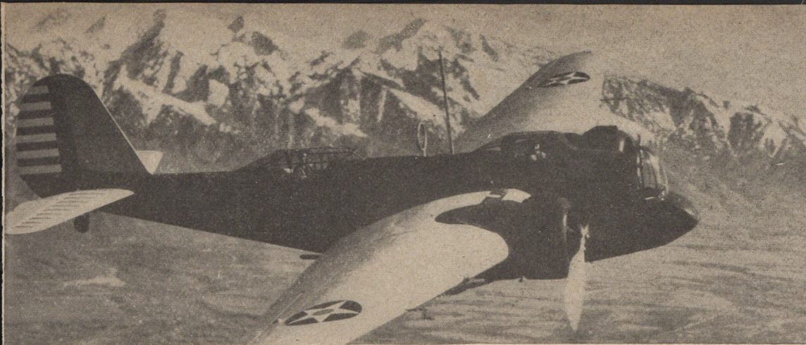
Martin built the B-10 prototype "on spec" in the depression year of 1931. Radical for its time, it contained such innovations as retractable landing gear, enclosed gun turrets, a 200 mph top speed. It altered the design trend.
