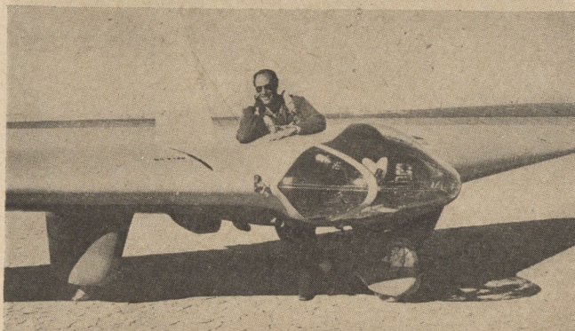
After two years, AAF released this view of test pilot Harry Crosby, standing "through" Northrop's rocket-powered prone-position all-wing fighter. Lack of a rocket engine caused change to turbos.
