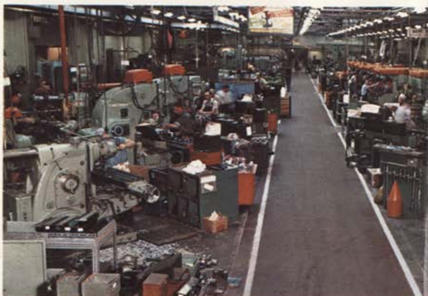
The Beech machine shops occupying nearly 60,000 square feet, are equipped with standard and special machines oriented to the aerospace industry. These include milling machines with
