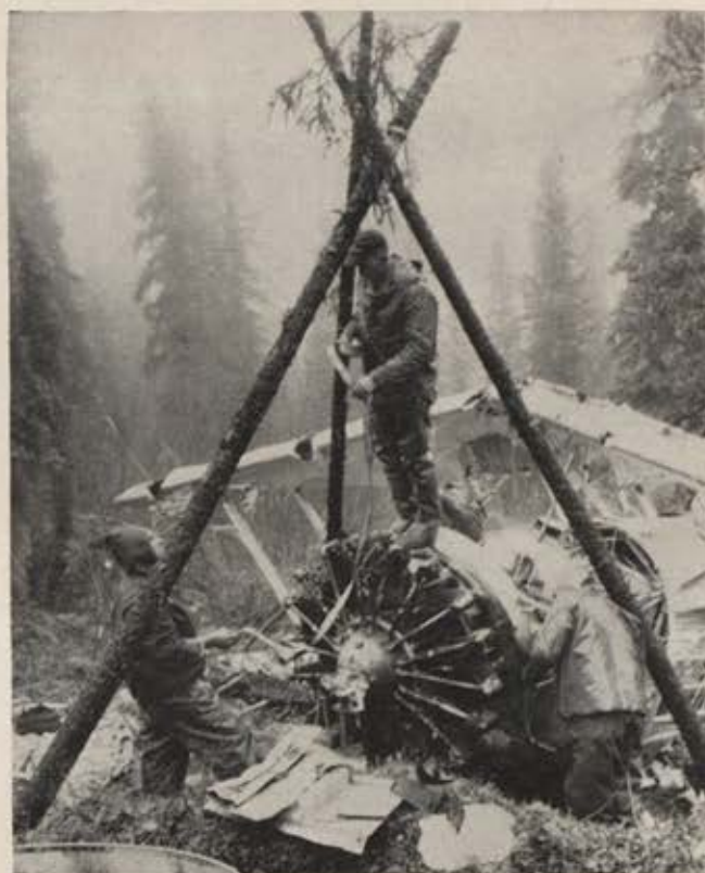
Arctic survival instructor TSgt. Robert Collins helps Sergeants Prosser and Poirier rig an "A" frame of logs to support engine when lifted from the aircraft's fuselage.
