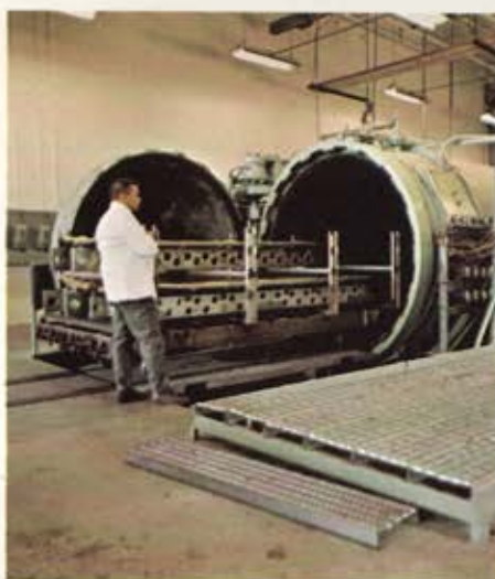
The complete bonding facilities (metal-to-metal and metal-to-honeycomb) at Beech are capable of manufacturing assemblies of metal, reinforced fiber, plastic and paper. All layup of assemblies is accomplished under "clean-room" conditions. Techniques and tools have been developed for honeycomb core shaping by machining and crushing. More than 600,000 military and commercial metal bond assemblies have been produced here.
