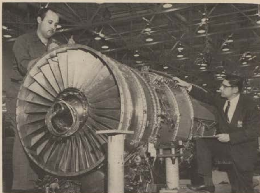
Pratt & Whitney Aircraft's JT8D turbofan in final stages of preparation for testing first-stage fan using boron/aluminum composite blades. Following installation of inlet case and guide vanes, the engine was run in a two-hour test in East Hartford, Conn., to JT8D takeoff rating thrust levels without damage. Fan is largest metal-matrix composite rotating component that has ever run.
