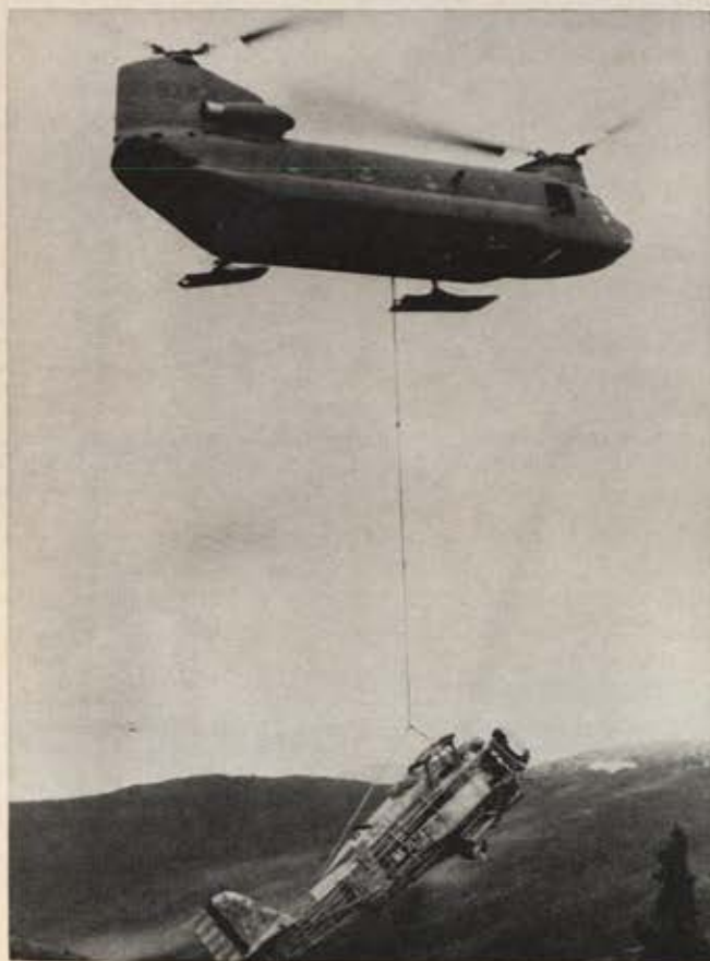
Chinook helicopter lifts out O-38 fuselage by a sling attached to the plane's original lifting cables at the four strut points. The O-38 begins its last flight, to a new home.
