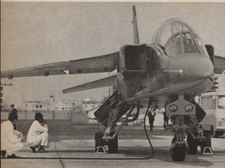
The Jaguar has been designed for easy maintenance under field conditions. Where possible, plug-in modules have been provided for replacement of electronic equipment.
