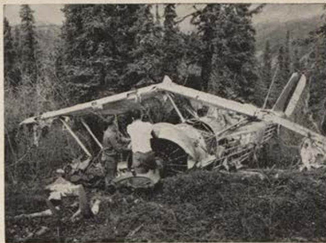
Sergeant Poirier and TSgt. Gary Prosser with crashed aircraft await the removal of a tree so that they can tilt the aircraft back and begin removing the ring cowlings.
