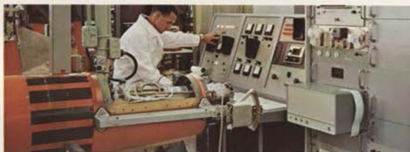
The never-ending search for highest reliability from all Beech-built products led to the design of this General Purpose Automatic Tester. It is shown here being applied to all functional areas, both electrical and mechanical, of an MQM-37A supersonic target missile produced by Beech for the U. S. Navy. The taped read-out will become a permanent record of the test, eliminating the chance of human error in reading, evaluating and recording.
