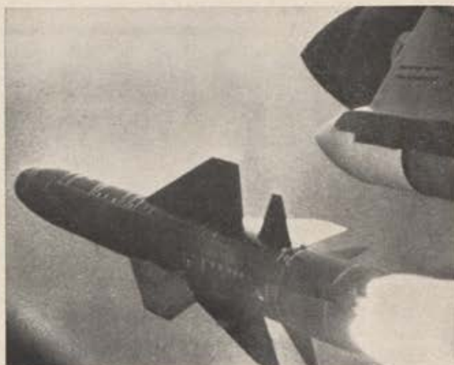
This is the first released photograph showing a launch of Martel, the Anglo-French air-to-ground missile. The bird has two versions: one that is guided to target by TV and an antiradar weapon that homes on enemy radar transmissions. Firing trials of Martel were highly successful.
