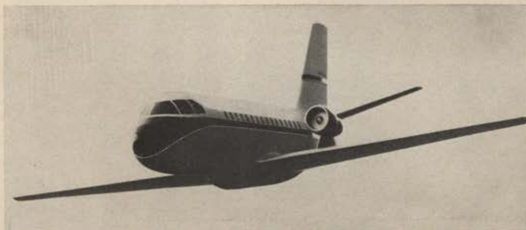
Scale model of West Germany's first postwar jet transport, the VFW 614, currently in development. Its features are to include STOL; fast turn-around; the ability to operate from roughly prepared airstrips; independence from ground power equipment; and a high utilization factor.
