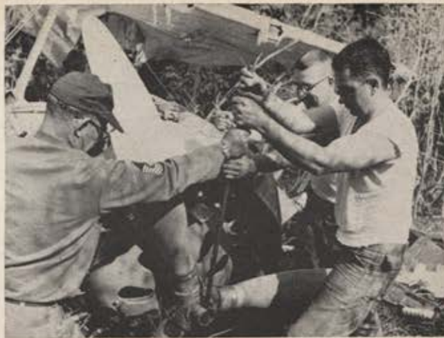
The initial task in recovery effort was removing aircraft's propeller. Sergeants Poirier, Prosser, and Marvin Mains here use bar to loosen it. The metal parts showed little rust.
