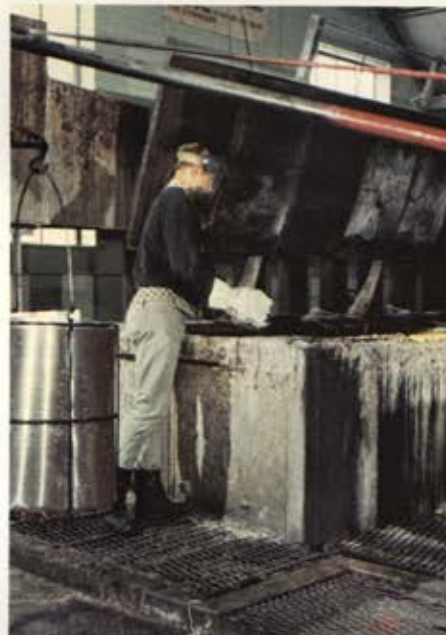
Heat-treating facilities include six aluminum heat-treat furnaces with capabilities of drop quenching and handling parts up to 9½ feet high, 8½ feet wide, and 24½ feet long. The facilities are furnished with aging furnaces having inside dimensions up to 8 feet wide, 6 feet high and 40 feet long.
