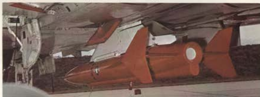
Sandpiper, the first maneuverable rocket-powered supersonic target missile has successfully completed first tests for the U. S. Air Force. The test vehicle was a modified Beech AQM-37A missile powered by the nation's first operationally-designed hybrid rocket engine. The engine, developed and produced by United Technology Center, uses both solid and liquid fuels and has sustained flight of Sandpiper during tests for an extraordinary full five minutes.
