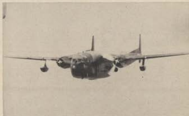
First AC-119, gunship version of the Flying Boxcar, arrives for duty in South Vietnam. Recalled from AF Reserve status, the vintage aircraft have been outfitted with four 7.62-mm Miniguns. Plans call for the gunships to augment the mission performed up to now by the AC-47 Spookies.
