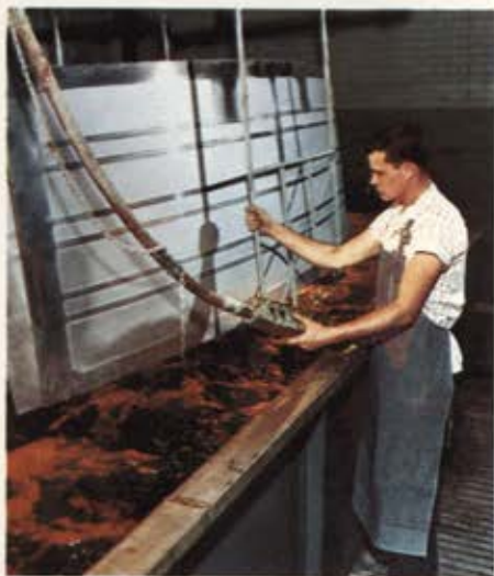
Chemical Milling for precision milling of aerospace metals (aluminum, magnesium, titanium, inconel, steel and stainless steel) to unconventional design specifications has developed to extensive capability at Beech. Among the largest in the U.S., 167,340 parts were produced here in 1967. Facilities include cleaning, rinsing and washing equipment. The tanks, in sizes up to 14 feet long and 14 feet deep, are equipped with automatically timed taper hoists.
