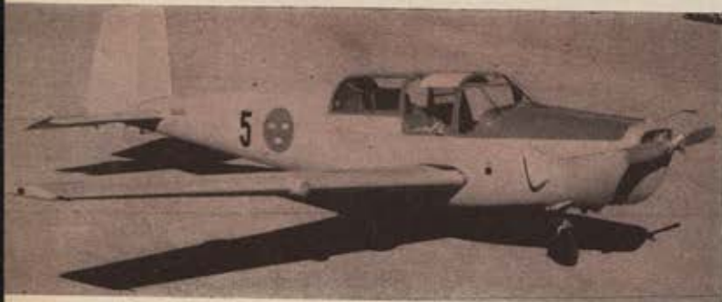
The Sk-50 Safir , whose top speed is 170 mph and range is 680 miles, is used for basic flight training. A Dutch factory now makes Sk-50s under sub-contract from SAAB.
