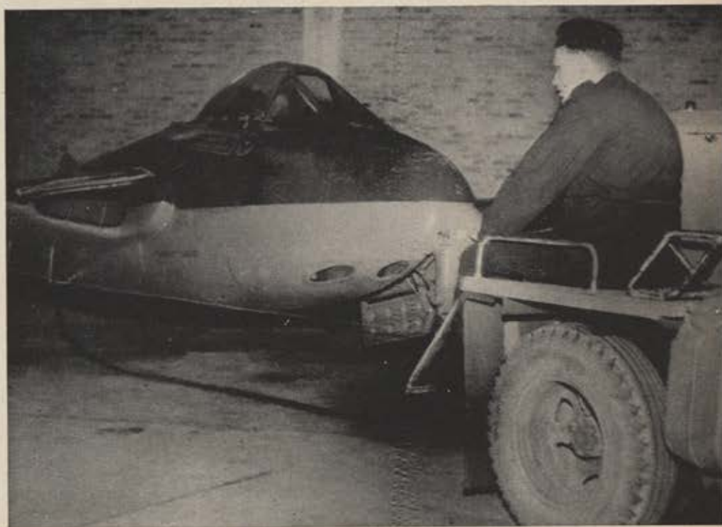
In one of the Swedish Air Force's underground rock shelters, a J-28 Vampire trainer is attached to a jeep which will tow it out to the starting runway.
