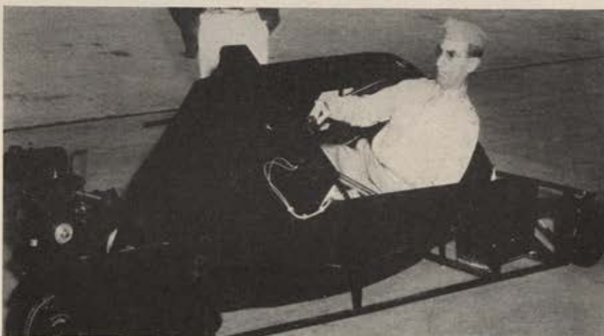
Colonel Ocker checks out in one of his own training devices—the Ocker Training Buggy, which was used in preflight to test the reflexes of flyers.
