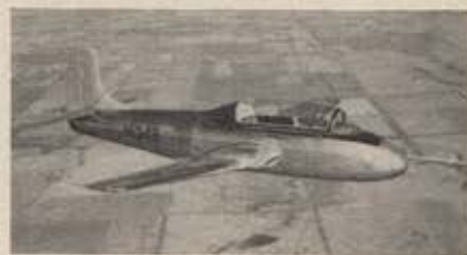
Beechcraft's Model 73 jet trainer during its first flight. The 290-mph tandem-seat two-place jet is powered by a Continental J69-T-9 turbojet engine.
