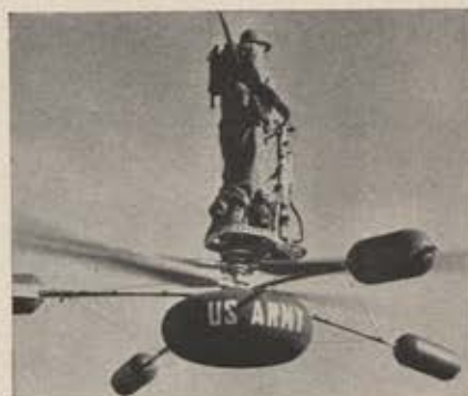
The Army has bought twelve DeLackner Helicopter, Inc. Aeroceles for tactical testing. Powered by a 44-hp engine, it will fly at a top speed of 65 mph.
