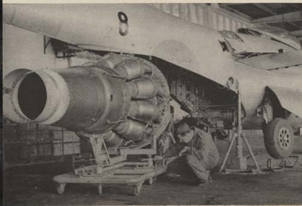
A 5,000-pound-thrust Ghost engine is readied for installation by mechanics.
