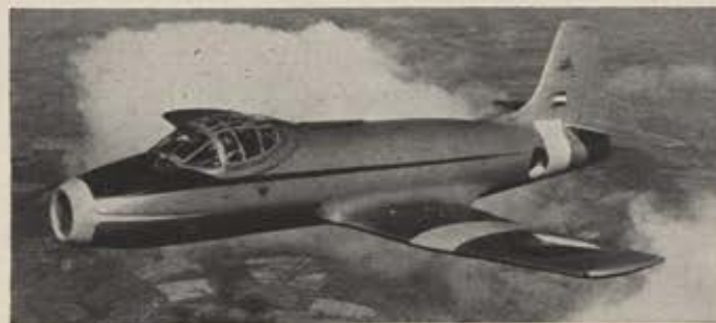
Fokker S-14 two-place intermediate jet trainer. Powered by a Rolls-Royce "8" Derwent engine, it is in 450-mph class.
