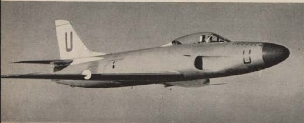
One of the better new planes now rolling off Swedish production lines is the SAAB-32 Lansen , in the same class with our Lockheed F-94C Starfire. Its Swedish-built RM-5 engine and afterburner give it speeds "well over 700 mph."
