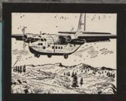
The Fairchild C-123 was especially designed for landings and take-offs on rough, unprepared fields.
