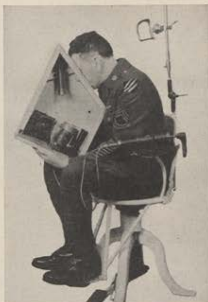
A cutaway view of the Ocker box. A hand pump is attached to the chair.
