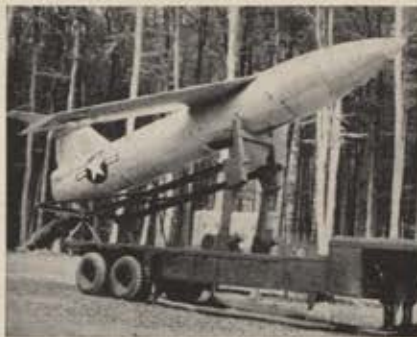
A TM-61 Martin Matador is raised into position at a First Tactical Missile Squadron launching site in Germany.
