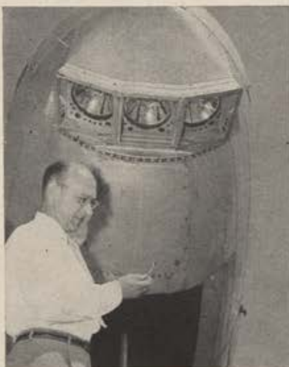
John W. Beatty, an engineer at the ARDC's Wright Air Development center, holds the tiny bulb used in mercury arc lamp photo illumination system.
