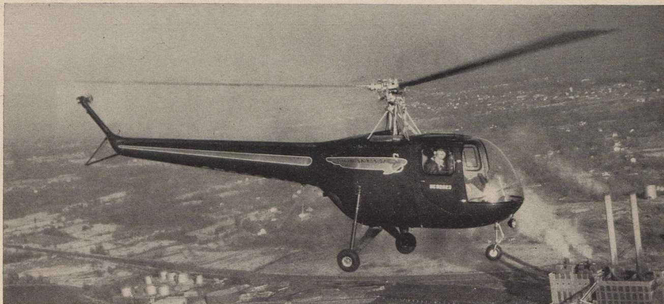
Sikorsky's new two-place S-52 helicopter, recently approved by CAA, features all-metal rotor blades.
