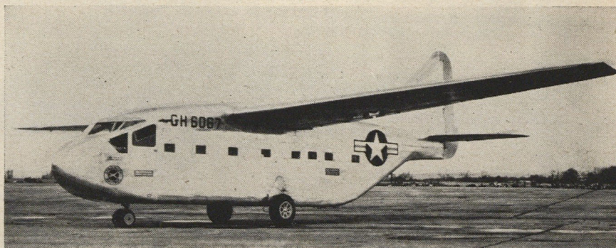
The Chase Avitrucc, the XCG-18A, is the world's first all-metal assault glider. It has an 86-foot span and is 53 feet long and has a gross weight loaded of over seven tons. The new Avitrucc is twice the size of the famed wartime invasion glider.
