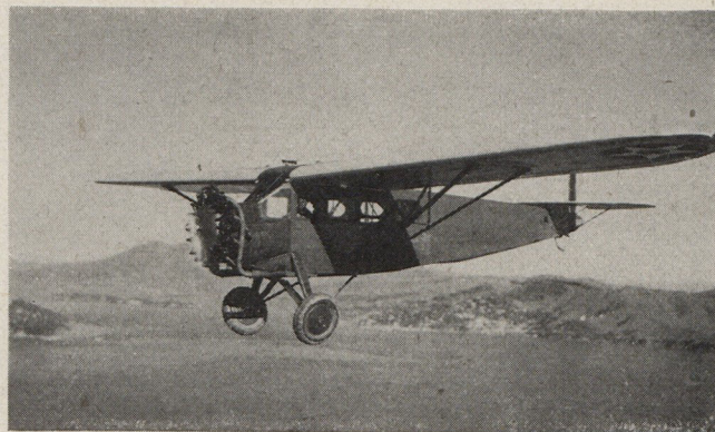
AAF's first photoplane was the F-1, a commercially built Wasp-engined Fairchild 71. It was used chiefly for making mosaic maps.
