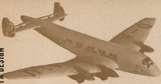
Sweepback on Germany's prewar Diesel-engined Junkers Ju 89 gave directional stability, the original use for that wing configuration.
