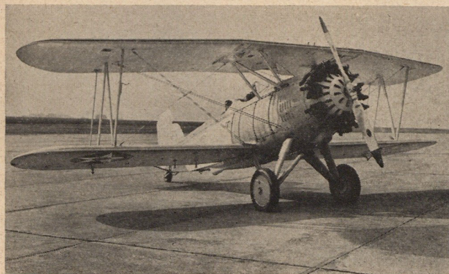
When original tests were conducted on dive-bombing, directional stability was important for accuracy. For that reason, sweepback was incorporated into the original Curtiss Helldiver, the O2C-1. This function differed from its later application for supersonic flight.
