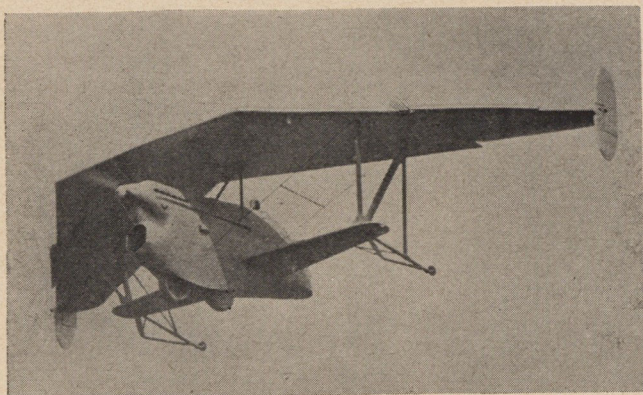
England's pioneer tailless, the Westland-Hill Pterodactyl. Deep sweepback was used to get the elevators a greater distance behind the engine and weight mass. Like the supersonic Delta-wings, slots were needed to prevent low-speed tip-stall in this craft.
