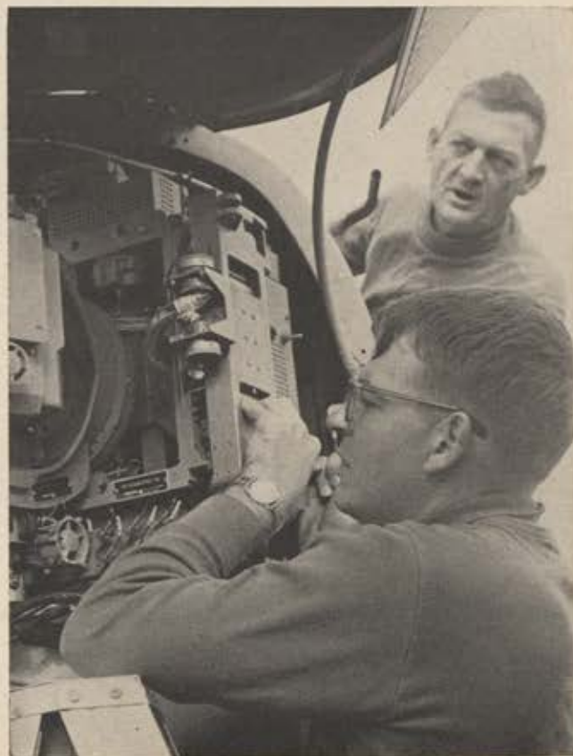
Sergeant Groover teams up with Navy radarman to repair APQ-116 radar, part of A-7's electronic gear.
