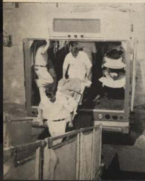
The C-9As are equipped with twenty-four-foot hydraulically operated ramps to permit litter or wheelchair patients easier boarding and unloading. Ambulatory patients board via a forward stairway or ventral stairway under the tail.
