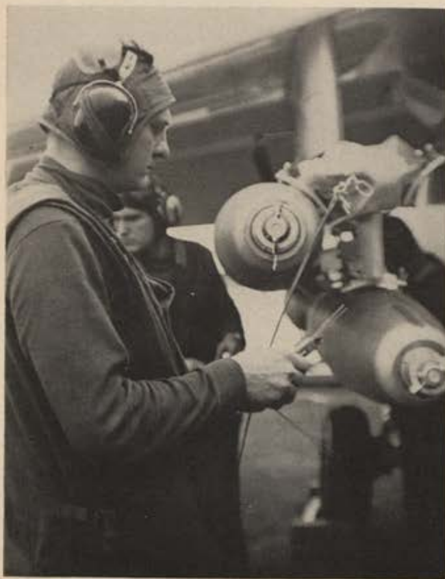
Navy ordnance men fuze a load of MK-82 (500-lb.) bombs on an A-7, in preparation for an armed reconnaissance to be flown by one of Air Force pilots.
