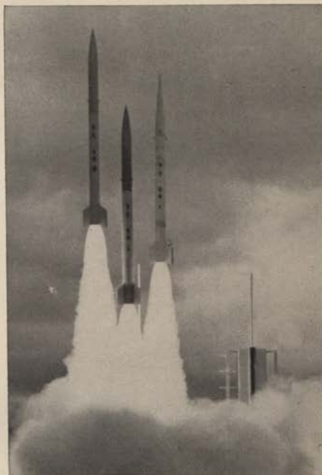
In biservice cooperative effort, this trio of Javelin III sounding rockets was recently launched in salvo at US Army's White Sands, N. M., Missile Range, by USAF crew from Holloman AFB, N. M. Trajectories of the rockets were varied.
