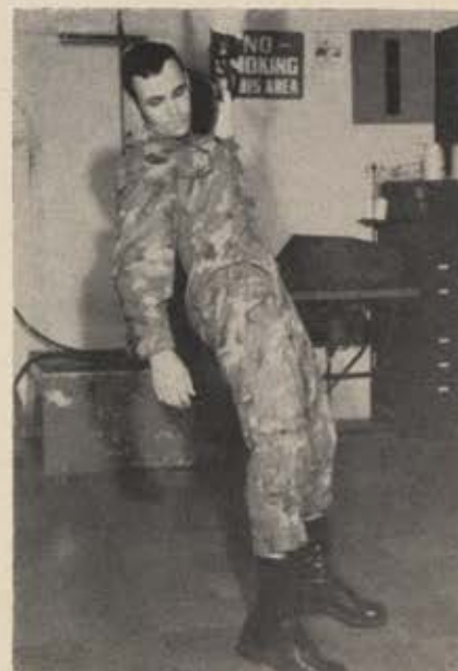
To standardize devices to rescue downed airmen, Aeronautical Systems Division, Wright-Patterson AFB, Ohio, is testing a rig of nylon tape sewn into AF flight suit with a loop on the chest that attaches to helicopter recovery cable.
