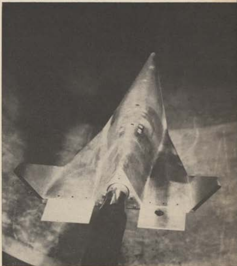
This scaled hypervelocity vehicle configuration is being tested in a wind tunnel at 20 times the speed of sound by Lockheed designers for USAF's Flight Dynamics Laboratory.
