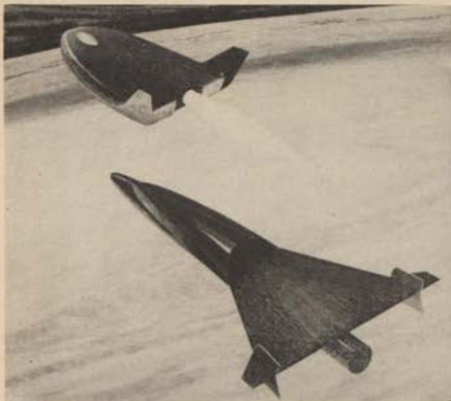
This Lockheed-California Co. artist's conception of a reusable aerospace transport shows two reusable stages, one performing boost and the other all orbiting functions.
