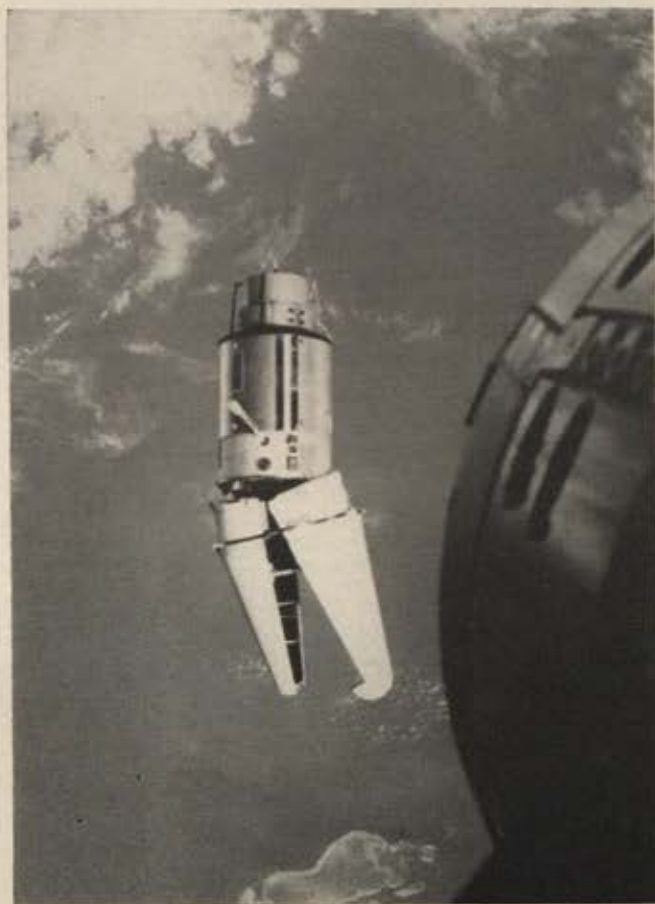
Upper rocket stages, such as this Agena with malfunctioning nose shroud, have been used in successful station-keeping experiments. Astronauts tracked them with the aid of flashing lights and could maneuver near them with precision.
