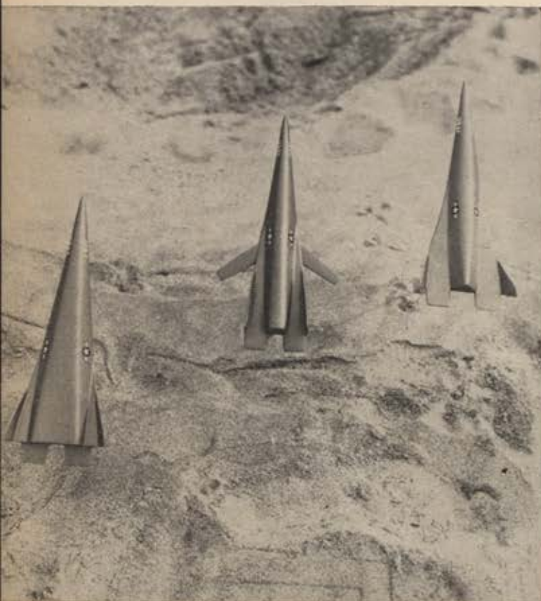
Lockheed-California Co. has studied various configurations of reusable air- and spacecraft for USAF's Flight Dynamics Laboratory, including arrowhead-shaped models shown here.
