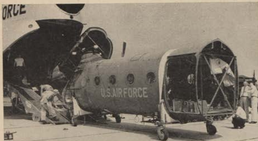
Half of a Piasecki H-21 helicopter is loaded aboard a Douglas C-124 Globemaster. At destination, it will be reassembled for flight by ground crew.
