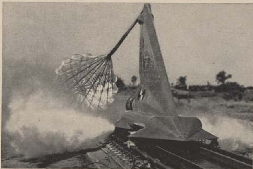
The Cook research parachute test sled throws up a cloud of spray as it hits the water brake on the High Speed Track. Rocket-powered sleds top 10,000 mph.
