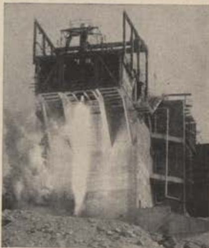
Before they're installed in aircraft or missiles, rocket engines are run in this test stand, which is built on a cliff to permit vertical firing on either side of a control room.
