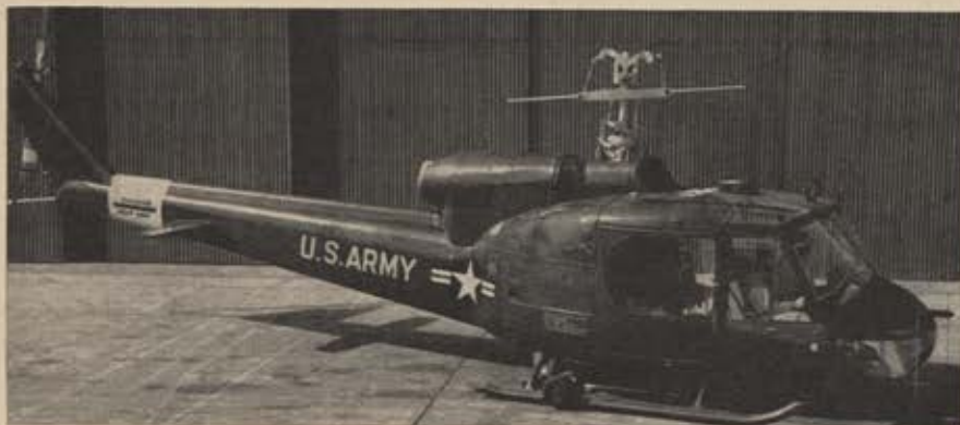
At Fort Worth, mock-up of new Bell 'copter (minus rotors) shows the XH-40's low silhouette. The Army plane will have a Lycoming XT-53 turbine engine.
