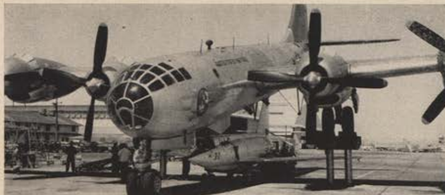
A B-29 crouches over the rocket-powered Bell X-2 like a mother hen over a chick. The giant Boeing bomber will carry the test ship aloft for launching.
