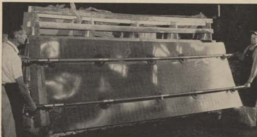
In new material-handling process in use at Convair's Fort Worth plant, vacuum cups and overhead vacuum lifts move aluminum sheet stock safely.
