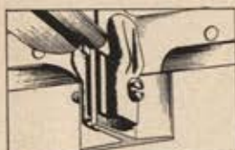
T-POSTS PUNCHED ON 1 1/2" CENTERS
