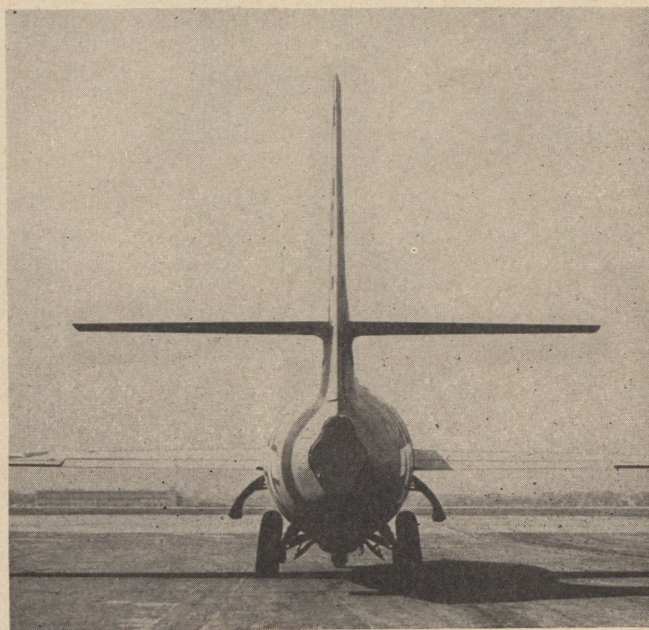
The high tail is required to lift the control surfaces out of the burning zone. Despite the unique task assigned to the Bell XS-1, its general wing pattern and configuration is quite conventional.
