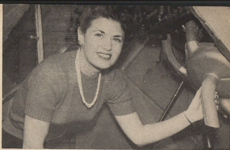
Aviatrix Betty Hughes shows the exhaust of the new Ryan muffler system for 65-85 hp engines, which reduces exhaust noises 90%. Like the setup in the Stinson Station Wagon, below, right, it also provides cabin and carburetor heat. Controllable pitch propellers, like the Beech electric, allow operation at a minimum rpm thus reducing noise-producing propeller tip speeds. Blade shapes can also help.
