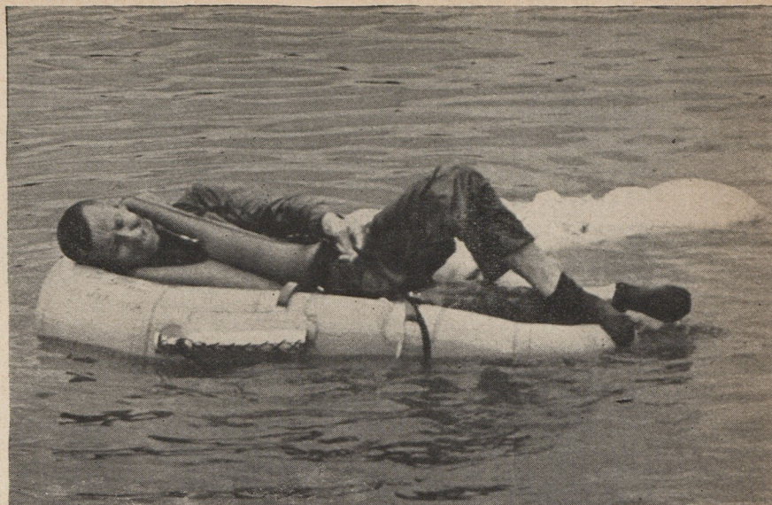
Inflated by a pressure cylinder such a collapsible craft will easily support the weight of a large man. Oars, sail, rudder and radio come with the raft, making an ideal kit for a fisherman, and it can weather high seas.
