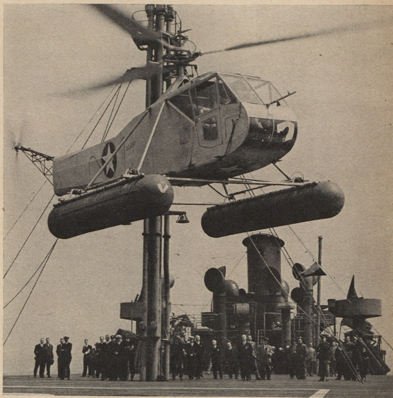
The potentialities of the helicopter were exploited by the AAF. Shown here is one of the vertical craft equipped with pontoons, ready for air-sea rescue missions.
