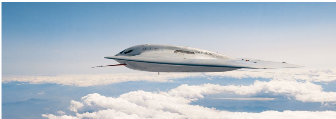
The B-21 Raider, America's newest stealth aircraft, features a refined shape, more durable radar-absorbant coatings, and other advances intended to further the science of low-observability.
