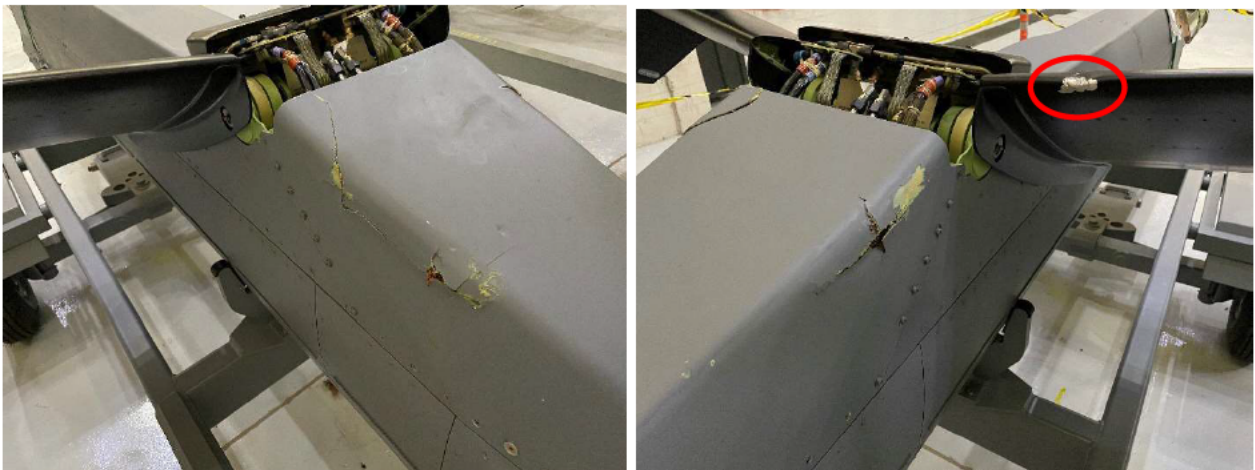
Figure 5: Close up of ARB Fairing and Elevator Damage (Tabs Z-7, Z-8)
