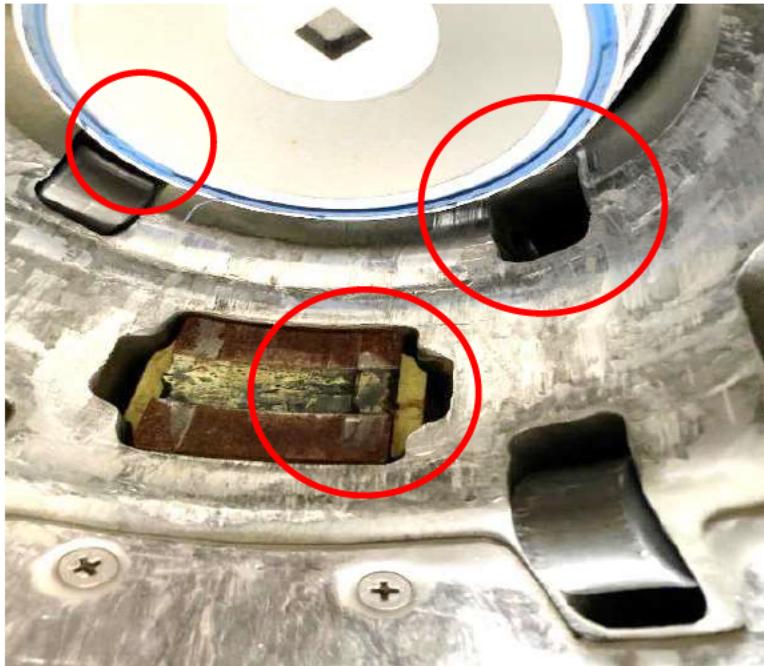
Figure 12: MA2 IFR Bucket Damage (Tab D-85)
