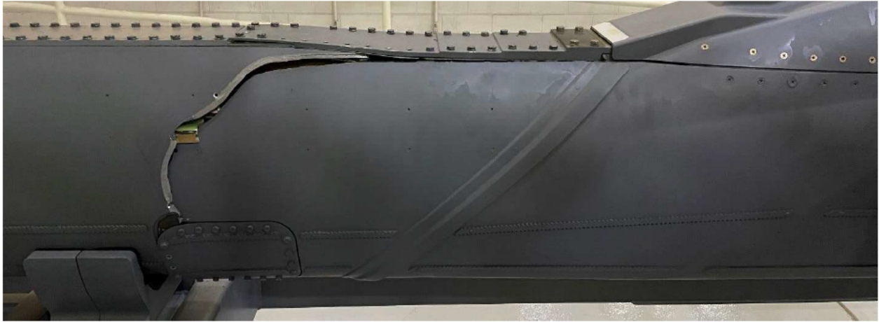
Figure 4: Close up of ARB Fairing Damage (Tab Z-6)
