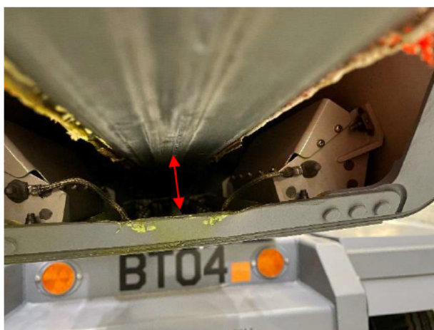
Figure 8: Close up of the Bottom Edge of the ARB Ice Shield Damage (Tab Z-10)
