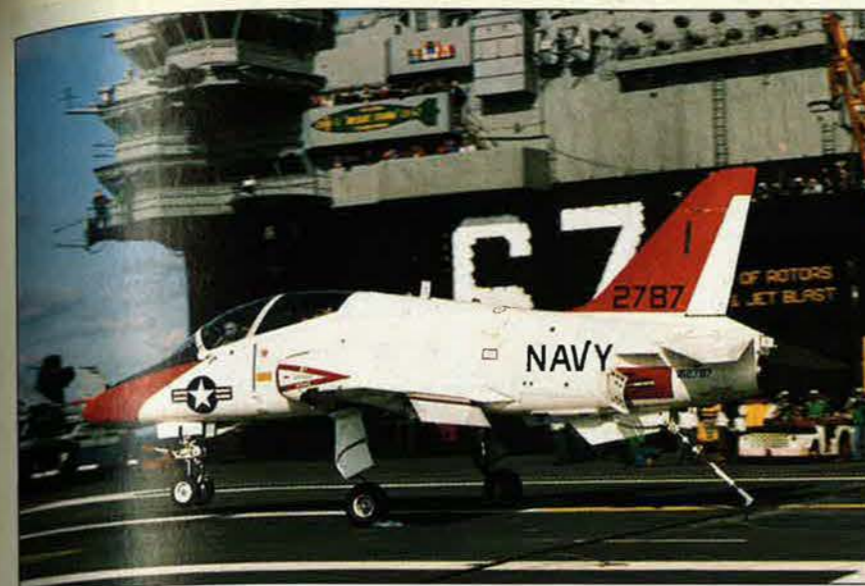
The Navy's T-45 training system began sea trials in December, successfully landing and taking off from USS John F. Kennedy. The Goshawk demonstrated all aspects of carrier suitability, logging thirty-three catapult launches and thirty-three arrested landings, with a total of 12.1 hours during six flight periods.
