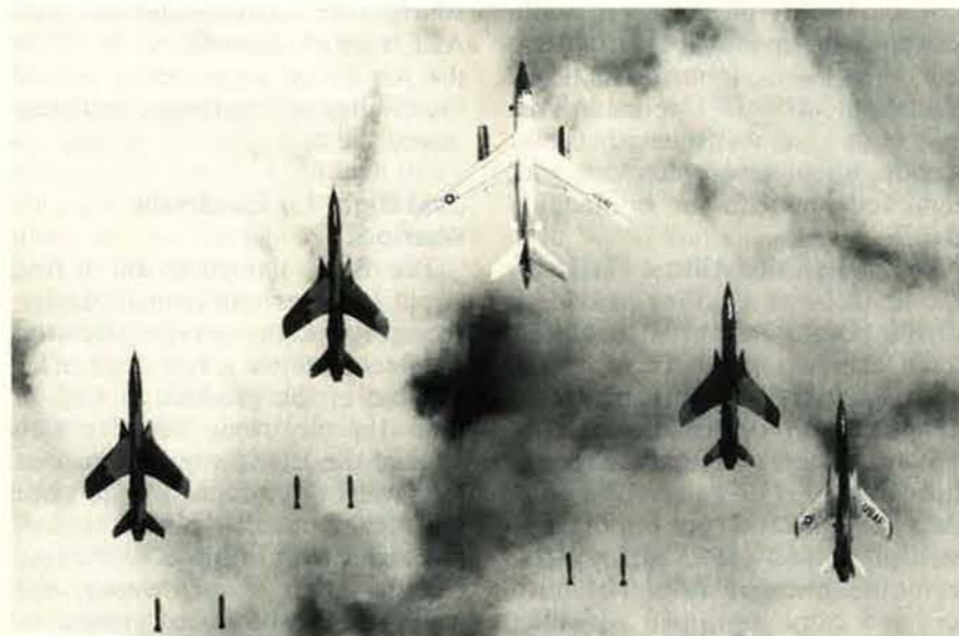
In the Vietnam War, the EB-66 performed standoff jamming and ECM escort for US strike aircraft. Here, an EB-66 guides a close formation of F-105 Thunderchiefs through clouds on a precision bombing mission while tuning in to North Vietnamese ground and airborne radar, ready to warn of a possible attack.
