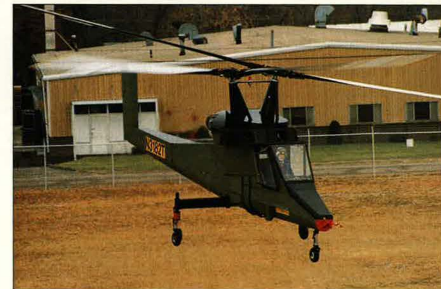
In December, Kaman Corp. first flew its new multimission intermeshing rotor aircraft (MMIRA) technology demonstrator. Its two contrarotating rotors provide increased payload capacity and endurance compared to other currently fielded helicopters. Mission applications include surveillance, resupply, and ordnance delivery.
