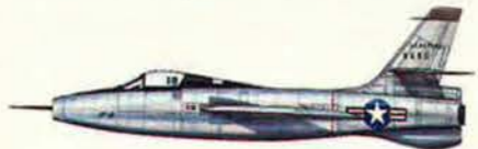
1949 The Republic XF-91 Thunderceptor used 4 rocket motors to pass the "century mark"—1000 mph.
