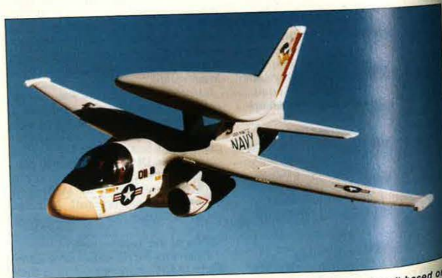
Lockheed and LTV are developing a proposal for an early warning aircraft based on the Navy's proven S-3 Viking, originally built in the 1970s. The proposal will include an electronically scanned phased-array radar, housed atop the fuselage, which would provide a full 360-degree view of the surrounding airspace.
