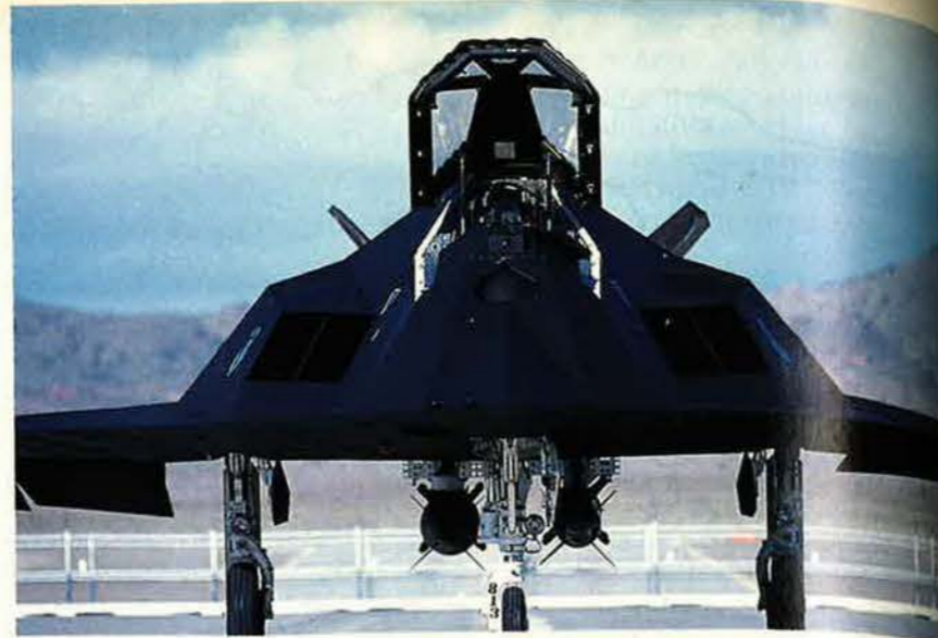
The GBU-27, a penetrating 2,000-pound weapon carried only by F-117s during the Gulf War, provided a deadly complement to the Stealth fighter. F-117 pilots sought to put the bombs "in the basket," using laser guidance to hit not just specific buildings but specific sections of those buildings.
