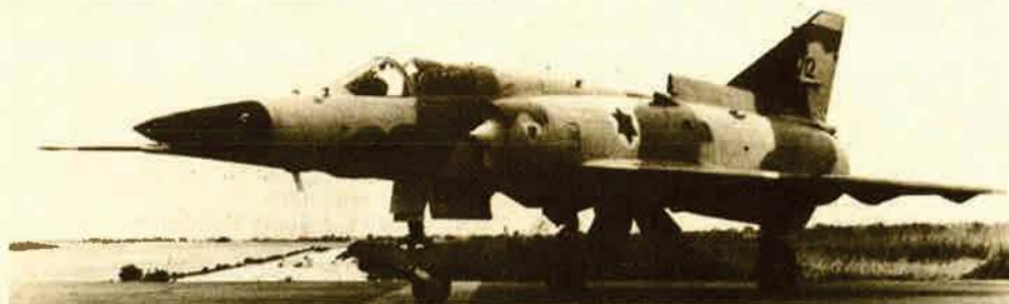
To counter possible arms embargoes, Israel built the Kfir fighter-bomber. Looking much like a Mirage V , it uses US-supplied J76 engines.
