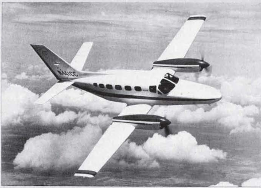
Cessna Model 441 eight/ten-seat pressurised executive transport (two 620 shp Garrett-AiResearch TPE 331-8-401 turboprop engines)
