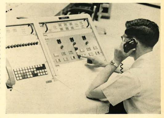
From this panel, the Command Destruct Transmitter Controller can select a destruct transmitting site from a series of sites located throughout the Western Test Range. This ensures that the missile is in range of the destruct signal through its entire boost phase. If the bird becomes a hazard to life or property, it is the MFSO's responsibility to hit the destruct switch.
