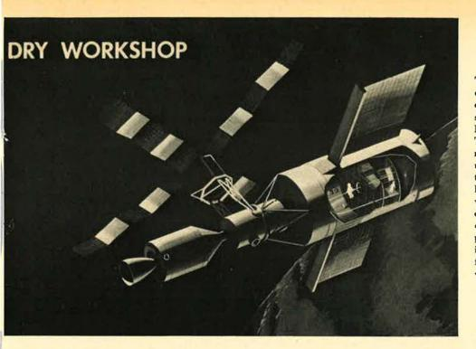
This is an artist's conception of the components of the NASA "workshop" space station planned by NASA for 1972 launching. The "dry" designation refers to the fact that under an earlier plan the workshop was to have been a booster stage that would have been sent up carrying fuel and then emptied out. The present plan allows launching of the empty lab, ready for occupancy by rendezvousing crews.
