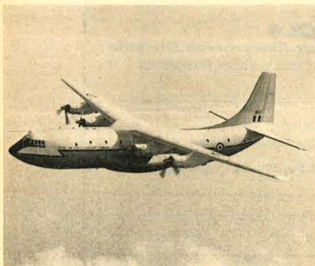
The RAF Belfast has been instrumental in several successful phases of a program to assess the blind-landing capabilities of an autoland system built by Smiths Aviation. The system has been proved so safe in tests that the RAF has authorized its use as a standard landing procedure.
