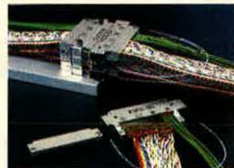
ABC connectors can be stacked, while accessibility is maintained to each plug shell for easy removal of the module.
