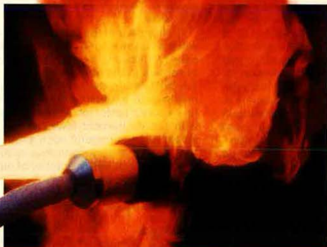
Even after being subjected to a 2,000°F flame, this DG123 connector demonstrated no loss of electrical continuity and did not support combustion.
