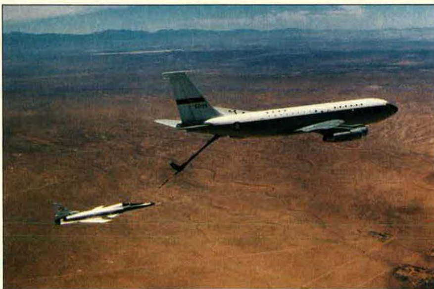
The experimental Grumman X-29 forward-swept wing demonstrator flew its 200th mission on June 8, setting a record for most flights of a single X-series aircraft. NASA test pilot Rogers Smith crewed the flight, which included this simulated aerial refueling to evaluate handling qualities.
