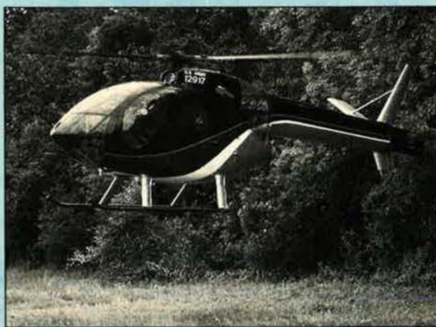
The McDonnell Douglas NOTAR helicopter can back its boom into the trees without fear of catastrophe.
