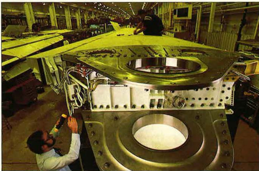
A triple-redundant wing-sealing process has eliminated many of the leaks that plagued some early production B-1B bombers. Here, Avco Aerostructures-Textron technicians do precision work on wingsets, which are reamed to a tolerance of two-thousandths of an inch to ensure exact matchup with fuselage during final assembly.
