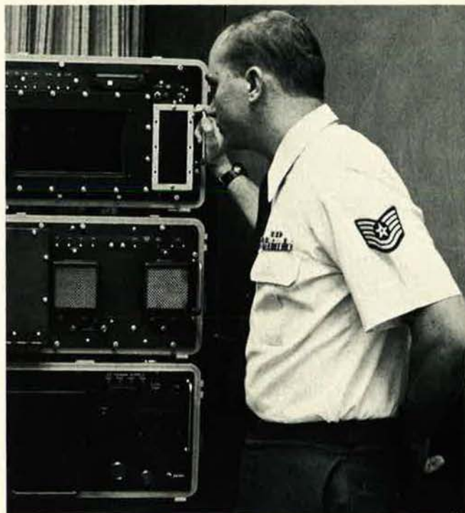
The portable Mobile Electronic Test Set (METS) is an interim solution to the AIS stations, which must be moved by forklift. The METS doesn't require strict environmental controls and is far more reliable than the AIS, and the newer equipment provides better support than equipment used previously.
