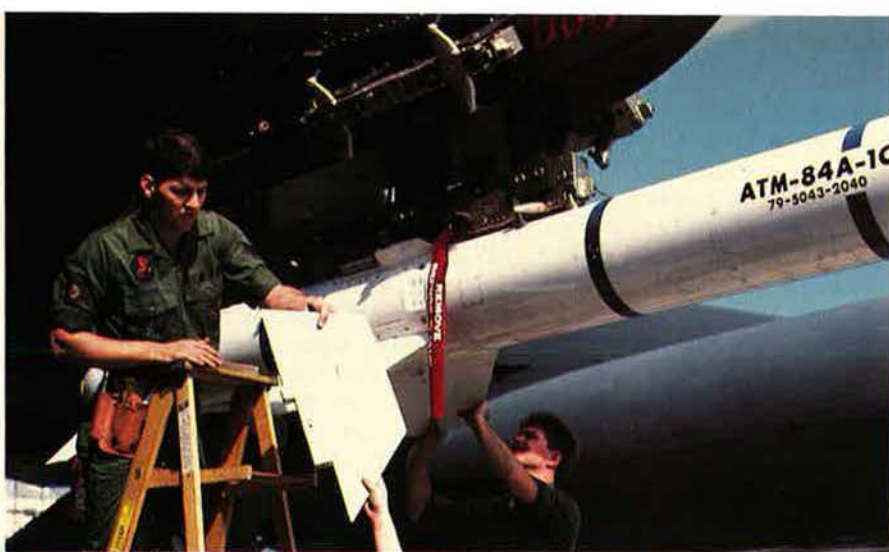
Once the Harpoon is mounted on the heavy stores adapter beam, the missile's fins are attached, which is what load crew team chief SSgt. John Osborne is doing here. Because the missile is liquid-fueled, both the Harpoon and the load equipment must be electrically grounded during loading.
