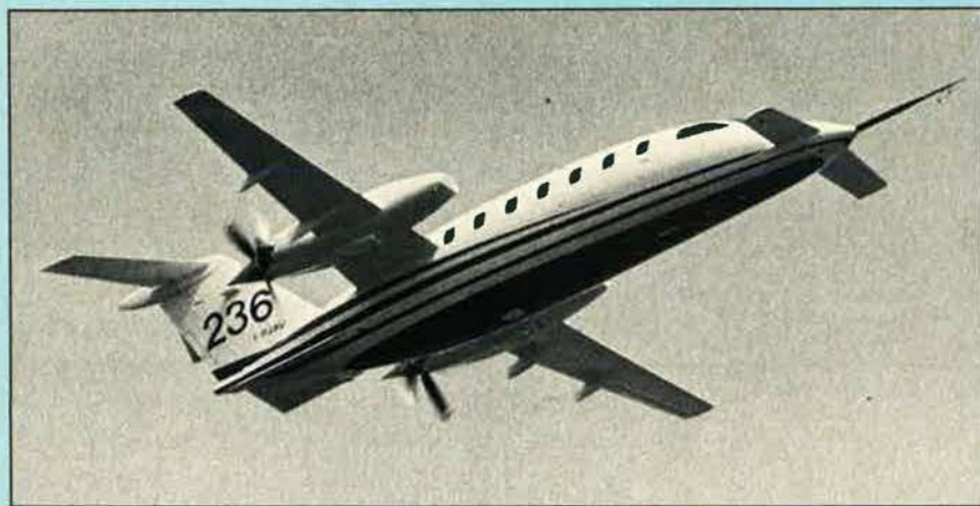
The 'three lifting surfaces' concept of the Piaggio P180 Avanti is illustrated clearly in this view (Brian M. Service)
