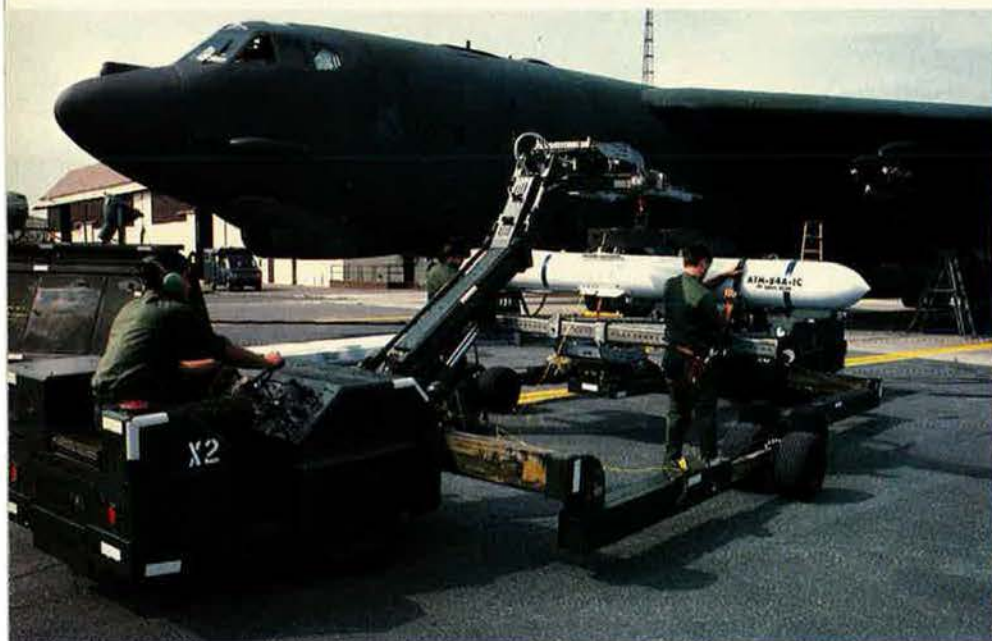
Loading the Harpoons onto the B-52 takes up to twenty-five minutes per missile. After being removed from its casket with a forklift, the Harpoon is transferred to the "jammer" and put on the airplane. Shown in this picture is one of the 42d Munitions Maintenance Squadron's seven load crews. This one includes A1C Jeffrey Andrews, Amn. Peggy Jo Therrien, A1C Joseph Dobel, and A1C Matthew Giacobbe.
