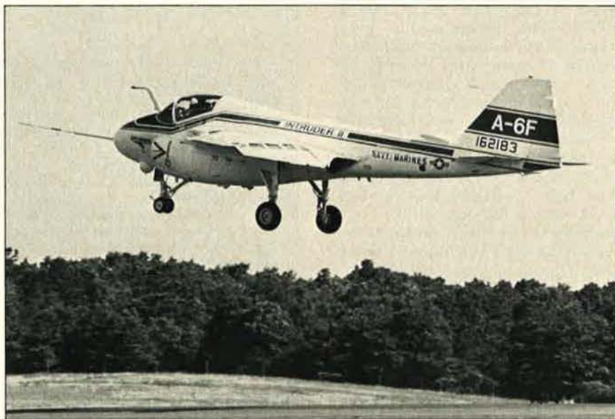
The first Grumman A-6F Intruder II flew for the first time on August 26 from the company's facility in Calverton, N. Y. The A-6F is a significantly upgraded version of the veteran attack aircraft and features a sharper, more powerful radar, an air-to-air capability, five new multifunction cockpit displays, and General Electric F404-GE-400D engines.
