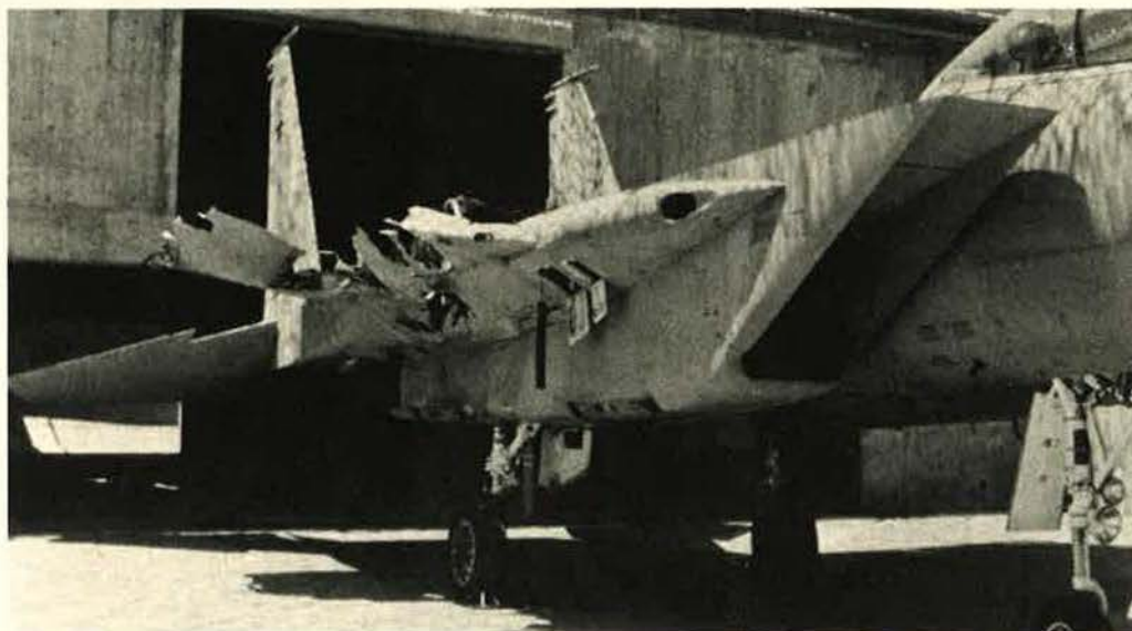
FIGURE IV. The nonpareil example of an aircraft taking a structural beating and remaining airworthy is this F-15, which recovered safely after losing an entire wing in a midair collision. USAF's new fighters owe their capacity for such survivability to stronger materials, ingenuity of design, and "smart" flight controls that compensate for structural damage by getting the most out of the aerodynamic capability that remains.
