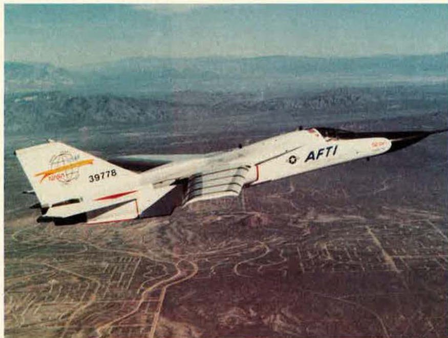
With the Mission Adaptive Wing in the fully cambered position, as in this photo, both the leading and trailing edges move approximately twenty degrees downward. The upper surfaces of both edges are made of high-strength, lightweight composite material that bends when actuated by internal hydraulic systems.
