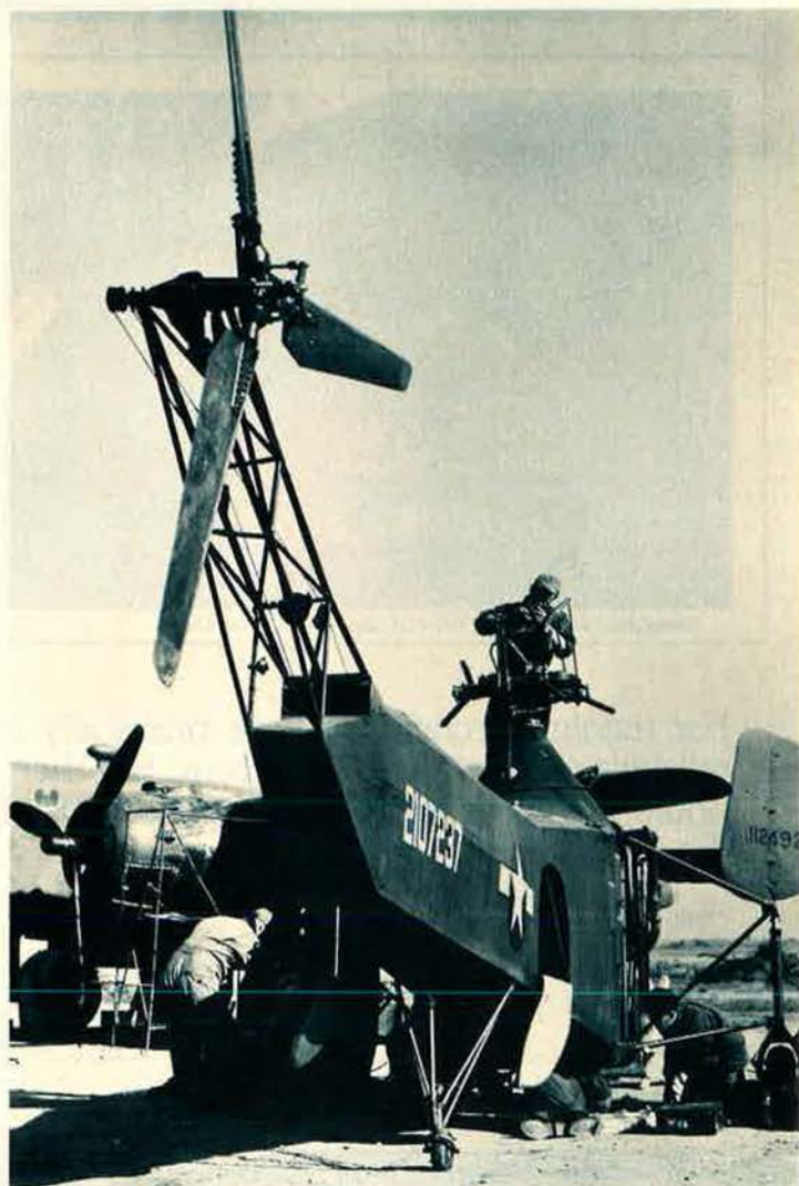
Just like a big Revell model! Here Sgt. Don Nigro (on top, working on the main rotor assembly) and his colleague at Myitkyina, Burma, reassemble the first YR-4 helicopter shipped to the Burma-India theater for rescue work during World War II. The Sikorsky was flown from Wright Field in a C-54.
