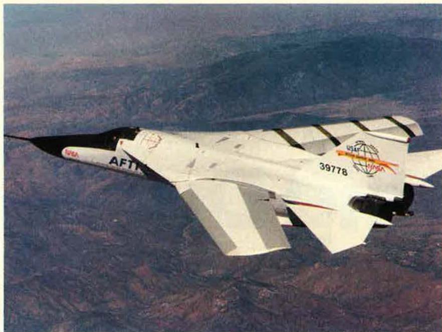
With the Mission Adaptive Wing, the "catch" is that airplane designers must be prepared to develop new airfoil shapes for each of the flight conditions that future aircraft will encounter. Result: a more complex design process, with a need for structures, flight controls, and other elements to work closely together.
