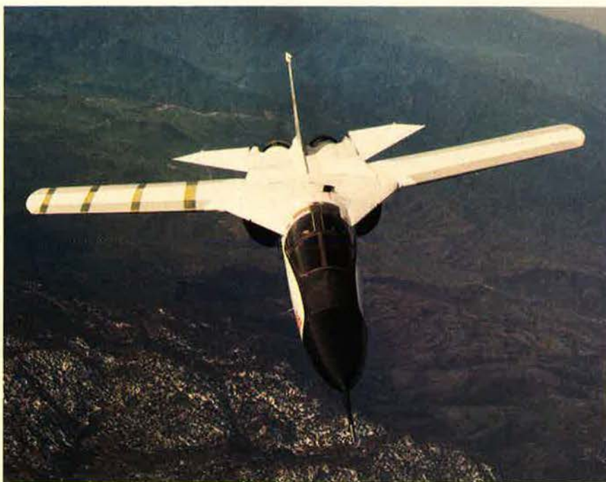
Advanced computers for controlling the Mission Adaptive Wing are contained in the F-111's nose. The upper surface of the wing is completely smooth, with the mechanism for controlling it buried inside. The wing's leading edge is a single span surface; the trailing edge consists of three panels capable of independent motion.
