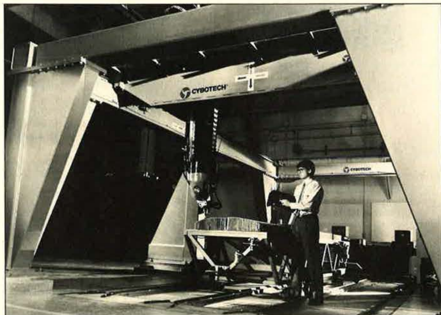
This Lockheed engineer is monitoring the performance of a Cybotec five-axis gantry robot as it cuts honeycomb-core composite material at Lockheed Aeronautical Systems Co.'s Composite Development Center, which opened last April. Composites will be invaluable in helping manufacturers attain the weight limits that USAF seeks for such future mainstays as the Advanced Tactical Fighter.
