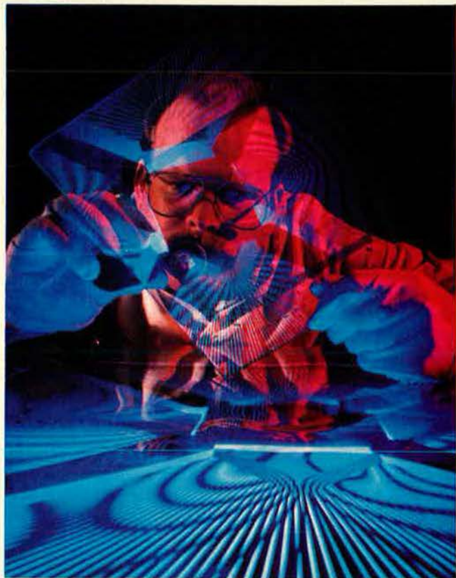
Microelectronics is one of the cornerstones many new technologies are built on. Here, Tim Hopkins, a General Dynamics technician, checks circuit paths printed on a glass plate. The plate, used to test missile electronics, must be accurate to twenty millionths of an inch.
