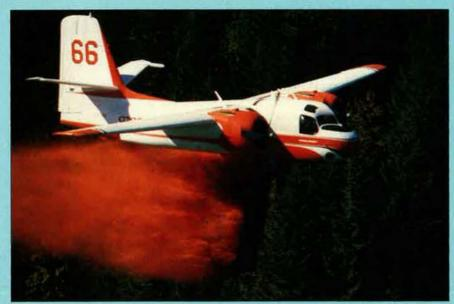
Conair Firecat fire control conversion of a Grumman S-2A/S2F-1 Tracker anti-submarine aircraft
