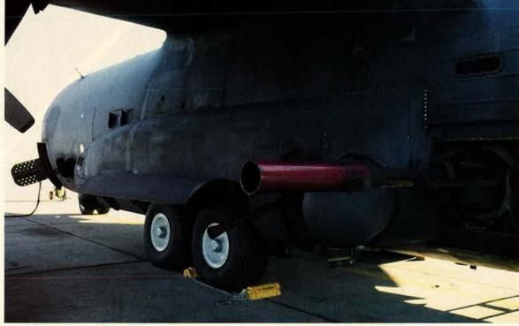
The business end of the AC-130H's 105mm cannon. The standard that the load crews strive for is to have one of the gun's fifty-five-pound shells striking the target, one on the way, and one in the breech at any given time. When this gun is fired, the entire AC-130 fishtails to the right from the recoil.
