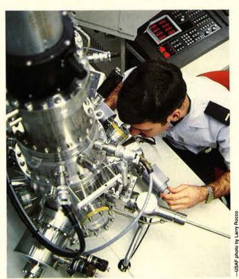
The state of the integrated circuit art is continually being refined, but because of their miniscule size and labyrinthine complexity, instruments such as this Auger spectrometer must be used to analyze the chips.
