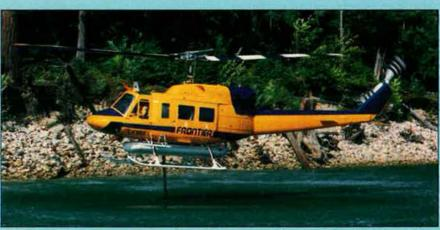
Conair equipped Bell 212 firefighting helitanker hovering to pick up water from a lake
