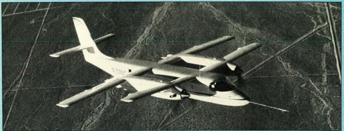
The 'trimaran' layout of the SCI Advanced Technology Tactical Transport proof-of-concept prototype reflects its Rutan parentage
