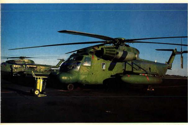
The 1st SOW's specialized rotary-wing assets are the Sikorsky MH-53H Pave Low II helicopters. The Pave Low Ils tend to operate closer to the ground more often than their fixed-wing brethren, so the helicopters are beefed up with 1,000 pounds of armor plate and are able to hover automatically. The helicopter in the background is a transient CH-53B.
